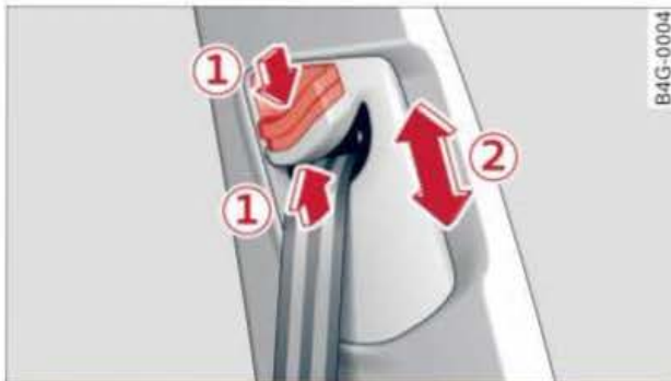
Fig. 185 Belt height adjustment for the front seats: guide fitting
