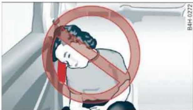
Fig. 168 Illustration of a dangerous sitting position near the opening for the side airbag
