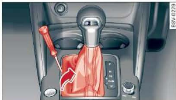
Fig. 124 Selector lever: Removing the cover
