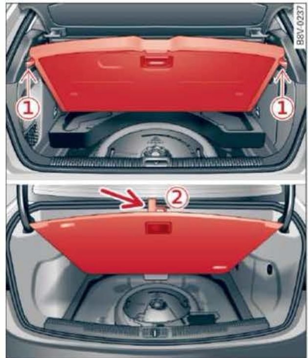
Fig. 247 Luggage compartment: Floor panel folded up (A3 and A3 Sportback top, A3 Saloon bottom)
