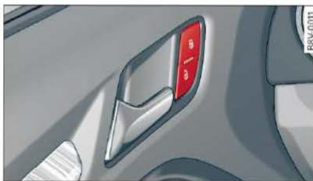
Fig. 39 Driver's door: Central locking switch
