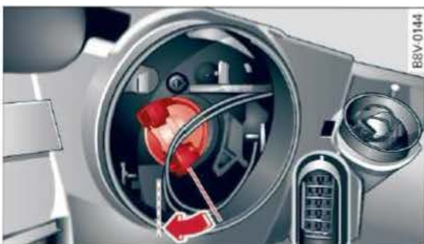
Fig. 274 Bulb housing: Fitting the bulb
