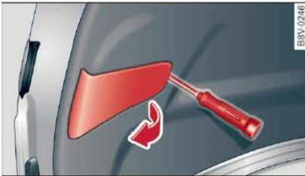
Fig. 313 Open boot lid (A3 Saloon): Removing cover from boot lid interior trim
