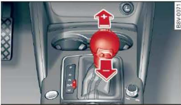
Fig. 120 Centre console: Manual gear selection using selector lever
