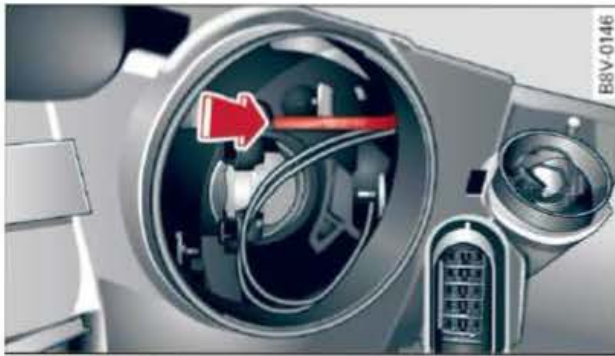
Fig. 277 Bulb housing: Inserting the bulb holder
