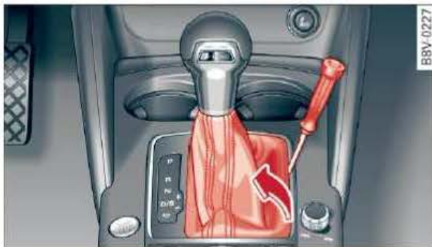
Fig. 122 Selector lever: Removing the cover
