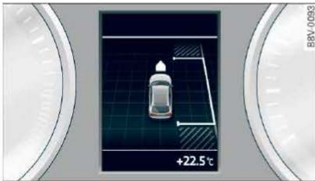
Fig. 163 Instrument cluster: Prompt to keep driving forwards (a parking space has been detected)
