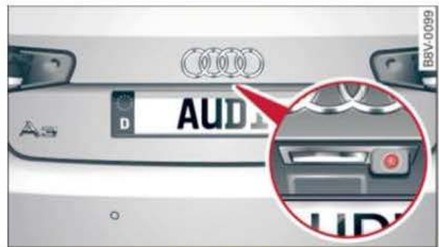
Fig. 153 Boot lid: Location of reversing camera (example)
