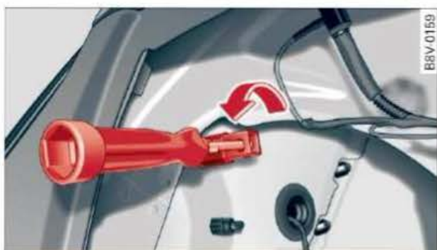
Fig. 291 Releasing rear light from luggage compartment (example on left side)
