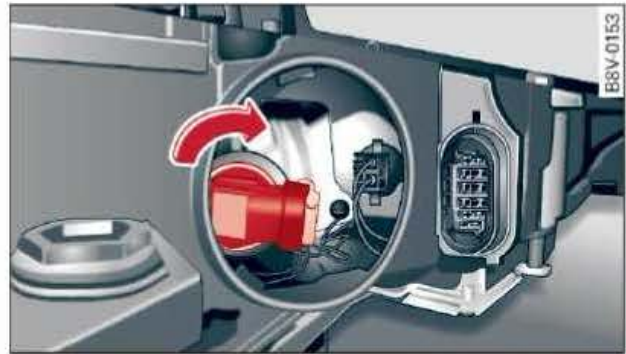
Fig. 286 Bulb housing: Tightening the bulb holder
