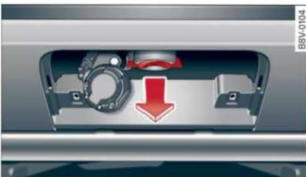
Fig. 204 Area below rear bumper: Pulling out plug
