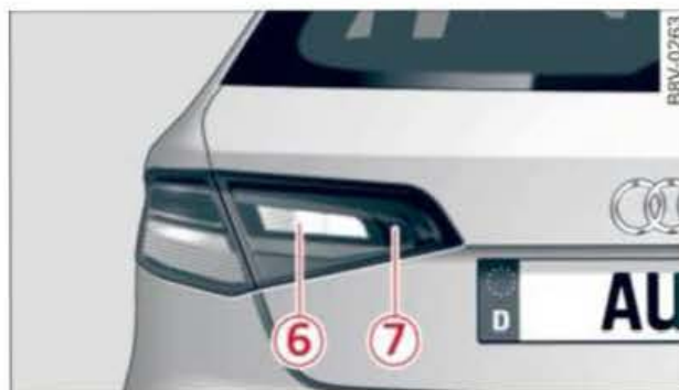
Fig. 265 Xenon/LED system, rear light: Bulbs in side panel and boot lid
