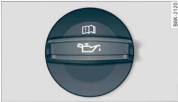
Fig. 222 Engine compartment: Engine oil filler cap
