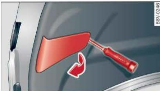
Fig. 316 Open boot lid: Removing cover from boot lid interior trim
