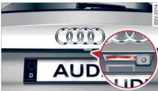
Fig. 42 Boot lid: Opening (release catch)
