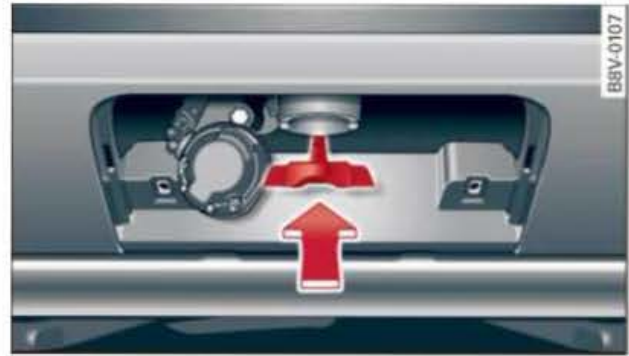
Fig. 211 Area below rear bumper: Fitting the plug
