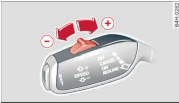
Fig. 134 Control lever: Setting the distance
