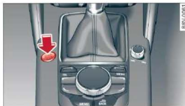
Fig. 104 Centre console: START ENGINE STOP button (vehicles with convenience key)
