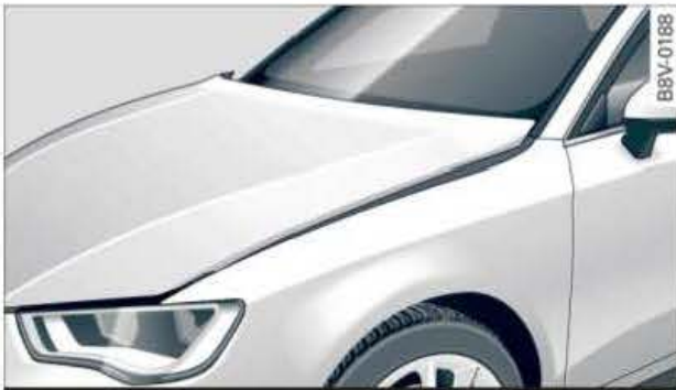
Fig. 174 Bonnet: Pedestrian protection system triggered
