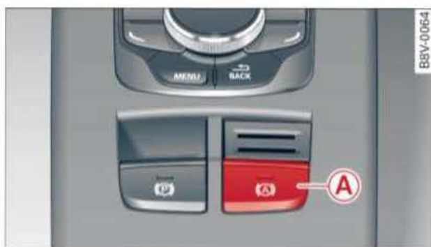
Fig. 107 Section of centre console: Button for hold assist
