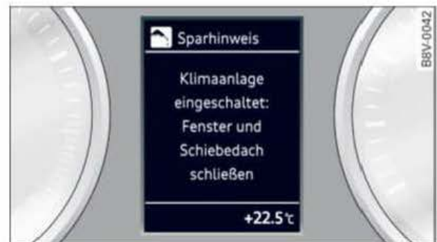
Fig. 22 Instrument cluster: Economy tip (Air conditioner switched on: close windows and sun roof)
