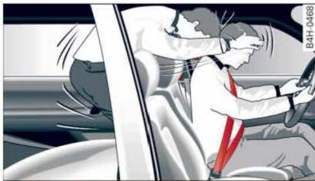
Fig. 180 A rear passenger not wearing a seat belt can be thrown forwards
