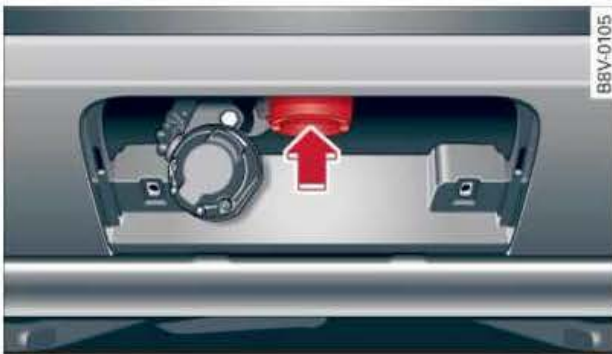
Fig. 207 Removable towing bracket: Inserting the ball joint
