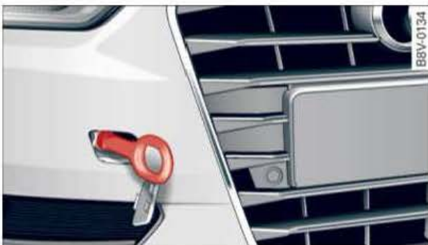
Fig. 252 Front bumper (right side): Towline anchorage screwed in
