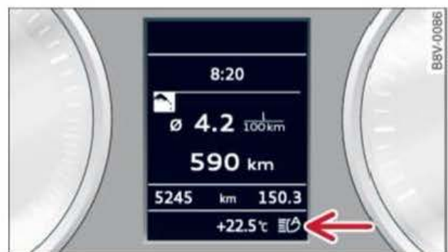
Fig. 53 Instrument cluster: Indicator lamp for main beam assist
