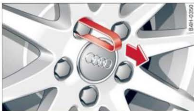
Fig. 240 Wheel: Wheel bolts with caps
