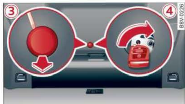
Fig. 45 (A3/A3 Saloon) Detail of inside of boot lid: Access to manual release
