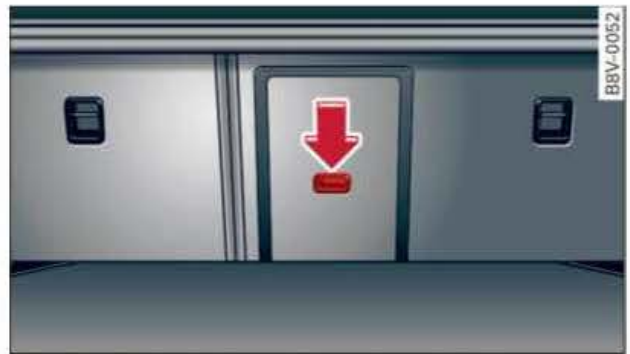
Fig. 92 Backrest: Cover of load-through hatch
