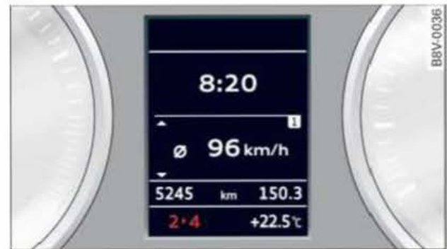
Fig. 7 Instrument cluster: Gear-change indicator (for manual gearbox)
