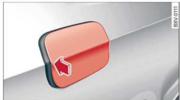
Fig. 115 Vehicle as seen from the rear right: Opening the fuel tank flap
