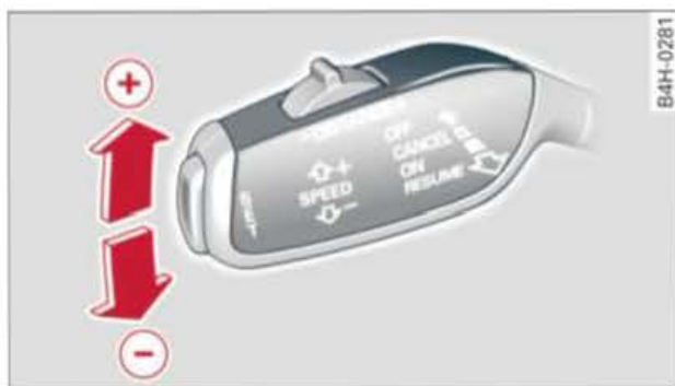
Fig. 132 Control lever: Setting a new speed
