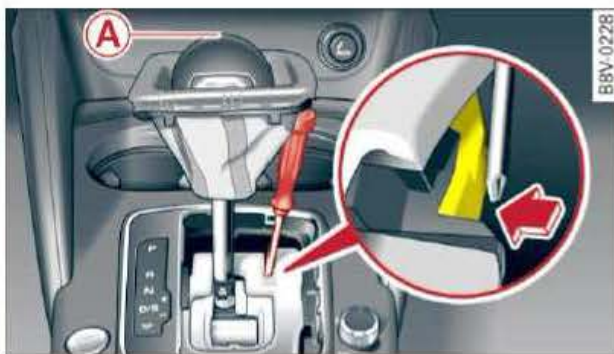
Fig. 123 Manually releasing the selector lever from position P
