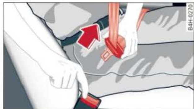
Fig. 186 The latch plate of the belt springs out of the buckle
