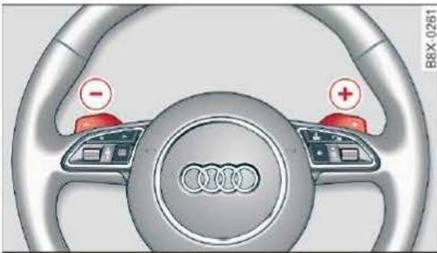
Fig. 121 Steering wheel: Manual gear selection with paddle levers*
