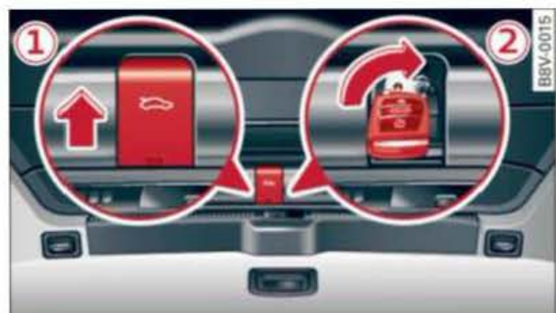
Fig. 44 (A3/A3 Sportback) Detail of inside of boot lid: Access to manual release
