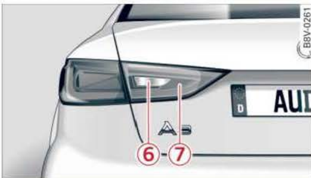
Fig. 267 Xenon/LED system, rear light: Bulbs in side panel and boot lid
