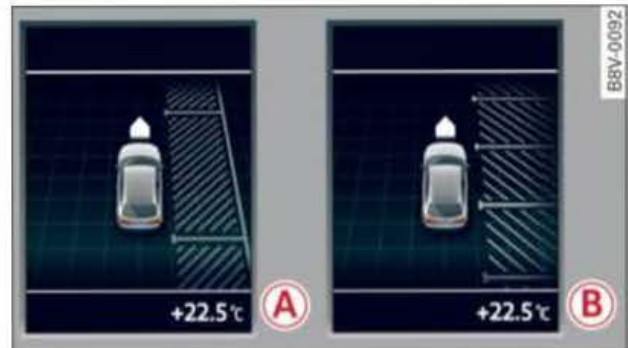
Fig. 162 Instrument cluster: Looking for a parking space. A parallel to the roadside, B perpendicular to the roadside
