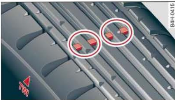
Fig. 228 Tyre tread: Tread wear indicators
