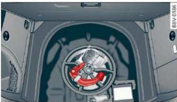
Fig. 202 Luggage compartment: Ball joint for towing bracket (stowage example)
