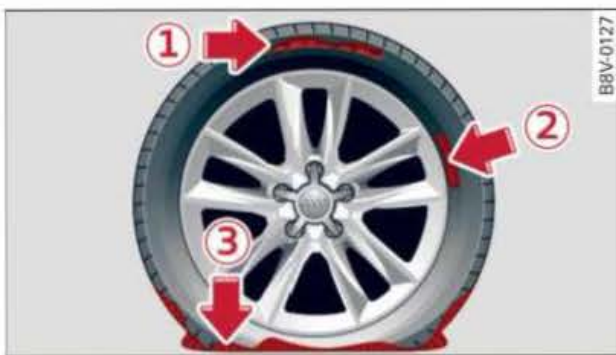
Fig. 237 Tyres: Irreparable tyre damage
