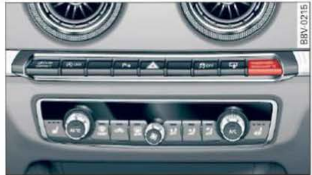
Fig. 199 Centre console: Warning lamp lights up when passenger's airbag is deactivated
