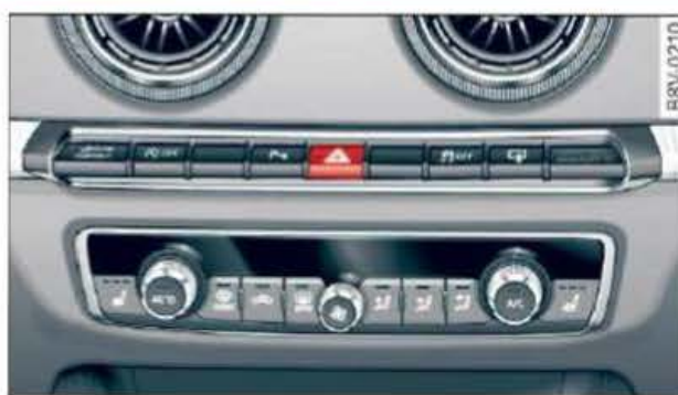
Fig. 55 Dashboard: Switch for hazard warning lights
