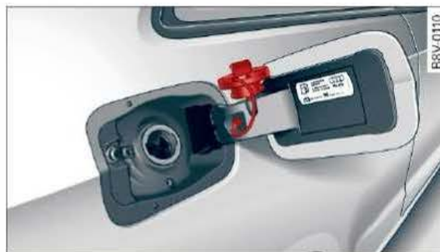
Fig. 216 Fuel tank flap with tank cap attached
