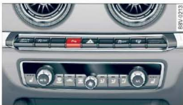
Fig. 148 Centre console: Switch for parking aid
