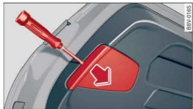
Fig. 299 Open boot lid: Removing cover from boot lid interior trim
