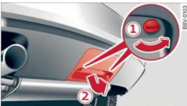
Fig. 203 Area below rear bumper: Removing bumper cover (example)
