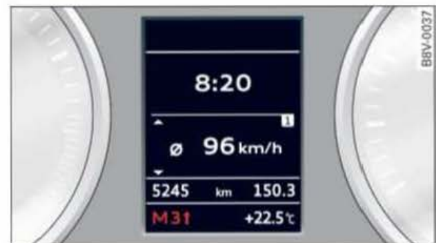
Fig. 8 Instrument cluster: Gear-change indicator in tiptronic mode (for automatic gearbox)
