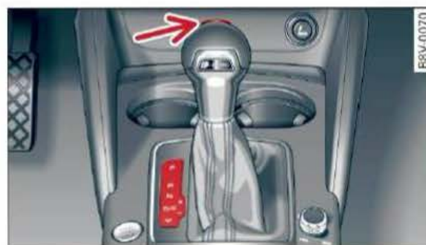
Fig. 119 Detail of the centre console: Selector lever with interlock button
