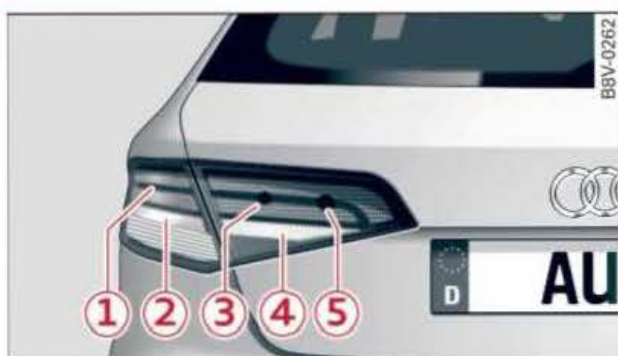
Fig. 264 Halogen system, rear light: Bulbs in side panel and boot lid
