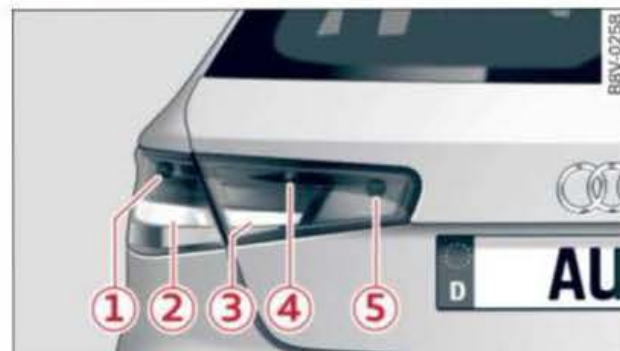
Fig. 262 Halogen system, rear light: Bulbs in side panel and boot lid
