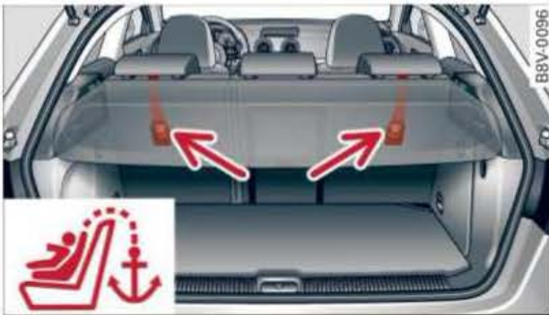
Fig. 171 Rear seat bench (A3/A3 Sportback): Top tether anchorages
