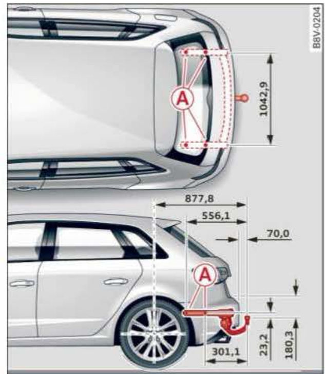
Fig. 213 A3 Sportback: Positions of securing points (viewed from above and from side)
