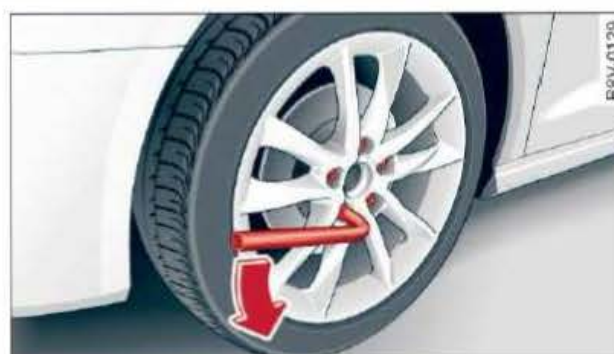
Fig. 242 Wheel: Loosening the wheel bolts
