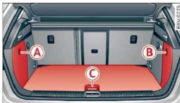
Fig. 235 Luggage compartment (example): Stowing the tools, tyre repair kit and jack*
