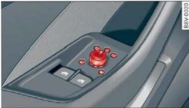
Fig. 59 Driver's door: Adjuster knob for exterior mirrors (example)
