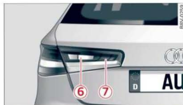
Fig. 263 Xenon/LED system, rear light: Bulbs in side panel and boot lid
