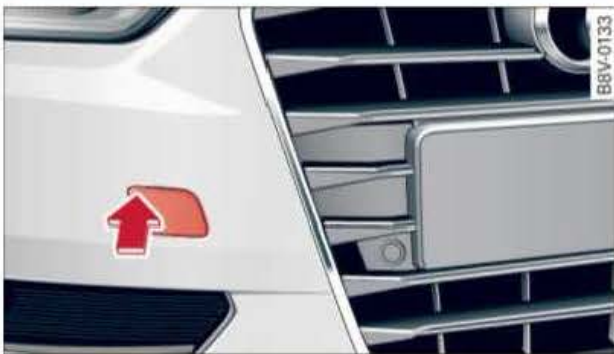
Fig. 251 Front bumper (right side): Removing cover
