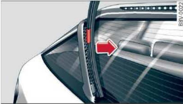
Fig. 65 Rear window wiper: Removing the wiper blade
