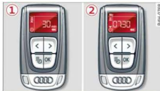
Fig. 100 Remote control for auxiliary heating: ① switching on immediately ② setting the timer
