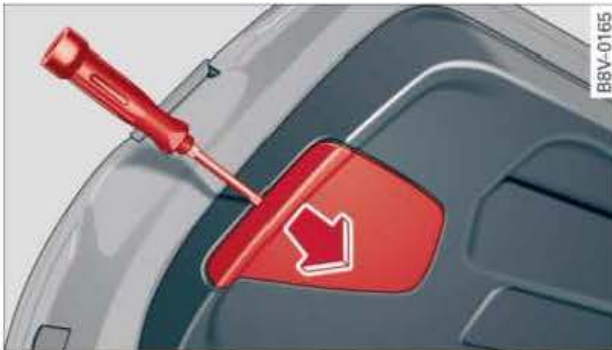
Fig. 301 Open boot lid: Removing cover from boot lid interior trim
