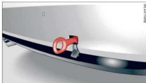
Fig. 254 Right side of the rear bumper: Towline anchorage screwed in
