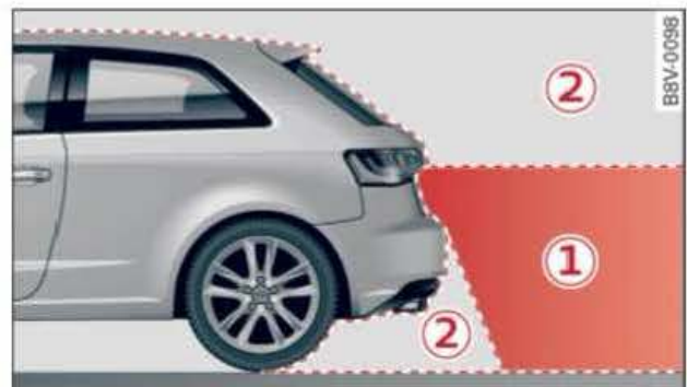
Fig. 152 ①: Area covered by the reversing camera; ②: area NOT covered by the reversing camera (example)
