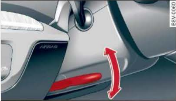
Fig. 102 Steering column: Lever for steering column adjustment
