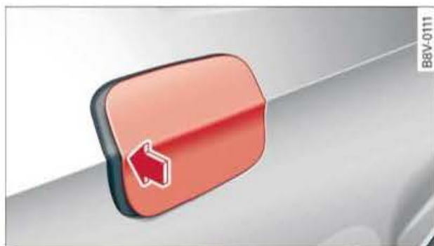
Fig. 215 Vehicle as seen from the rear right: Opening the fuel tank flap
