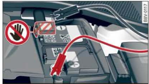
Fig. 225 Engine compartment: Terminals for jump leads and battery charger
