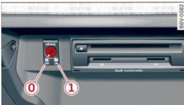
Fig. 198 Glove box: Key-operated switch for deactivating front passenger's airbag
