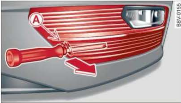
Fig. 287 Detail from front of vehicle, left side: Removing trim
