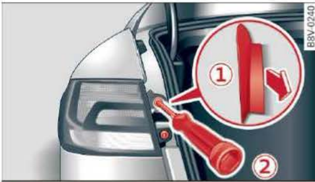
Fig. 307 Releasing rear light (example on left side)
