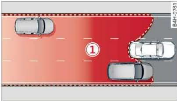
Fig. 141 Area covered by the radar sensors
