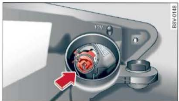
Fig. 280 Bulb housing: Inserting the bulb holder
