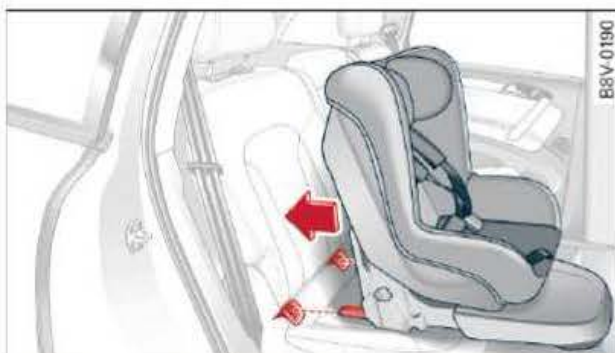
Fig. 170 Rear seat: Securing child seat with ISOFIX (example)
