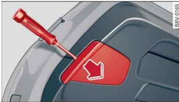
Fig. 304 Open boot lid: Removing cover from boot lid interior trim
