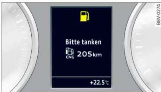
Fig. 114 Display: Combined fuel warning for petrol and natural gas
