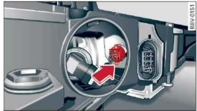
Fig. 283 Bulb housing: Tightening the bulb holder
