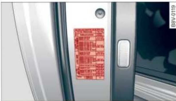
Fig. 227 Open driver's door (LHD vehicle): Sticker listing tyre pressures
