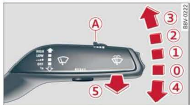
Fig. 62 Windscreen wiper lever: Operating the windscreen wipers (example shows vehicle without rear window wiper)
