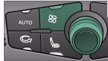
Fig. 109 Blower button and rotary control
