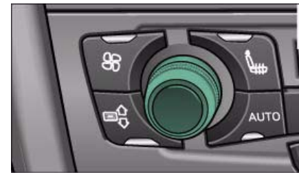
Fig. 117 Rotary control for temperature selection
