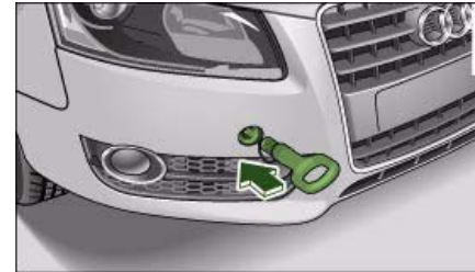
Fig. 251 Front bumper: Fitting the towing eye
