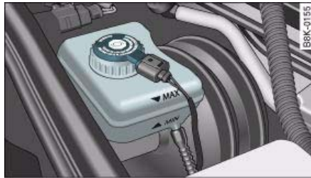
Fig. 228 Engine compartment: Markings on brake fluid reservoir
