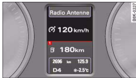
Fig. 142 Symbol: Cruise control temporarily switched off
