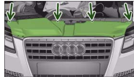
Fig. 258 Trim panel: Attachment points are marked by arrows
