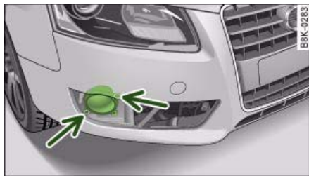
Fig. 270 Screws securing fog light
