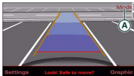
Fig. 161 MMI display: Aligning the vehicle with the help of the blue area markings
