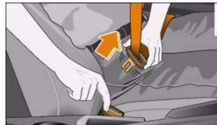
Fig. 186 The latch plate of the belt springs out of the buckle
