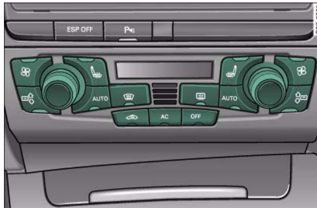
Fig. 116 Air conditioner controls
