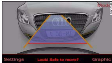
Fig. 169 MMI display: Red line makes contact with bumper
