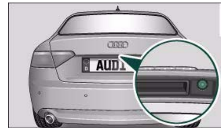
Fig. 154 Boot lid: Location of reversing camera
