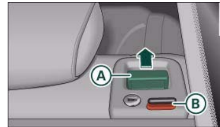
Fig. 90 Release handle on backrest
