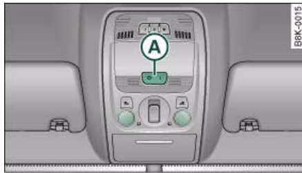
Fig. 58 Headliner: Front interior lights
