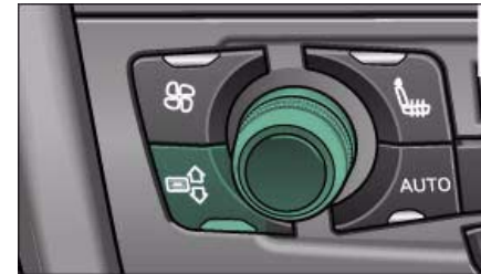
Fig. 121 Air distribution button and rotary control
