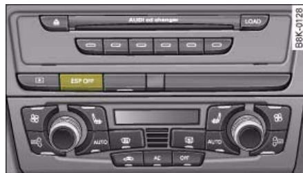
Fig. 204 Centre console with ESP switch
