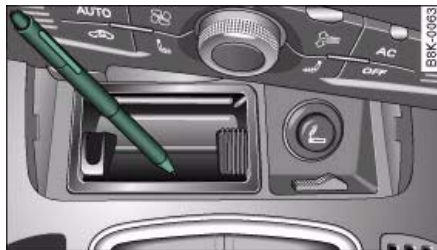
Fig. 151 Manual release of selector lever
