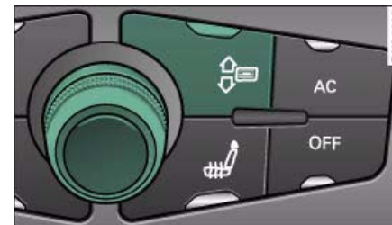
Fig. 111 Air distribution button and rotary control
