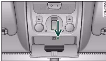
Fig. 48 Detail of headliner: Unscrewing the light housing
