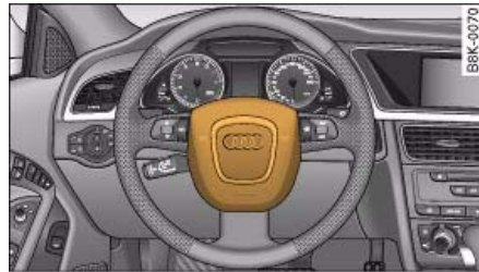
Fig. 187 Driver's airbag in steering wheel
