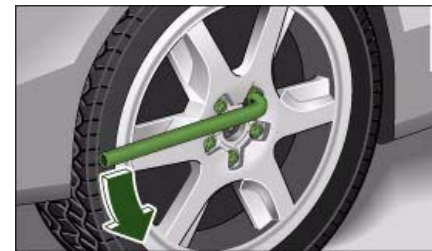
Fig. 242 Changing a wheel: Loosening wheel bolts
