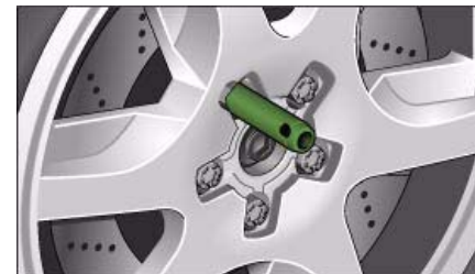
Fig. 246 Changing a wheel: Mounting pin in wheel bolt hole nearest to the top
