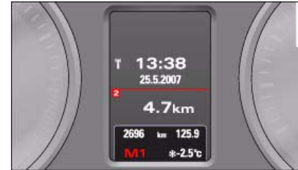
Fig. 148 Display: Manual gear selection (tiptronic mode)
