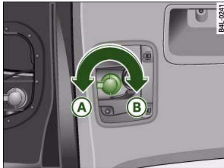
Fig. 257 Diagram: Bulb holder with a bayonet fastener
