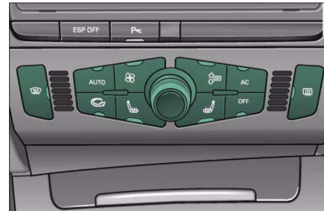
Fig. 106 Controls for deluxe automatic air conditioner
