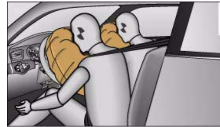
Fig. 189 Front airbags in inflated condition
