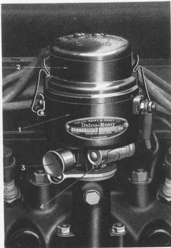
Fig. 39.—CONTACT BREAKER AND DISTRIBUTOR. 1. Contact breaker. 3. Lubricator. 2. Distributor. 4. Condenser.
