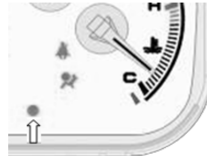
Security system indicator
