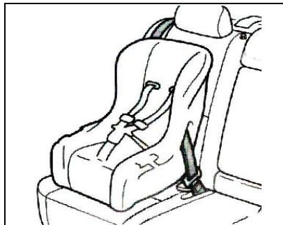
Seat belt equipped with child protection device locking mechanism
