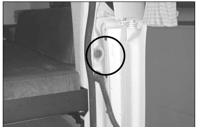
Picture G-P8 : The gravity fill for the interior fresh water tank, (located on passenger side rear door post).
