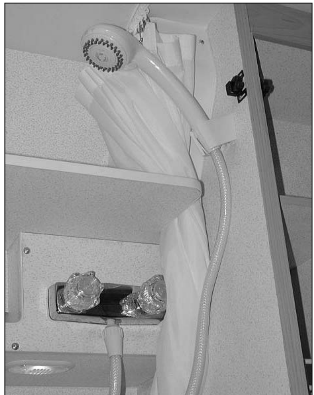
Picture B-P22: Hand held shower head in its shower position.
