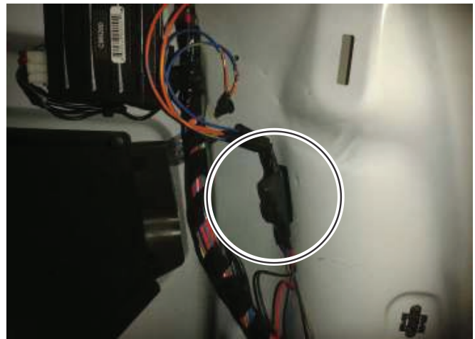
Driver's Power Seat Connector (Passenger's Same)
