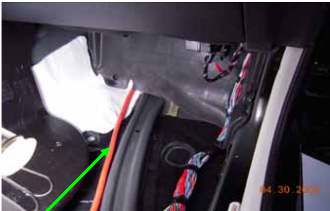
Starter Cable left of harness with 120 amp Police PDC
