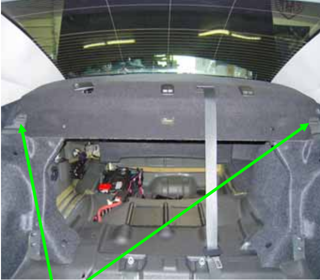
Rectangular slots (1) that spring clips (2) go into.
