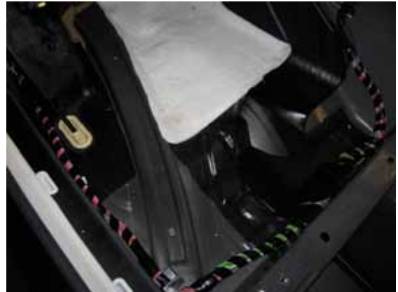
BODY HARNESS – Drivers floor pan left & driveshaft tunnel left
