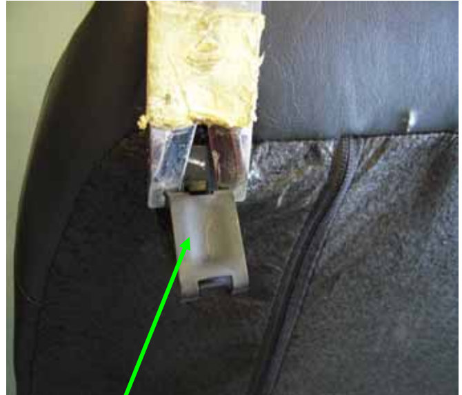
Spring clips (2) that snap into rectangular slots (1). There is one on each side of the seat back.
