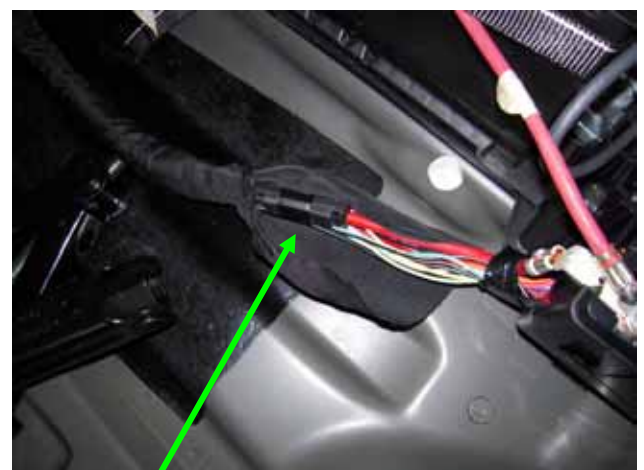
125 amp Police PDC Fuse Fuse is in the trunk next to the battery.
