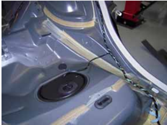
BODY HARNESS – Left rear door and wheel well area (Black Cover is Fuel Pump Access)
