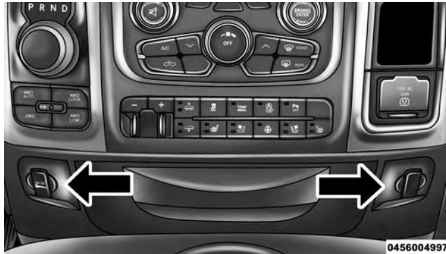
Power Outlets — Center Stack
