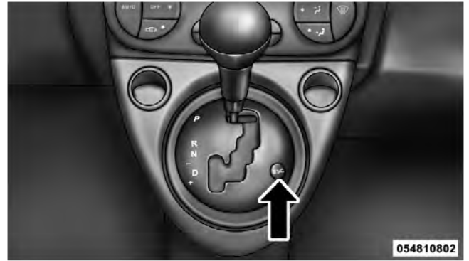
ESC Off Switch (Automatic Transmission)
