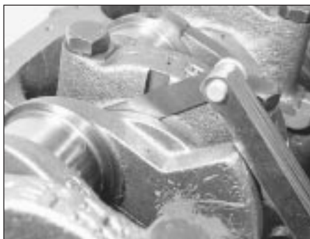
22.6 Checking crankshaft endfloat
