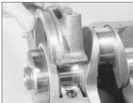
22.7 Removing the rear main bearing cap
