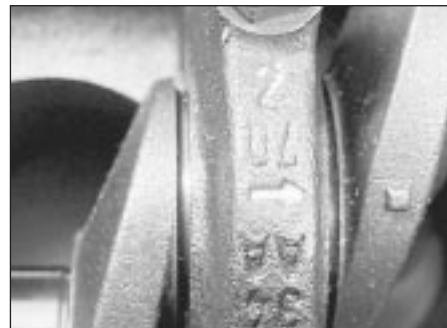
22.5 Main bearing cap identification marks The arrow points to the front of the engine
