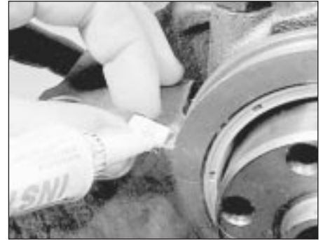
36.19 Fitting a sealing wedge to the rear main bearing cap
