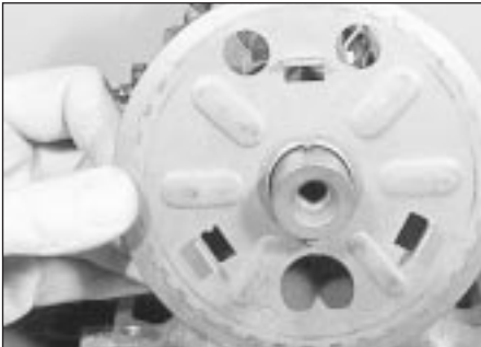
11.3 Removing the camshaft sprocket backplate
