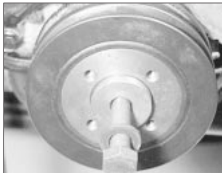
45.5b Crankshaft pulley bolt and washer
