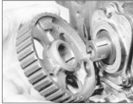
13.11 Removing the auxiliary shaft sprocket
