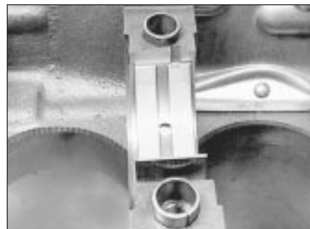
22.9 Removing the centre main bearing shell
