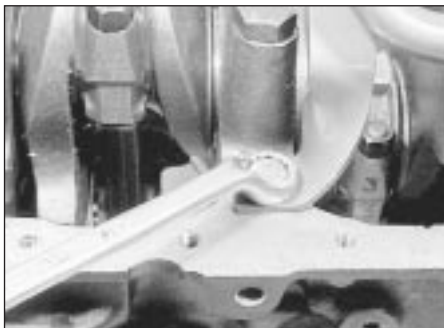
19.2 Unbolting the oil pump pick-up strainer from the block
