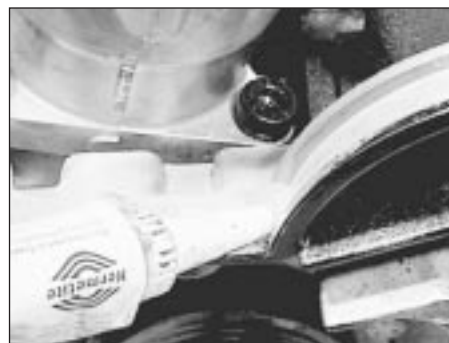
39.1a Applying sealing compound to a rubber strip location
