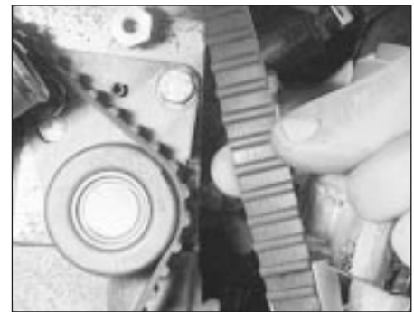
45.12 Twisting the timing belt to assess its tension
