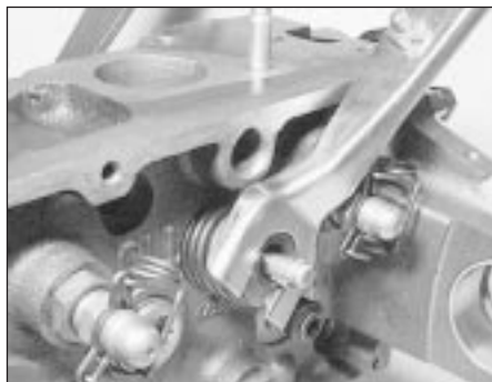
12.2a Compressing a valve spring
