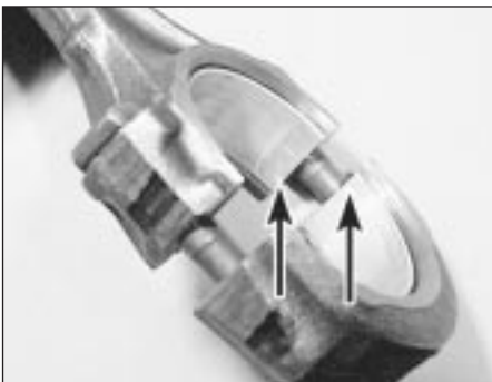
37.2 Big-end bearing shell lugs (arrowed) are adjacent
