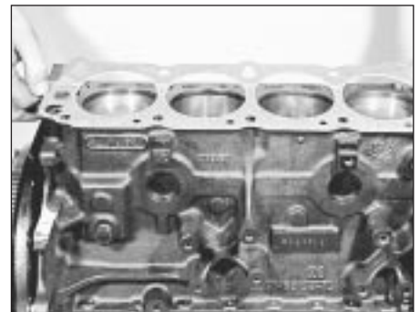
44.3 Fitting a new cylinder head gasket
