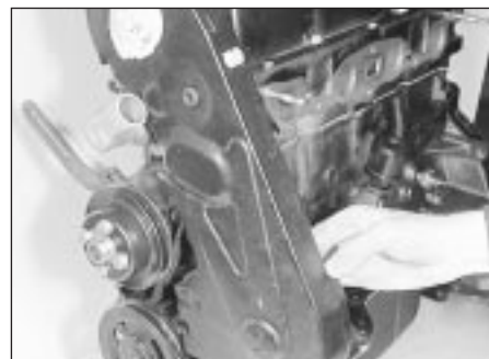
10.2 Removing the timing cover
