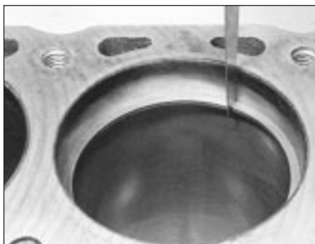
29.4a Checking a piston ring gap at the top of the cylinder
