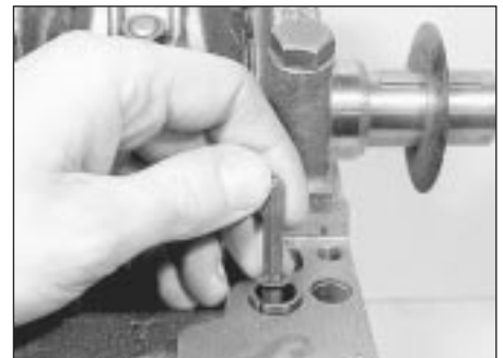
19.4 Removing the oil pump driveshaft
