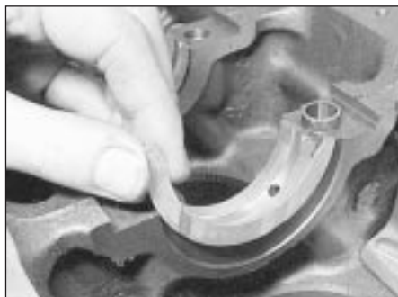
22.8b Removing a thrustwasher from the centre main bearing
