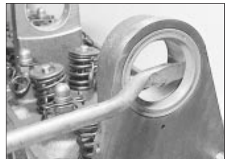
11.9 Prise out the camshaft bearing oil seal
