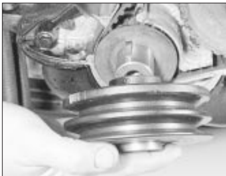
45.5a Refitting the crankshaft pulley
