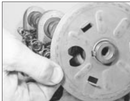
43.7 Fitting the camshaft sprocket backplate
