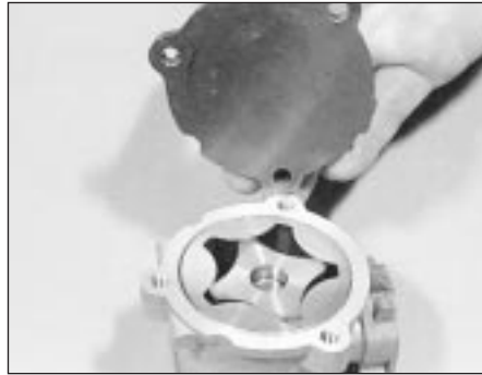
26.1 Removing the oil pump cover
