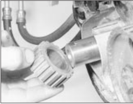
13.9 Removing the crankshaft sprocket
