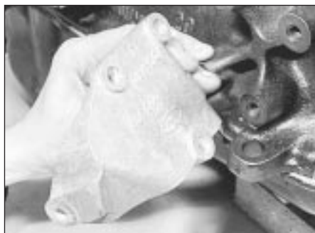
9.1c Removing the alternator bracket
