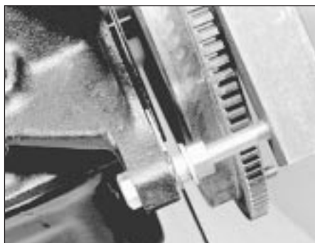
40.4a Method of holding the flywheel when tightening the bolts
