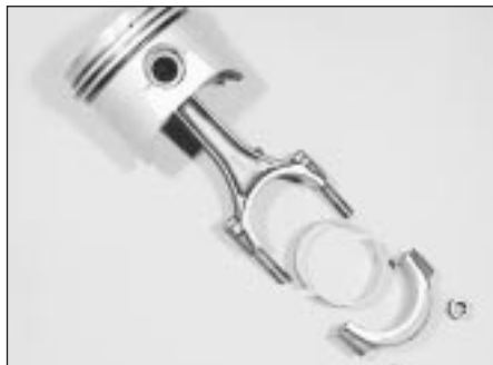
21.4 Piston, connecting rod, cap and bearing shells
