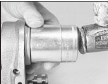
43.1 Fitting the camshaft front bearing oil seal
