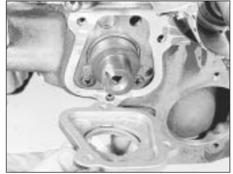
14.4 Removing the auxiliary shaft front cover
