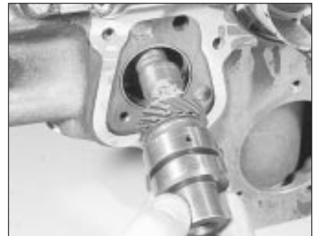
14.5b Removing the auxiliary shaft
