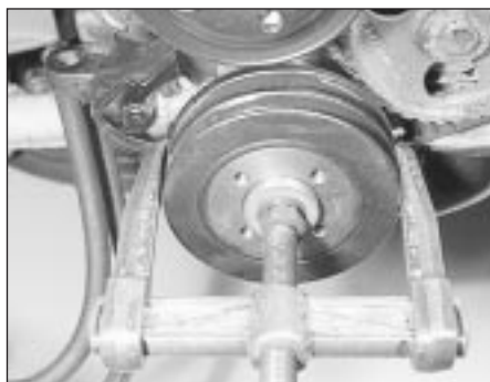
13.7 Using a puller to remove the crankshaft pulley
