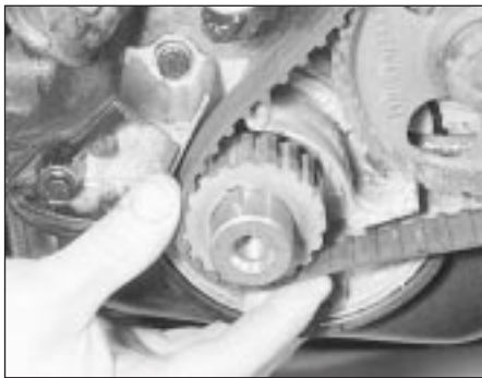
45.4 Fitting the timing belt over the crankshaft sprocket
