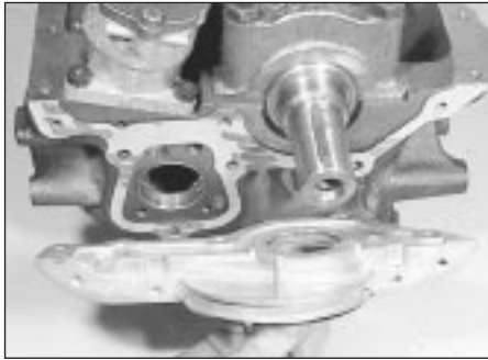
17.3a Removing the crankshaft front oil seal housing
