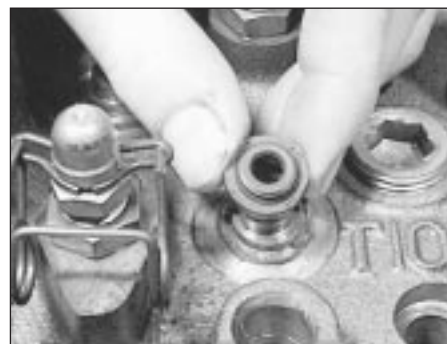
12.4 Removing a valve stem oil seal
