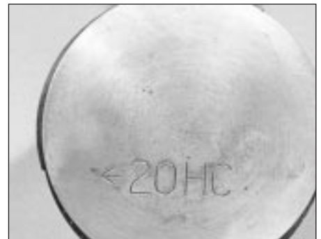
37.4b Piston crown markings Arrow points to front of engine
