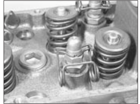
42.3 Cam follower ball-pins and spring clips fitted
