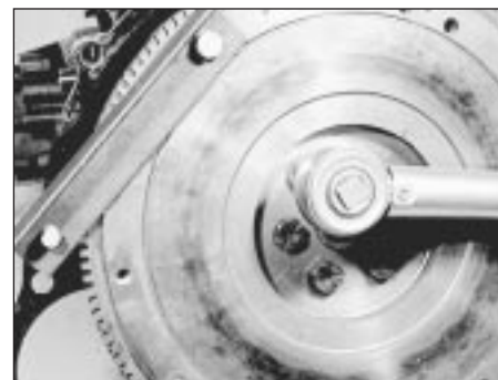
40.4b Tightening a flywheel bolt
