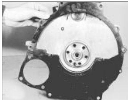
15.4 Removing the engine adaptor plate (backplate)
