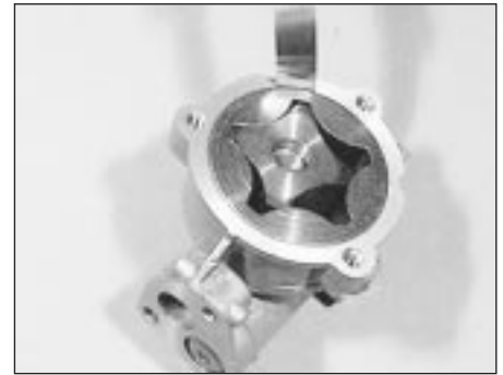
26.2a Checking the outer rotor-to-housing clearance
