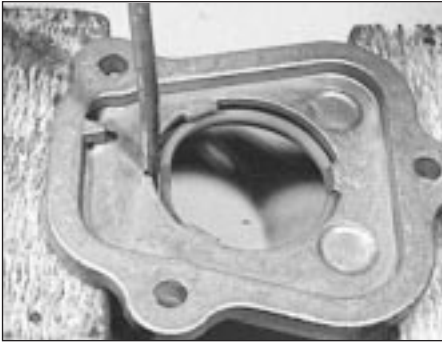
41.3a Driving out the auxiliary shaft cover oil seal
