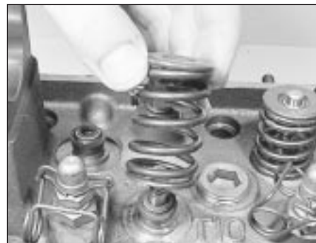
12.2b Removing a valve spring and cap
