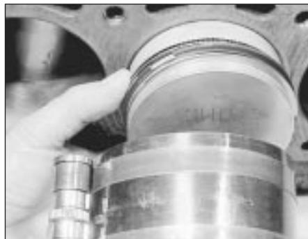
37.4a Fitting a piston ring compressor
