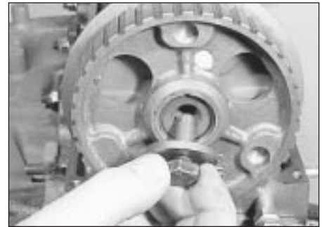
11.2 Removing the camshaft sprocket bolt and sprocket
