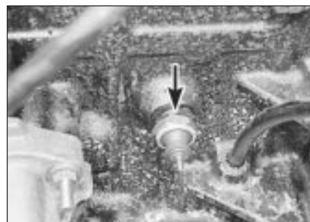
9.1a Engine oil pressure switch (arrowed)
