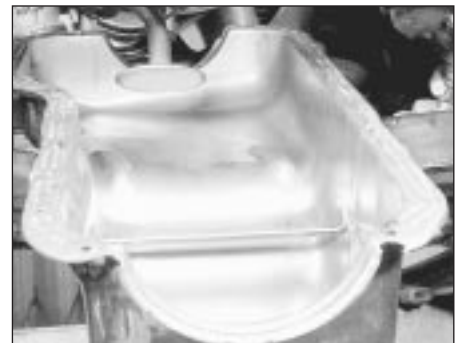
16.12 Removing the sump
