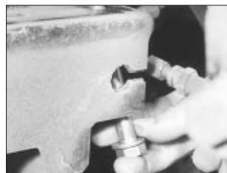
5.38 Removing a suspension crossmember securing bolt
