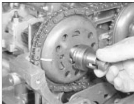
18.5 Removing the inlet camshaft sprocket bolt and the distributor rotor shaft
