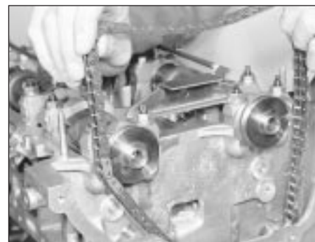
15.13 Withdrawing the timing chain through the top of the timing case
