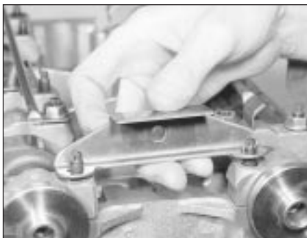
18.30c Fitting the timing chain guide plate
