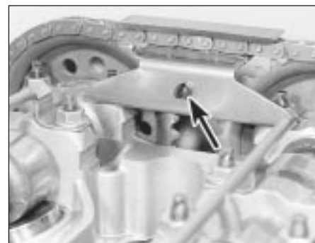
18.7 Upper timing chain guide securing lugs (arrowed)
