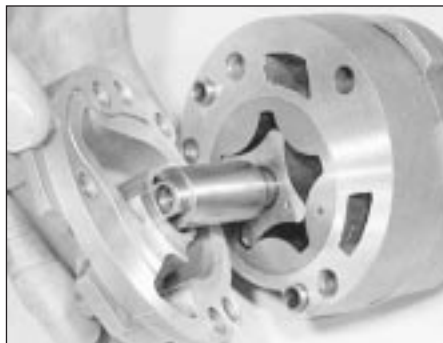
27.3 Removing the oil pump cover
