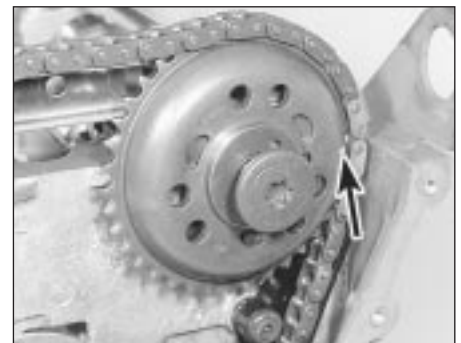
18.38 Spacer and sprocket securing bolt fitted to end of camshaft, with camshaft in TDC position (timing marks arrowed)
