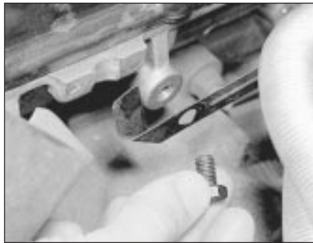
5.5 Removing the hose support bracket bolt from the cylinder head
