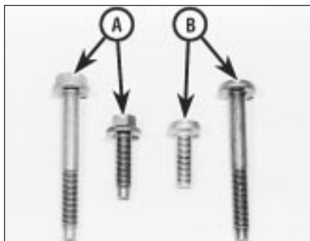
18.0 Use new M8 (auxiliary) cylinder head bolts with hexagonal heads (A), not the earlier Torx type bolts (B)
