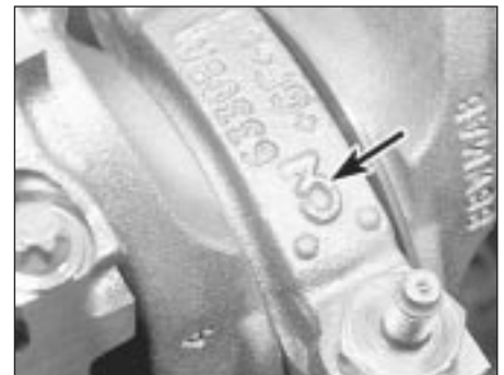
30.5 Main bearing cap identification mark (arrowed)
