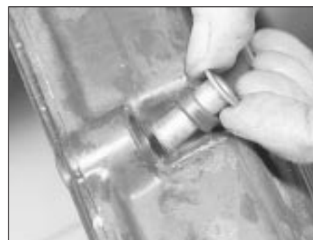
18.54 Fitting a camshaft cover reinforcing sleeve and sealing ring
