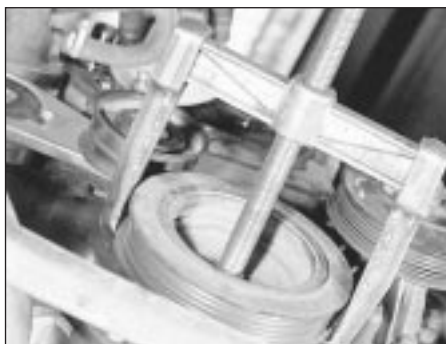
15.5a Using a puller to remove the crankshaft pulley (viewed from underneath vehicle)
