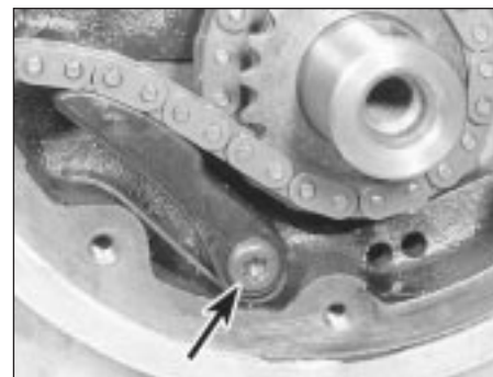
15.9 Oil pump chain tensioner securing screw (arrowed)
