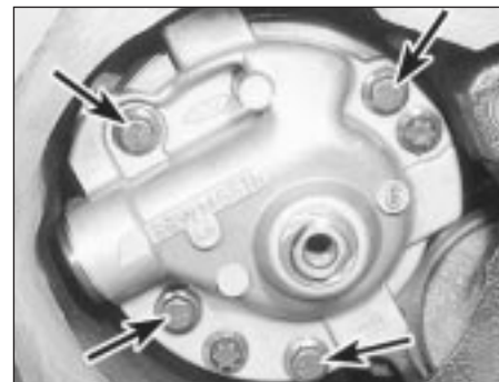
26.3 Oil pump securing bolts (arrowed)
