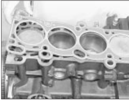
18.22 Fitting a new cylinder head gasket
