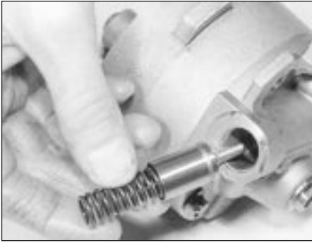
27.5b . . . and withdraw the spring and plunger
