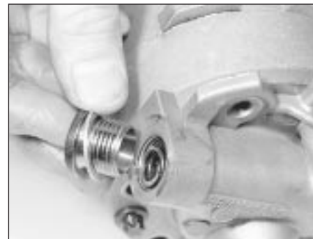
27.5a Unscrew the pressure relief valve plug and washer . . .
