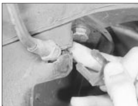
5.37 Removing a brake line securing clip from the suspension crossmember
