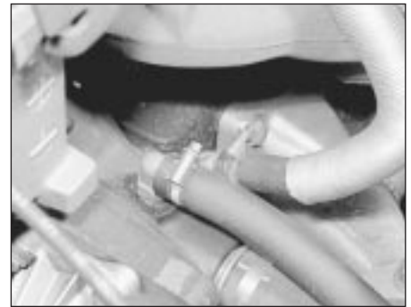
5.8 Water pump coolant hoses (viewed from above)
