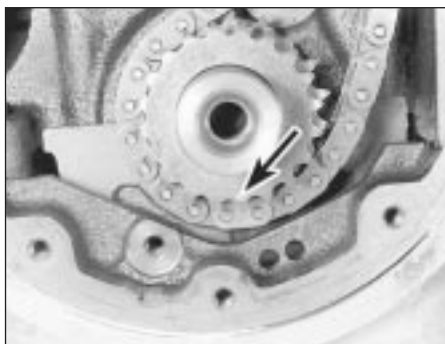
15.19 Coppered link in timing chain aligned with crankshaft sprocket timing mark (arrowed)
