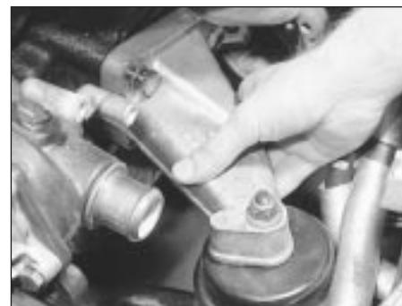
5.36 Remove the engine mounting brackets to improve clearance
