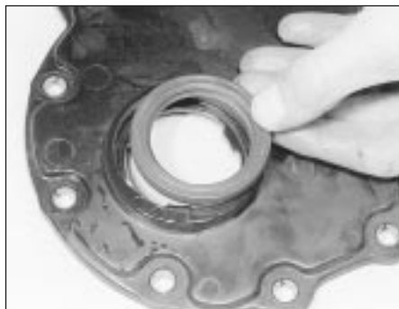
15.31 Fitting a new lower timing chain cover oil seal
