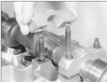
18.14a Lifting off a camshaft bearing cap
