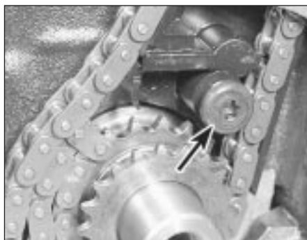
15.11b Lower timing chain guide lower securing bolt (arrowed)
