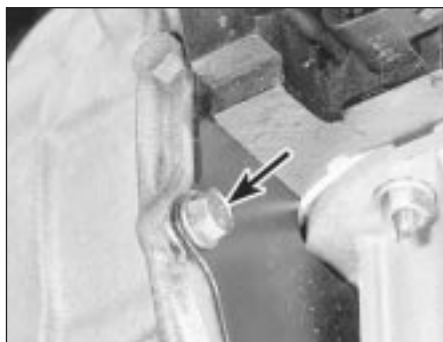
5.33 Engine adaptor plate bolt (arrowed)
