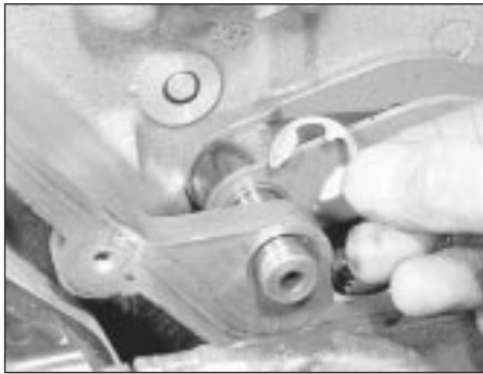
18.9 Removing the chain tensioner arm pivot pin circlip
