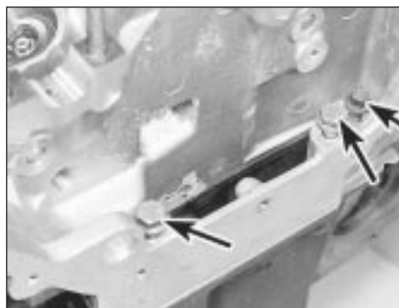
18.16 M8 cylinder head bolts (arrowed) located at front of cylinder head
