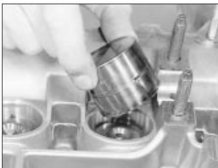
18.15 Withdrawing a cam follower
