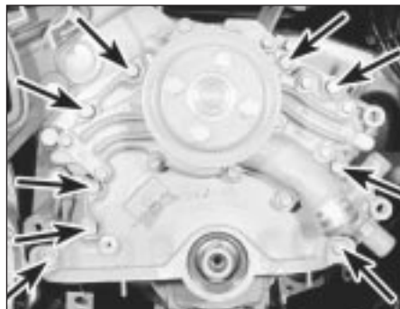
36.27 Timing cover retaining bolts (arrowed)
