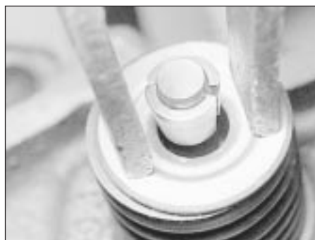
23.2a Compressing a valve spring to expose the collets
