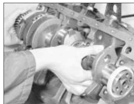
31.6 Placing the crankshaft in position
