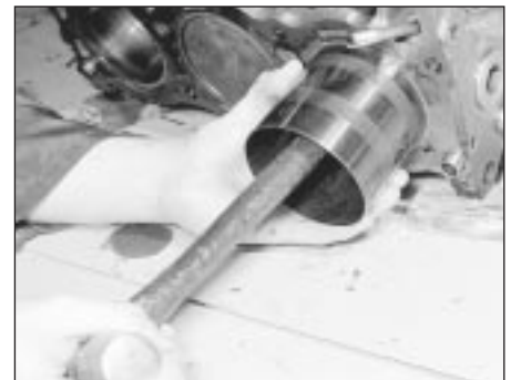
33.8 Tapping a piston into the bore
