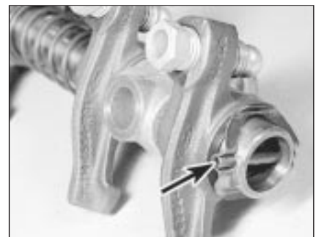
20.1 Rocker shaft roll pin (arrowed)
