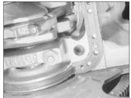
36.28 Sump gasket at rear main bearing cap
