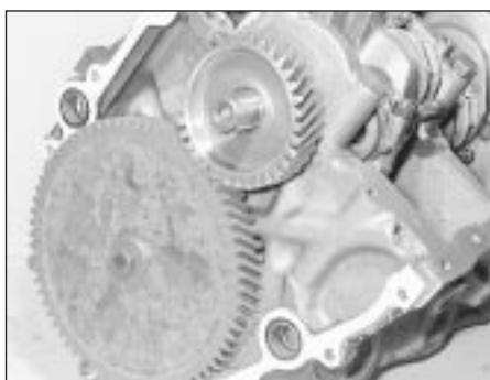
36.7a Timing cover gasket in position
