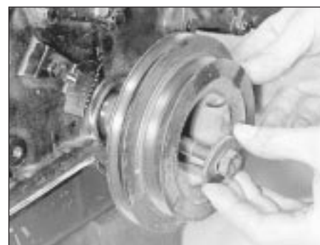
36.9 Fitting the crankshaft pulley
