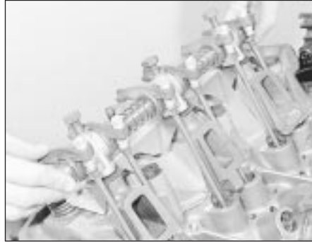
38.7b Fitting an assembled rocker shaft
