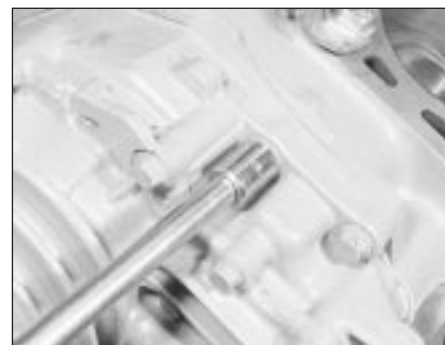
10.36 Removing a timing cover retaining bolt
