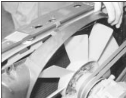
10.22b Removing radiator upper shroud
