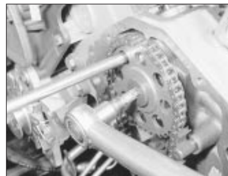
10.39 Slackening camshaft sprocket retaining bolt
