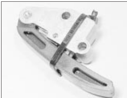
36.21 Timing chain tensioner retracted using a cable-tie
