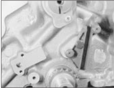
36.15 Crankshaft and camshaft key and slot alignment
