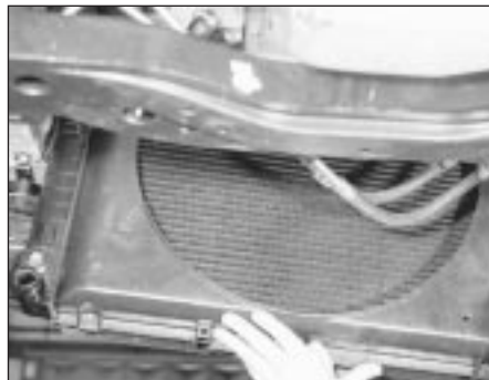
10.22c Manoeuvre the radiator out from under the vehicle
