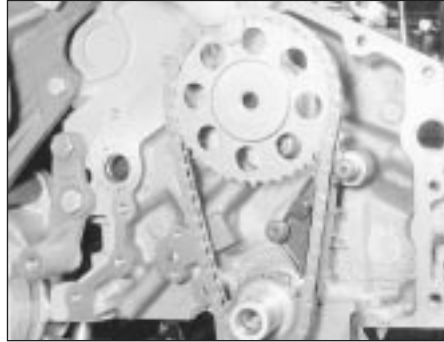
36.18 Fitting timing chain and sprockets
