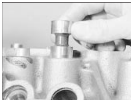
38.1 Fitting a tappet in the block
