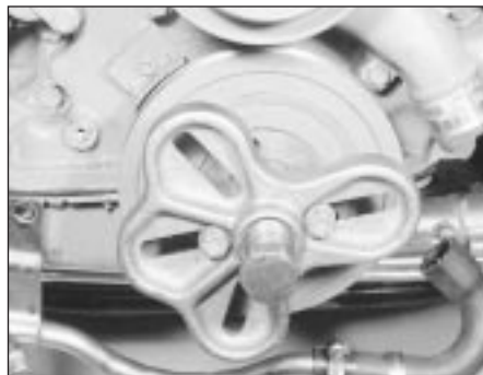
10.27b Using a puller to withdraw the vibration damper
