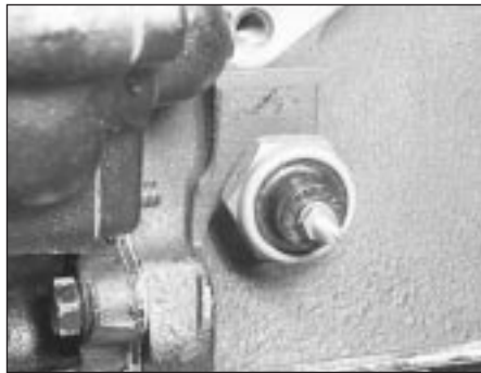
7.1 The oil pressure switch is on the left-hand side of the block
