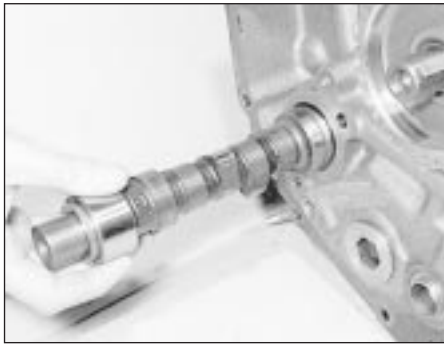
32.3a Fitting the camshaft into the cylinder block
