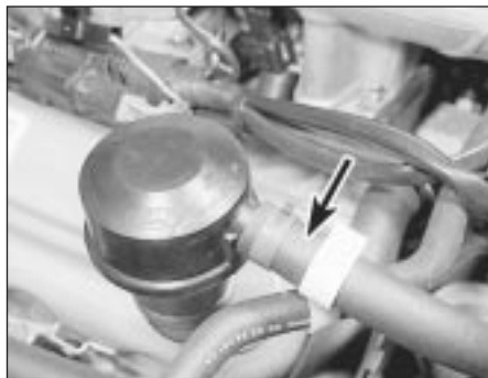
8.15 Oil filler breather hose (arrowed)
