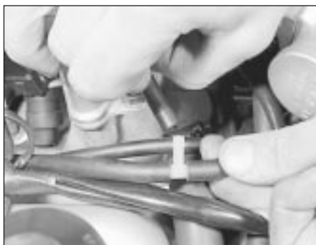
8.22 Vacuum hose T-piece connector
