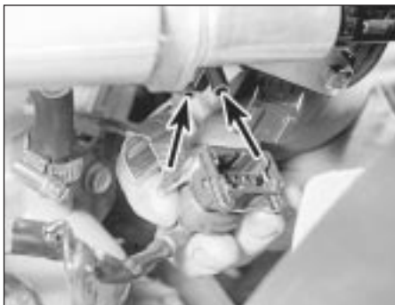
8.14b Throttle position sensor wiring plug Vacuum nozzles arrowed
