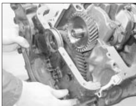
36.7b Fitting the timing cover
