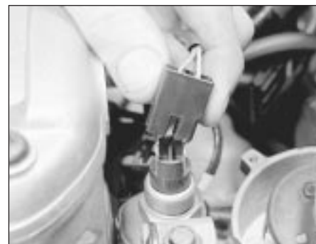
8.19b Disconnecting the fuel temperature sensor wiring plug
