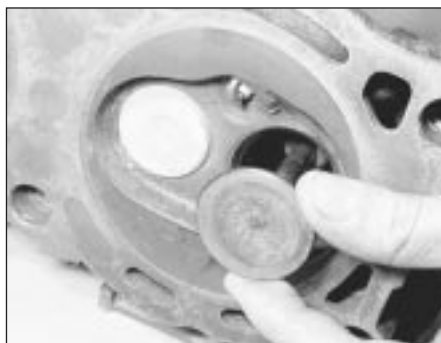
23.2c Removing an inlet valve
