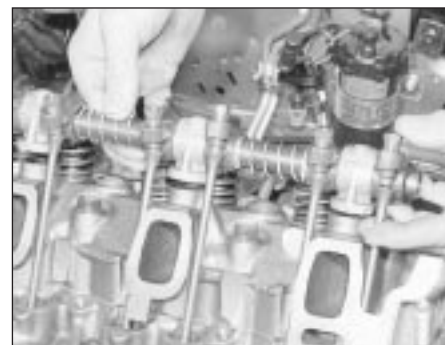
8.29 Removing rocker shaft and pedestal
