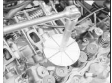
38.16 Tightening a cylinder head bolt using an angular tightening disc
