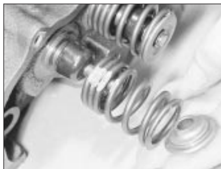
23.2b Removing the spring retainer and spring
