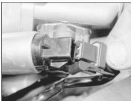
8.18b Disconnecting the idle speed control valve wiring plug
