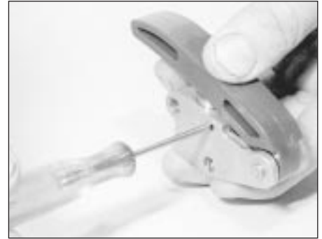
36.20 Releasing timing chain tensioner pawl
