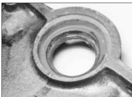
36.1 Timing cover oil seal
