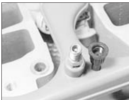
8.20 Fuel rail vent (depressurising) valve and cap
