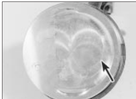
30.10a Cut-out (arrowed) in piston crown . . .
