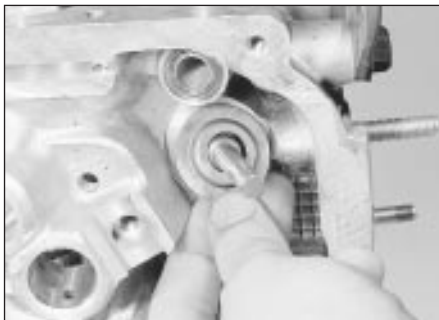
21.3a Remove the spring seat . . .
