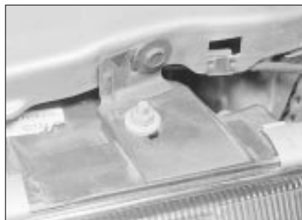
41.10b . . . the upper securing nut . . .
