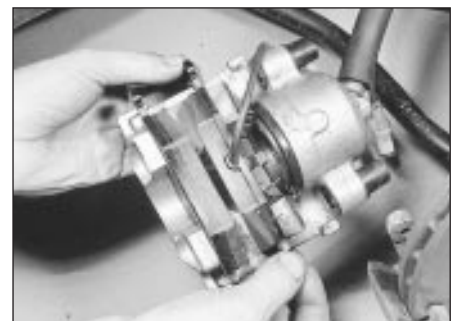
4.19 Withdraw the disc pads from the caliper - Teves caliper
