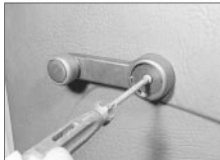
17.1a Prise the cover from the window handle, remove the securing screw ...
