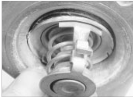
7.17 Correct orientation of thermostat with flow direction arrow pointing towards pressure relief valve
