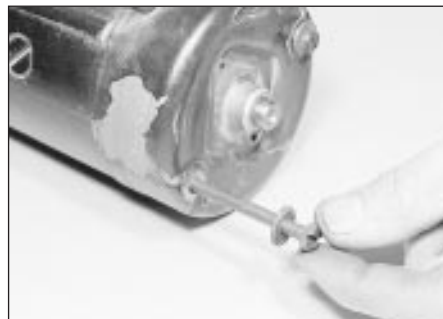
10.4a Remove the commutator end housing securing screws - Bosch long frame starter motor
