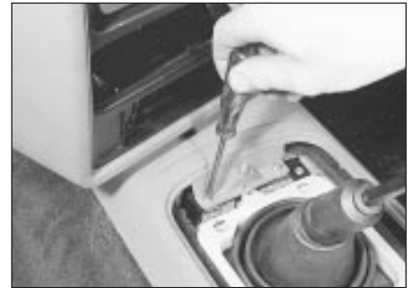
44.6a Removing a lower console panel front securing screw . . .
