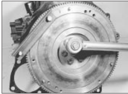
26.12 Use a strap to prevent the flywheel turning as its securing bolts are tightened
