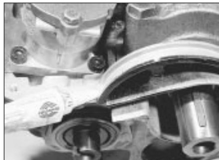
29.15a Apply sealing compound . . .
