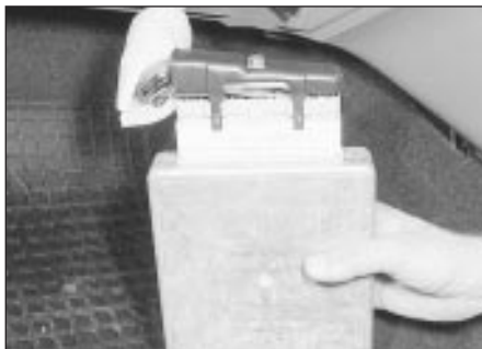
18.39 Engine management module withdrawn from its mounting bracket
