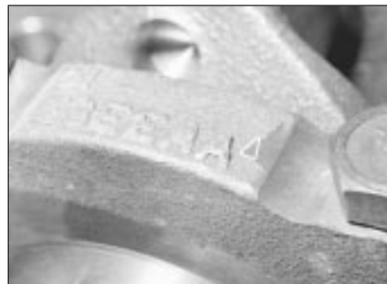
32.22a The arrows on the bearing caps must point towards the front of the engine - 1.8 litre (R2A)
