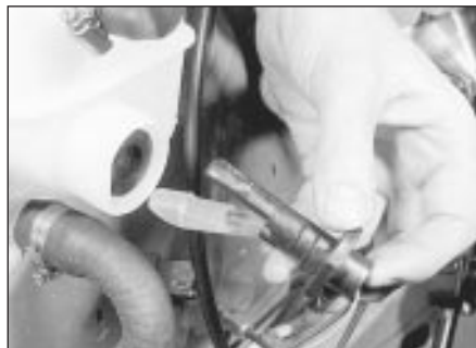
15.8b Fitting the coolant level sensor
