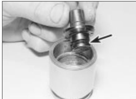
7.10e . . . and finally the adjuster nut itself. Note the seal (arrowed) on the nut
