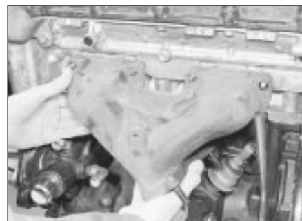
26.8c Fitting the exhaust manifold - DOHC models
