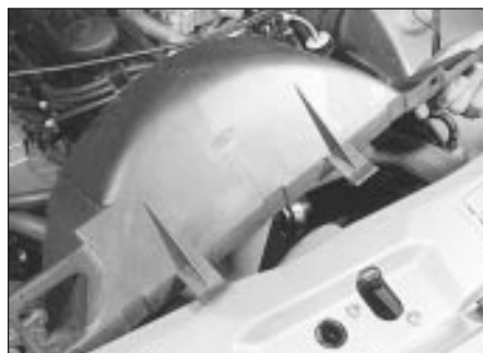
12.2b . . . and withdraw the upper section of the fan shroud
