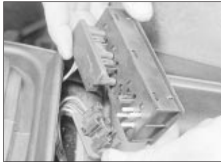
49.2 Disconnecting the wiring plug from a centre console-mounted electric window switch - models from 1987
