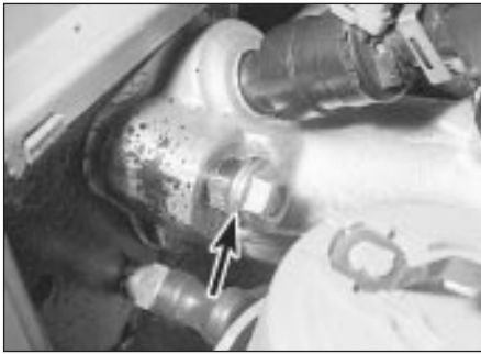
30.13 Where necessary use two nuts locked together (arrowed) to remove the front inlet manifold stud
