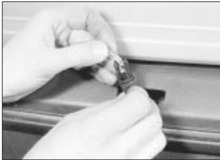
48.41 Removing a rear number plate lamp bulb - Saloon, Hatchback and Estate models
