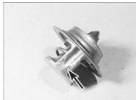
7.9 Thermostat flow direction markings (arrowed)
