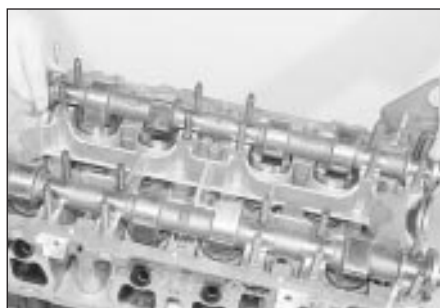
18.14b Lifting out the exhaust camshaft
