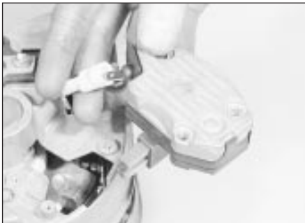
7.14 Disconnect the wiring plug and withdraw the regulator/brushbox - Lucas A127 alternator
