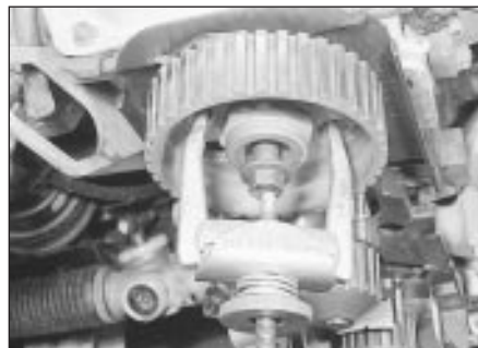
18.12 Using a puller to remove the camshaft sprocket - 1.8 litre (R2A)
