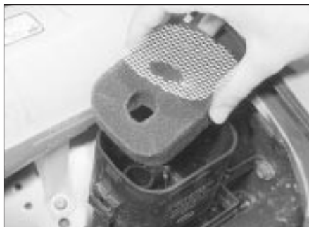
37.2 Withdrawing the pulse-air filter element and gauze - 1.6 litre CVH models
