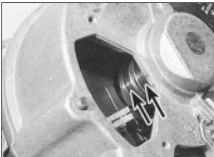
7.4 Inspect the condition of the slip rings (arrowed) - Bosch alternator
