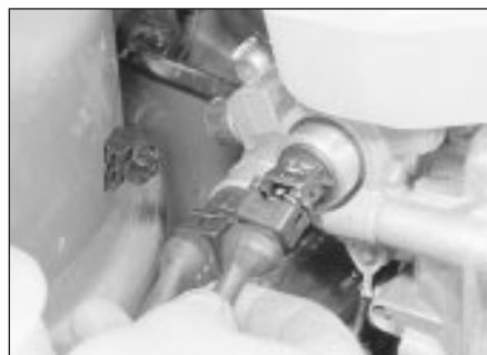
16.3b . . . the main valve multi-plug . . .
