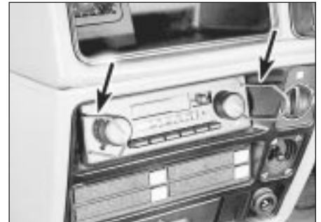
57.10 Removing a radio/cassette player using special tools - DIN fixing
