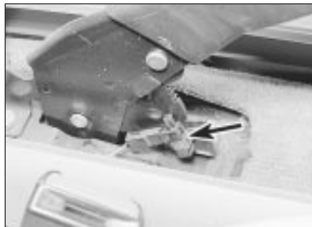
14.3 Handbrake "on" warning lamp switch location (arrowed)
