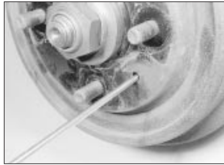
5.5b Releasing the automatic adjuster using a screwdriver
