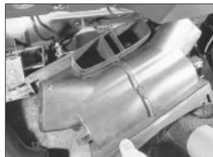
18.9 Withdrawing the heater
