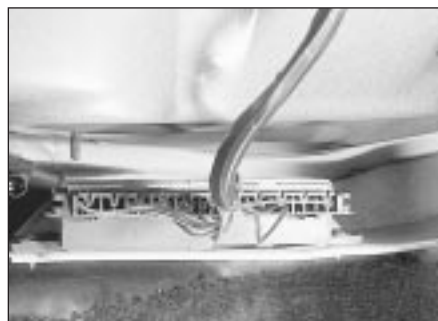
23.15 Auxiliary warning system control unit location
