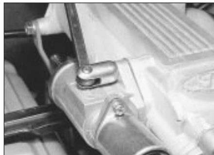
13.3 Unscrewing an idle speed control valve retaining nut
