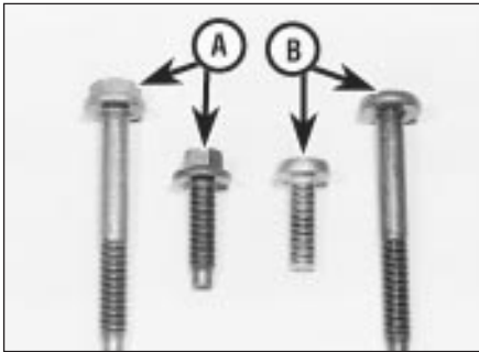
18.26 Use new M8 (auxiliary) cylinder head bolts with hexagonal heads (A), not earlier-type Torx bolts (B)
