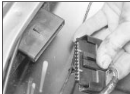
18.22 Disconnecting the ignition module wiring plug
