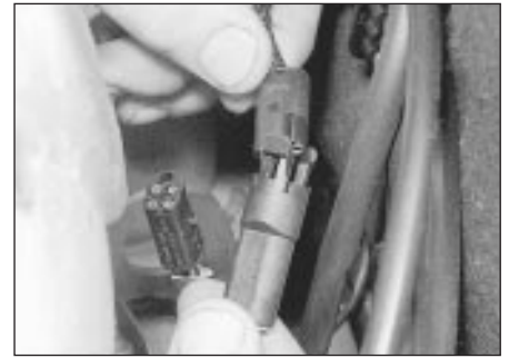
30.6 Disconnecting a fuel injection harness wiring plug
