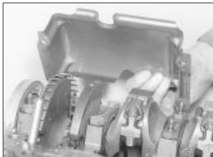
29.3 Withdrawing the oil baffle
