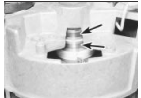
7.16 Inspect the condition of the slip rings (arrowed) - Lucas A127 alternator
