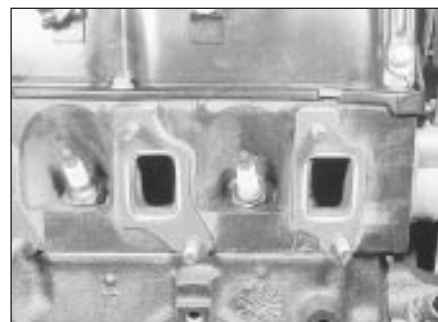
26.6d SOHC models have separate manifold gaskets for each exhaust port
