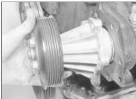
9.32 Withdrawing the coolant pump from the cylinder block (engine removed)
