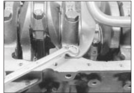
30.2 Unscrewing the oil pick-up tube securing bolt
