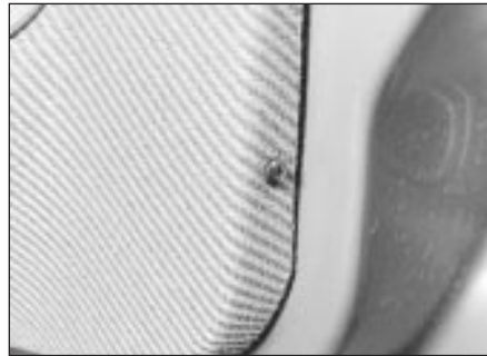
17.15a Trim panel securing screw at bottom rear edge of door
