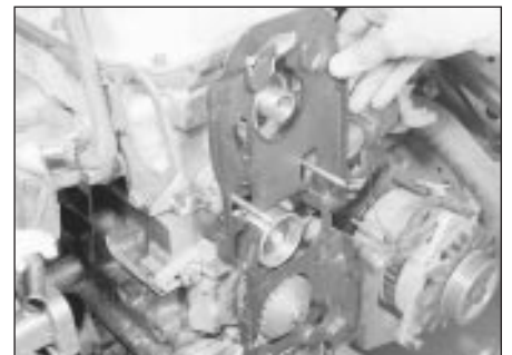
18.13 Removing the timing belt backplate - 1.8 litre (R2A)
