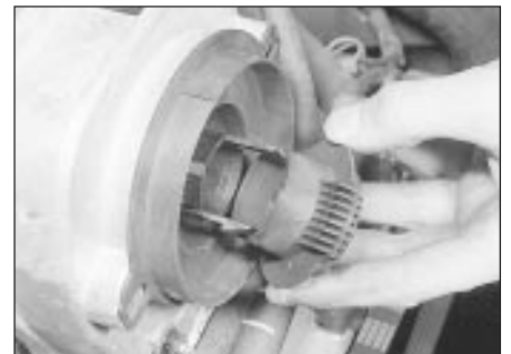
14.8 Removing the rotor arm
