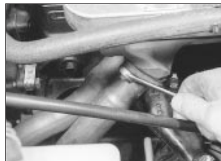
26.4 Unscrewing an exhaust downpipe securing nut
