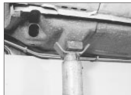
Axle stand correctly positioned under front jacking point - Hatchback model
