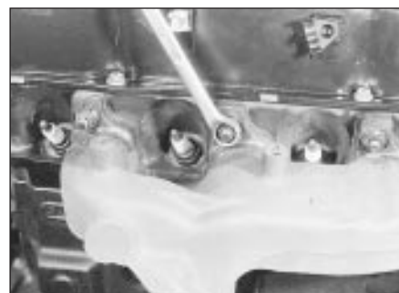
26.6a Unscrew the exhaust manifold securing nuts . . .
