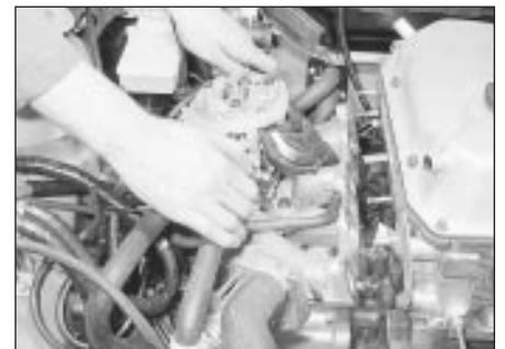
19.10 Withdraw the inlet manifold - 1.8 litre (R2A)
