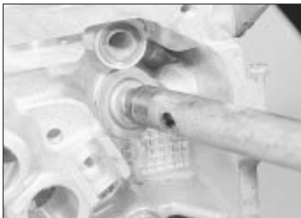
21.7 Seat each new valve seal using a metal tube - 1.8 litre (R2A)
