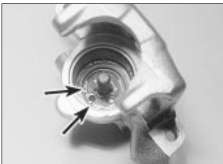
7.15 Remove the circlip (ends arrowed) to release the pushrod and key plate
