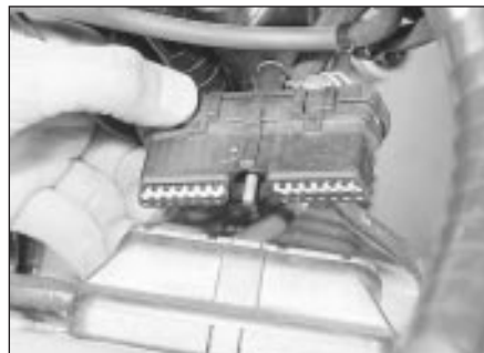
18.3c Disconnecting ESC Hybrid module wiring plug
