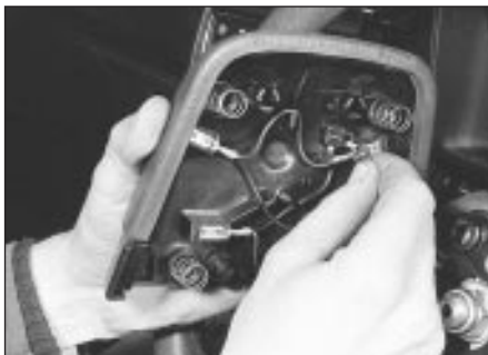
22.2 Prise off the steering wheel trim insert and disconnect the horn electrical lead
