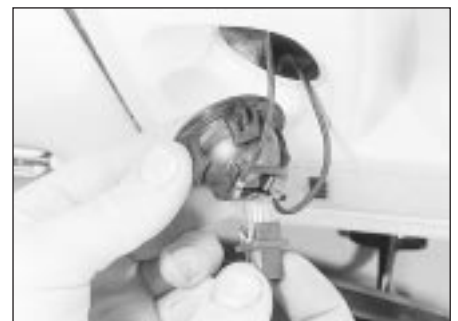
27.6 Removing a map reading lamp bulb
