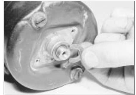
10.3a Remove the C-clip . . .
