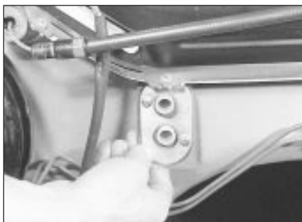
18.5 Heater pipe cover
