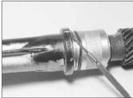
15.12 Removing distributor driveshaft O-ring - Motorcraft distributor
