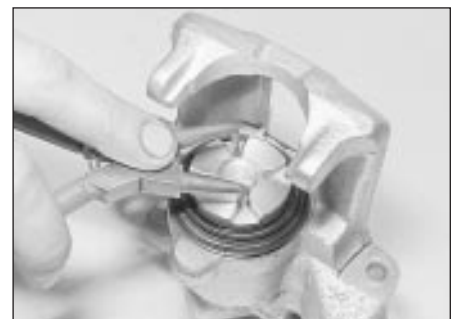
4.32 Retracting the piston using circlip pliers
