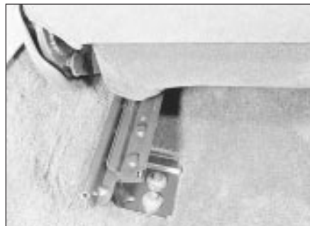
47.2 Front seat inner rear mounting
