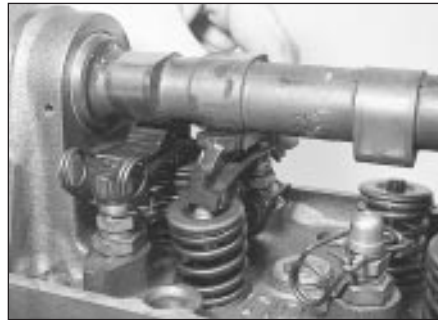
24.5 Note how the cam follower retaining springs are fitted
