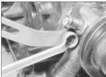
9.8 Location of the alternator adjusting link under the right-hand retaining bolt
