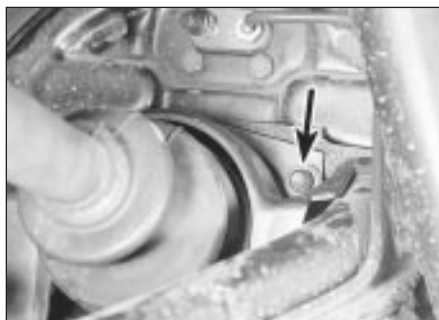
14.4 Remove the nylon fasteners (arrowed) to free the plastic shield from the brake backplate
