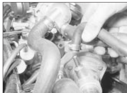
7.12c . . . and the expansion tank hose
