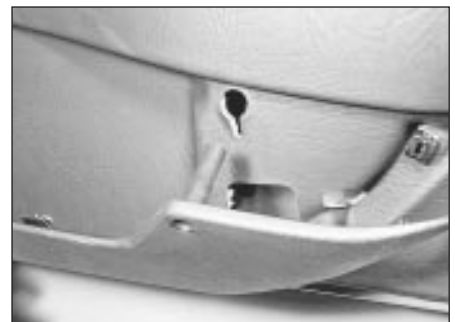
17.4 Withdraw the door pocket
