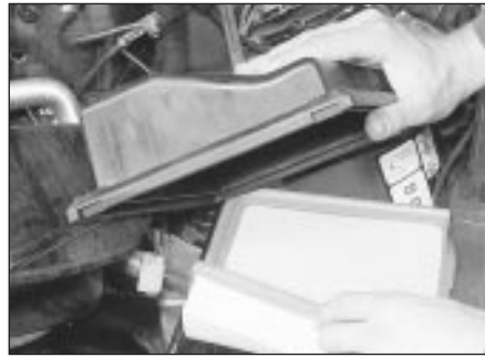
38.19 Lifting out the air cleaner element
