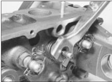
22.2a Compressing a valve spring
