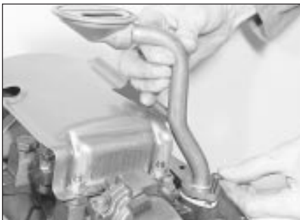
29.2 Removing the oil pick-up pipe
