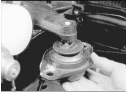
17.4 Withdrawing an engine mounting
