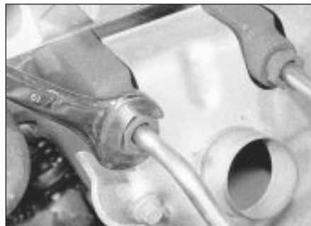
22.4 Unscrewing a pulse-air delivery tube union
