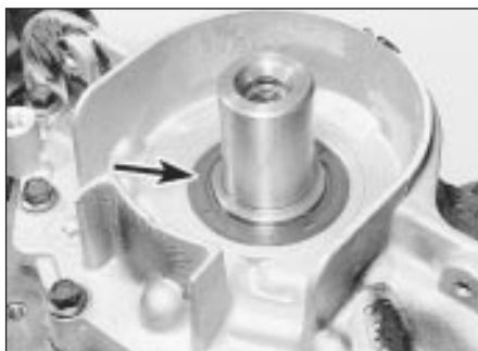
25.5 Crankshaft front oil seal (arrowed) located in oil pump housing - 1.8 litre (R2A)
