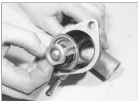
7.6b . . . and extract the thermostat . . .
