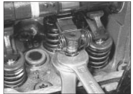
23.7b Adjusting a valve clearance
