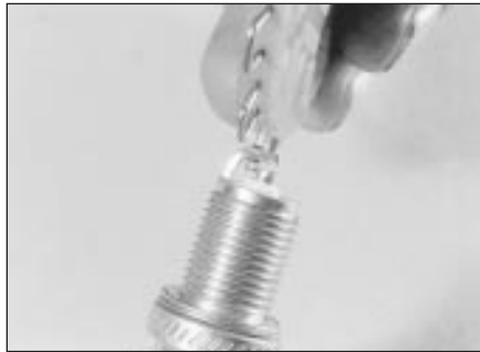
11.9c Adjusting a spark plug gap using a special tool
