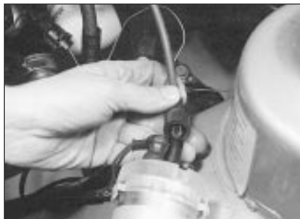
12.7 Disconnecting the HT lead from the coil
