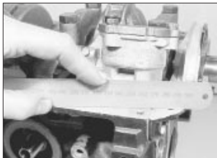
27.5b Checking the alignment of the crankshaft front oil seal housing
