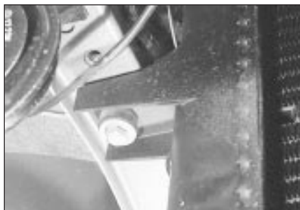
5.10b Lower radiator mounting bolt
