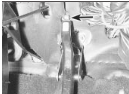
11.3 Throttle pedal assembly - cable connection arrowed
