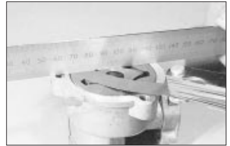
31.11 Checking the oil pump rotor endfloat
