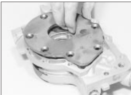
29.2 Remove the oil pump cover
