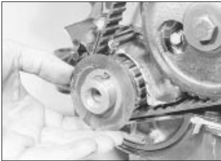
19.9 Removing the guide washer from the crankshaft
