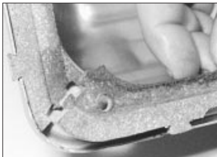
23.9a Camshaft cover gasket dovetails
