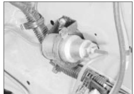
23.1b Later type deceleration sensitive valve
