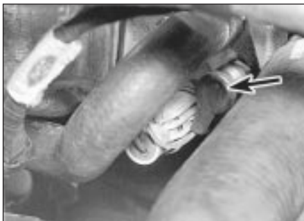
16.1 Temperature gauge sender location (arrowed)
