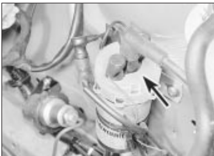
12.1 Ignition coil - CVH model. Plastic cover arrowed
