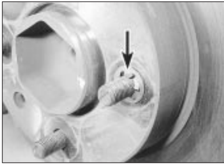
5.5a Brake drum retaining spire washer (arrowed)
