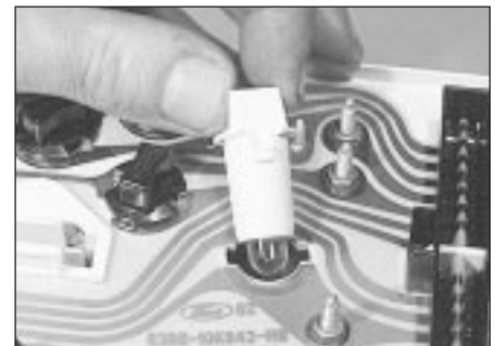
21.3b Removing an instrument panel illumination bulb - bulb is integral with bulbholder
