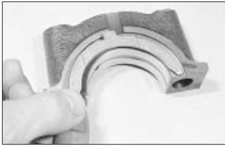
34.24 Fitting a thrustwasher to the centre main bearing cap
