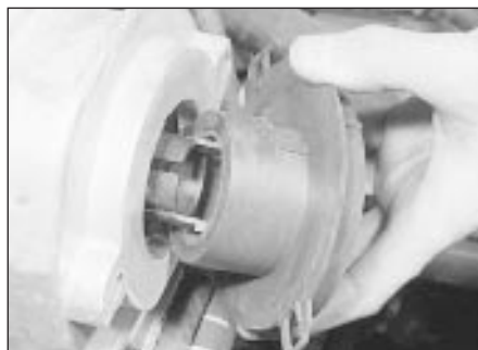
14.9 Removing the rotor housing
