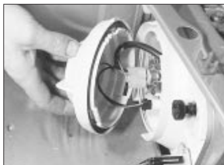
48.2 Remove the headlamp rear cover
