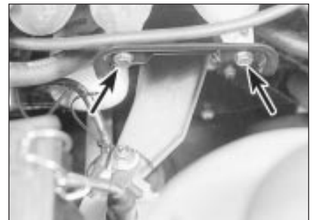
30.12 Lower inlet manifold bracket (arrowed)
