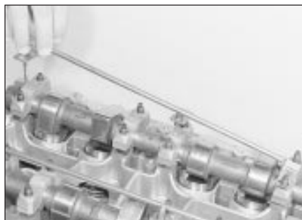
18.13 Lifting off a camshaft oil spray bar
