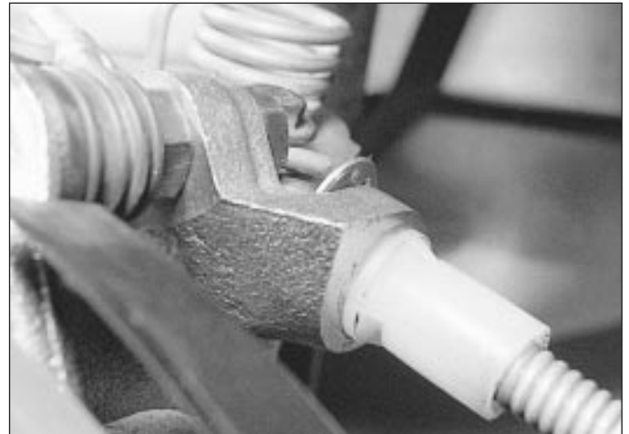
27.5b Handbrake cable-to-caliper carrier bracket attachment - ABS
