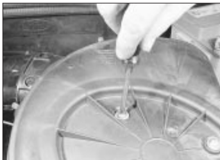
38.1 Remove the air cleaner cover screws . . .
