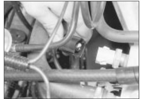
21.5 Disconnecting the engine coolant temperature sensor wiring plug
