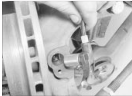
22.3 Unscrew the mounting bolt and withdraw the front wheel sensor - ABS
