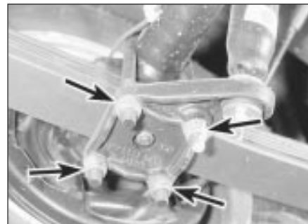
19.3 Unscrew the nuts (arrowed) from the rear axle-to-leaf spring U-bolts
