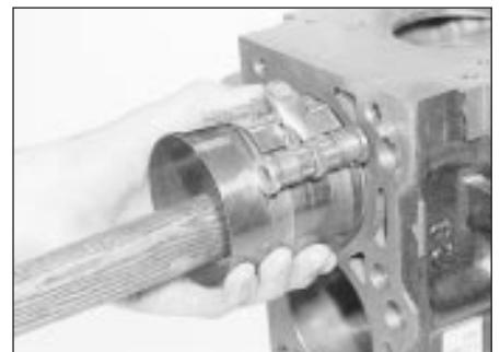
30.10d Fitting a piston and connecting rod into the cylinder bore - 1.8 litre (R2A)
