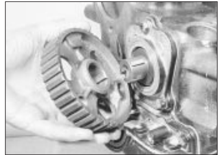
19.13 Removing the auxiliary shaft sprocket
