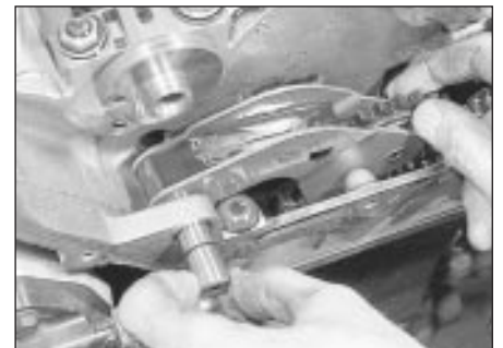
18.9b Withdrawing the pivot pin from the chain tensioner arm
