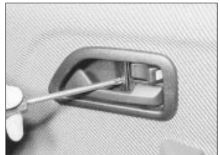
17.9 Remove the interior door handle surround securing screws
