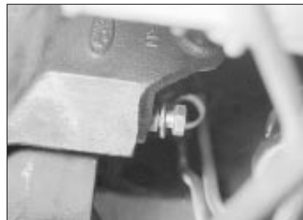
29.14b Power steering pump rear securing bolt
