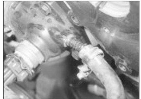
7.20a Disconnect the coolant hoses . . .
