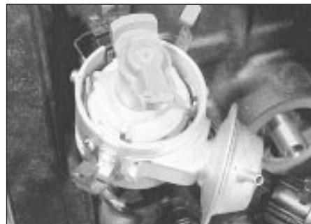
15.7b Rotor arm tip aligned with scribed line on distributor body - Bosch distributor
