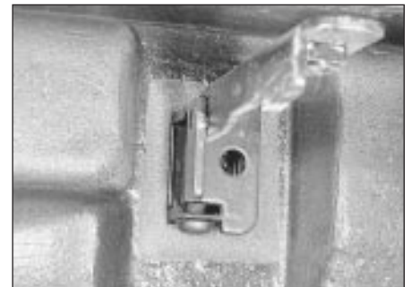
30.12b Front bumper height adjusting screw - models from 1987
