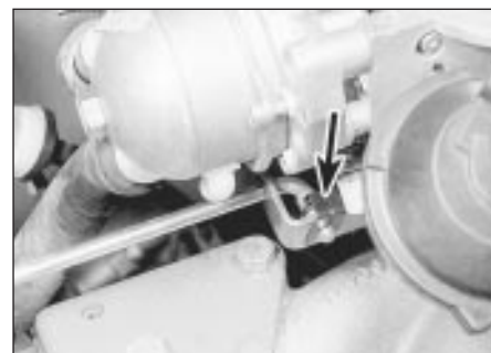
19.4 Throttle arm retaining clip (arrowed) - Pierburg 2V carburettor
