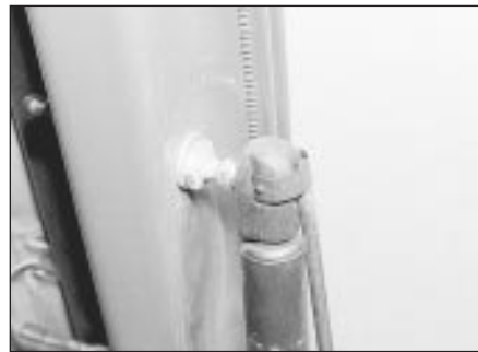
11.5 Prising out a tailgate strut retaining clip
