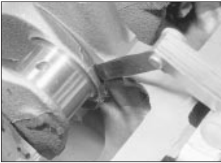
32.6 Checking crankshaft endfloat - 1.8 litre (R2A)
