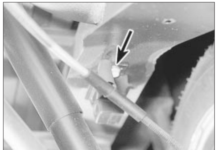
27.7 Handbrake cable support spring (arrowed)
