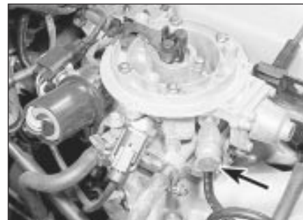
4.4 CFI unit fuel inlet union (arrowed)
