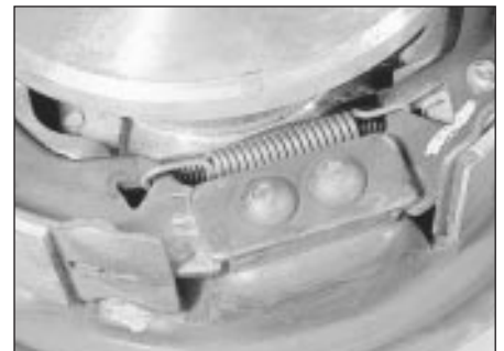
5.6b Bottom shoe return spring
