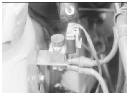
20.18 Throttle damper control solenoid - ESC Hybrid system
