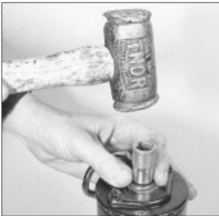
10.30 Use a soft faced hammer and socket to fit a new star clip to the end of the armature shaft - Lucas 5M90 starter motor
