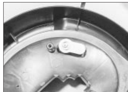
36.3b Air cleaner heat sensor viewed from inside air cleaner - OHC models
