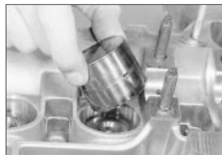
18.15 Withdrawing a cam follower
