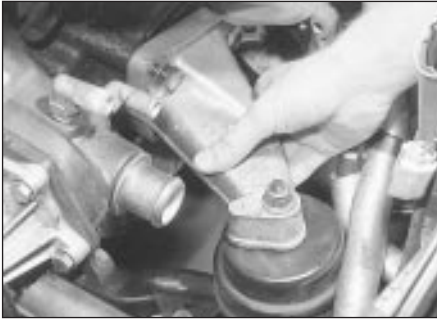
5.36 Remove the engine mounting brackets to improve clearance
