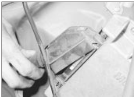
18.3b Disconnecting ESC II module wiring plug
