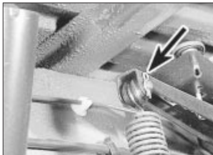
18.7 Remove the split pin (arrowed) from the brake load apportioning valve lever
