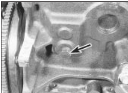
46.7 Cylinder block drain plug (arrowed) - SOHC models (engine removed)
