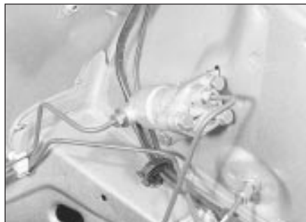
23.1a Early type deceleration sensitive valve
