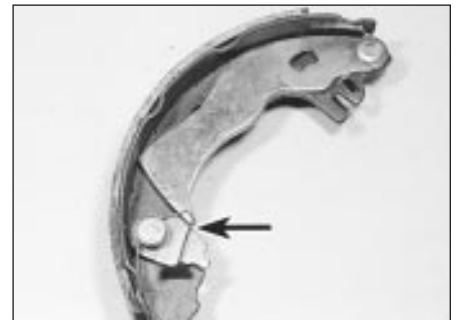
5.13 Fully retract the self-adjuster ratchet (arrowed) before refitting the trailing shoe
