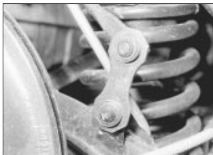
17.2 Anti-roll bar-to-lower arm connecting strap
