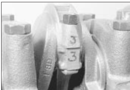
32.2 Big-end cap and connecting rod identification numbers
