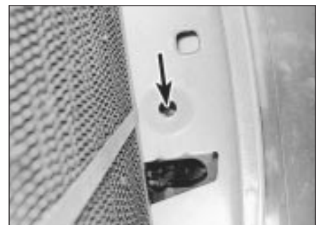
7.9 Access hole (arrowed) below bonnet lock
