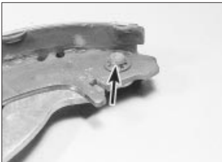
5.11 Handbrake lever-to-trailing shoe securing clip (arrowed)
