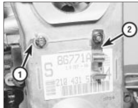
18.29 Earth tag (1) and coolant hose clip (2) locations on timing cover - 1.8 litre (R2A)
