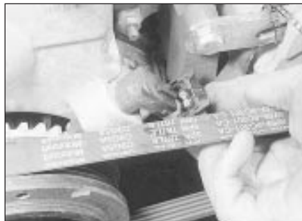
20.3 Disconnecting crankshaft speed/position sensor wiring plug - ESC Hybrid system
