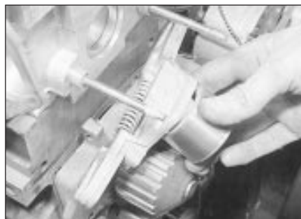
9.20 Remove the timing belt tensioner
