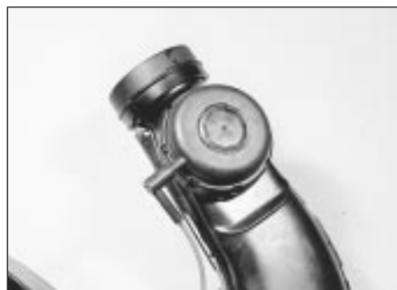
36.3a Air cleaner vacuum diaphragm unit - OHC models
