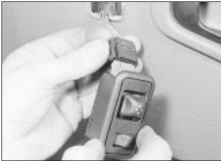
10.3 Disconnect the wiring plug from the door mirror switch - models up to 1987
