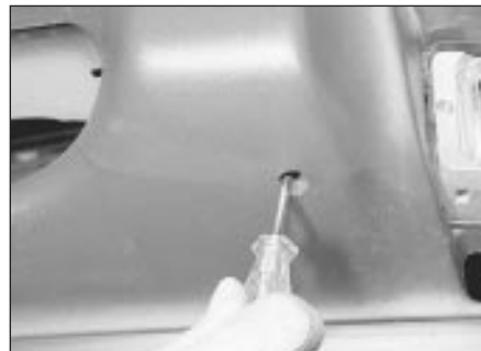
30.12a Adjusting the height of a front bumper - models from 1987
