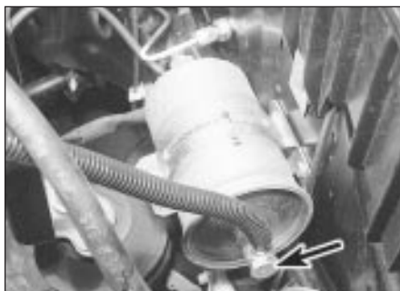
41.1 Fuel filter location - outlet union arrowed
