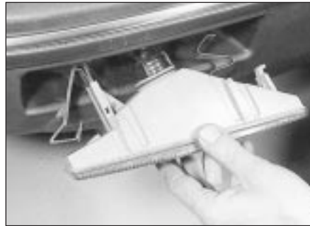
44.3 Withdrawing a front direction indicator lamp unit - "low specification" models up to 1987
