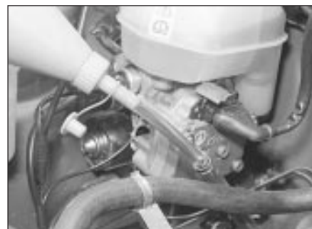
17.4 Topping-up the transmission fluid
