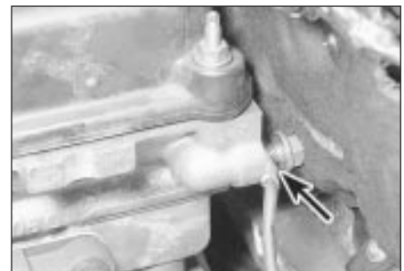
17.7 Disconnect the earth lead (arrowed) from the cylinder head
