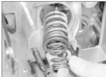
19.1 Withdrawing the double valve springs from the cylinder head
