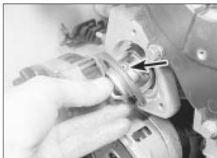
7.26 Thermostat relief valve (arrowed) should be in the 12 o'clock position
