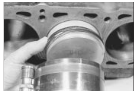
32.10 Fitting a piston ring compressor
