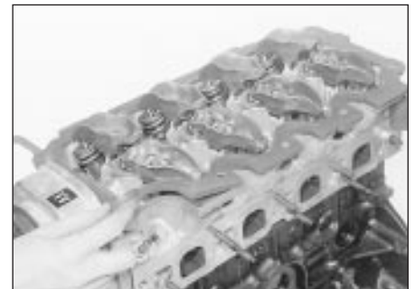
20.14 Ensure that the camshaft cover gasket locates over the edges of the cylinder head - 1.8 litre (R2A)
