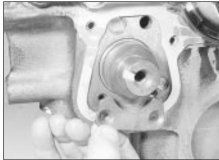
25.5a Unscrew the auxiliary shaft thrustplate securing screws and remove the thrustplate
