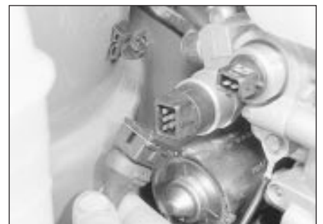
16.3c . . . and the pressure switch multi-plug - ABS
