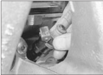
18.23 Lifting a fuel injector from the cylinder head
