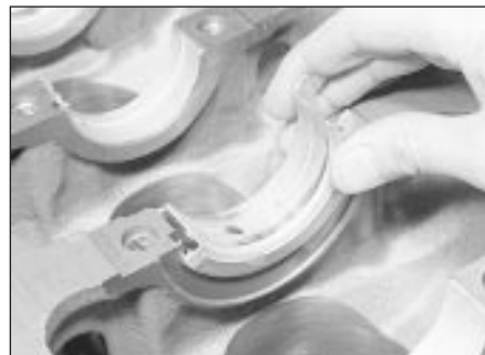
32.13b Centre main thrust bearing shell in cylinder block - 1.8 litre (R2A)
