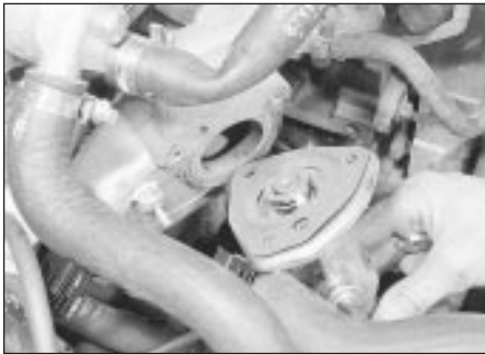
7.13 Removing the thermostat housing and gasket
