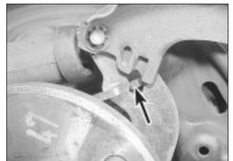
5.15 Engage the hole in the adjuster with the hook on the strut (arrowed)
