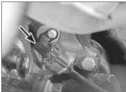
21.9 Crankshaft speed/position sensor (arrowed) viewed from front of engine with shroud removed
