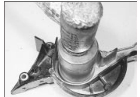
27.4 Using a socket to fit a new crankshaft front oil seal
