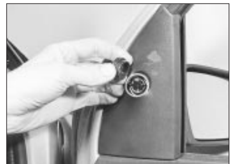
29.1 Unscrew the bezel from the adjuster knob . . .
