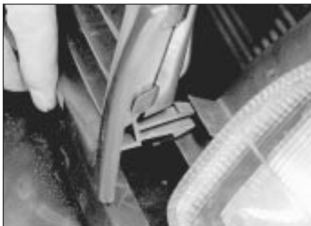
32.8 Removing the later type front grille panel
