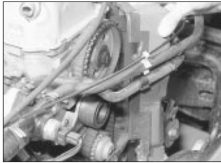
18.33b Removing the upper timing cover - 1.6/1.8 litre (R6A)
