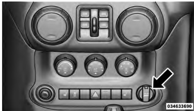
Front Power Outlet
