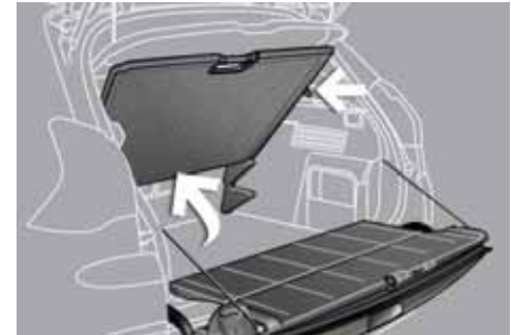
From the high position, place the floor in this position (at an angle), two stops support it to allow access underneath it or to the spare wheel.
