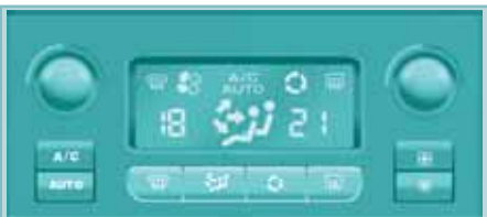
Automatic air conditioning
