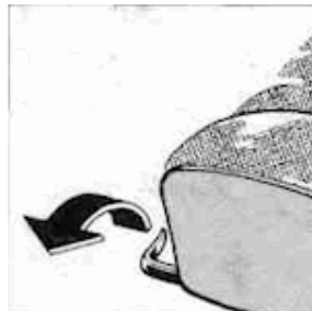
Seat adjustment Pull lever in front of seat.
