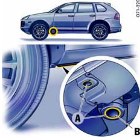
A - Front jacking points platform lift B - Front jacking point garage lift
