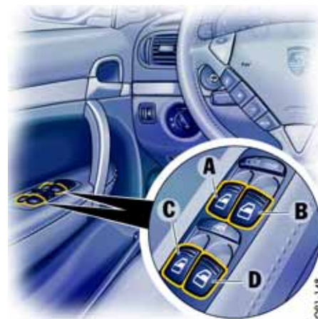
A - Power window in driver's door B - Power window in passenger's door C - Left rear power window D - Right rear power window
