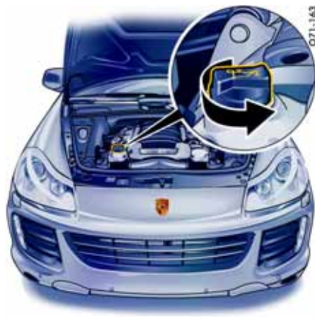
Engine oil filling point on Cayenne S, Cayenne GTS, Cayenne S Transsylvia
