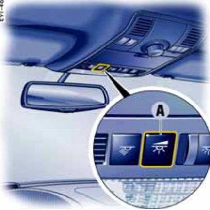
A - Button for dimming the comfort lighting
