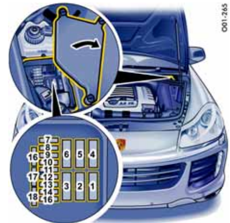
Fuse plan and fuse box in engine compartment
