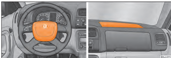
Fig. 102 Driver airbag in the steering wheel/front passenger airbag in the dash panel
