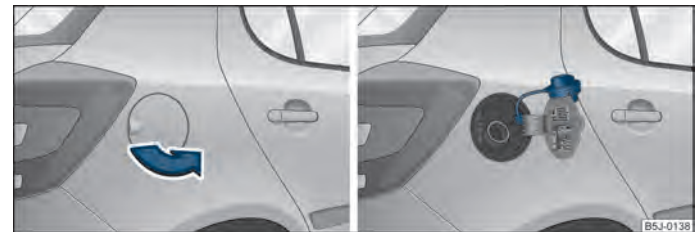
Fig. 125 Right rear side of the vehicle: Fuel filler flap/fuel filler flap with cap unscrewed
