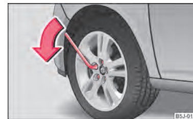
Fig. 142 Changing a wheel: Loosening the wheel bolts ▶
