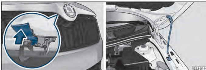
Fig. 127 Radiator grille: Locking lever/securing the bonnet with the bonnet support
