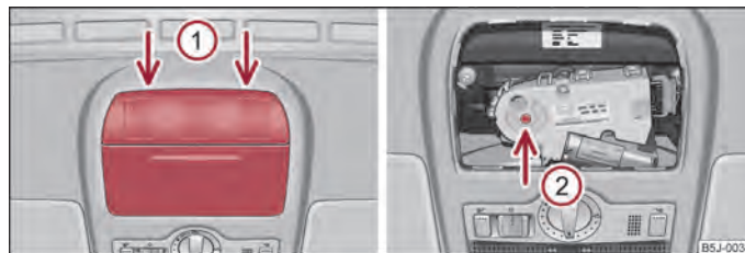
Fig. 21 Detail of the headliner: Points for positioning screwdriver/opening for positioning the key
