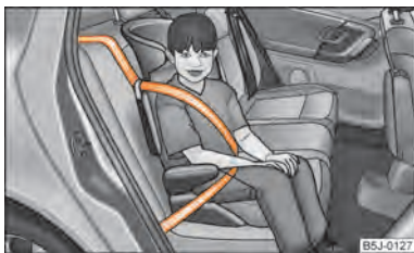
Fig. 114 Child seat in Group 2 installed on the rear seat facing the direction of travel
