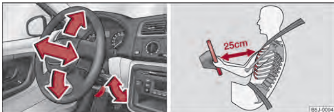
Fig. 81 Adjustable steering wheel: Lever below the steering column/Safe distance to steering wheel
