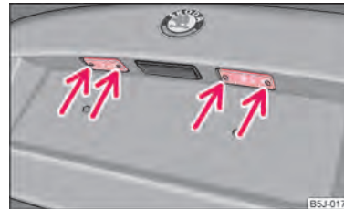
Fig. 164 Remove the licence plate light
