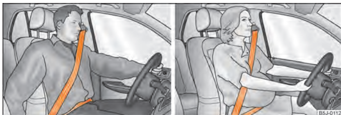
Fig. 99 Routing of belt webbing over the shoulders and the lap belt/Routing of belt webbing for an expectant mother
