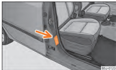
Fig. 110 Sticker on the centre column of the body on the front passenger side.
