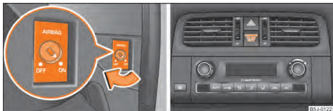
Fig. 109 Switch for the front passenger airbag/indicator light for a switched off front seat passenger airbag
