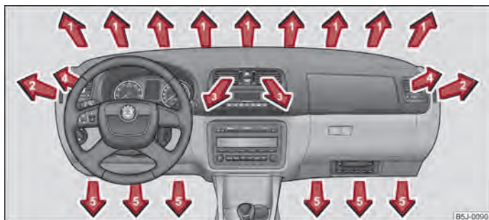
Fig. 77 Air outlet vents
