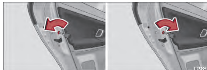
Fig. 11 Switching child safety lock on: for vehicles without or with central locking system
