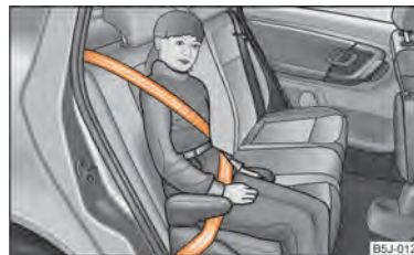
Fig. 115 Child seat in Group 3 installed on the rear seat facing the direction of travel
