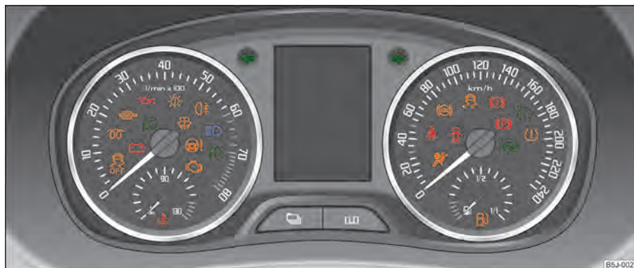
Fig. 8 Instrument cluster with warning lights
