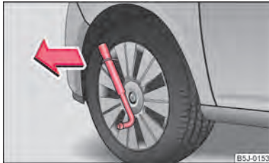
Fig. 140 Removing the full wheel trim
