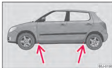
Fig. 143 Changing a wheel: Jacking points for positioning lifting jack
