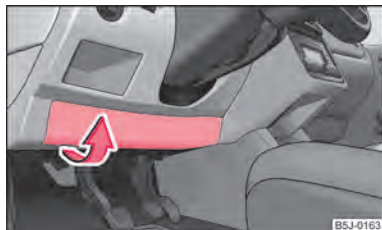
Fig. 151 Bottom side of the dash panel: fuse cover
