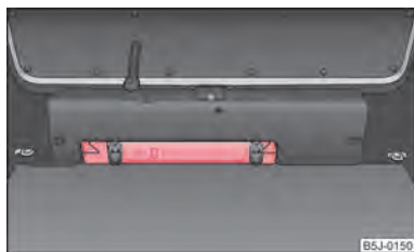
Fig. 137 Placing of the warning triangle
