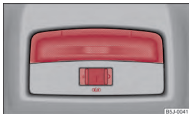
Fig. 28 Interior lighting - version 2
