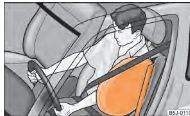
Fig. 106 Inflated side airbag
