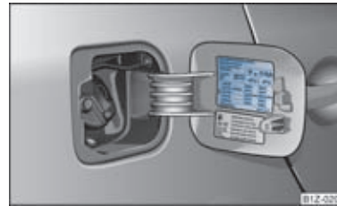
Fig. 157 An opened fuel filler flap with a tyre size and tyre inflation pressure table
