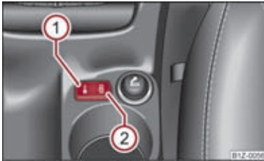
Fig. 13 Centre console: Central locking system
