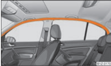
Fig. 127 Installation position of the head airbags
