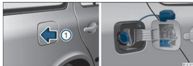
Fig. 147 Right rear side of the vehicle: Open fuel filler flap/fuel filler flap with cap unscrewed ►
