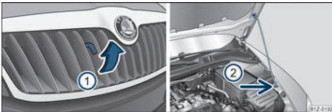
Fig. 149 Radiator grille: Locking lever/securing the bonnet with the bonnet support
