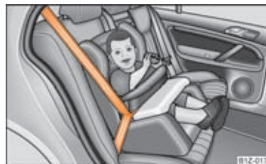
Fig. 133 Child seat with padded table in Group 1 installed on rear seat bench facing the direction of travel
