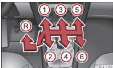
Fig. 100 The shift pattern: 5-speed or 6-speed manual gearbox
