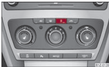
Fig. 96 Button for direct switching on/off of the auxiliary heating (auxiliary heating and ventilation) on the operating part of the air conditioning system
