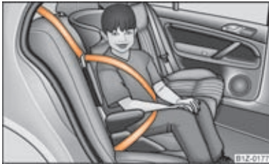
Fig. 134 Child seat in Group 2 installed on the rear seat facing the direction of travel
