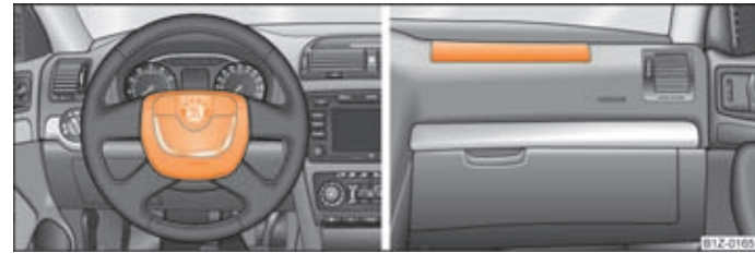
Fig. 122 Driver airbag in the steering wheel/front passenger airbag in the dash panel
