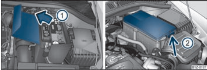
Fig. 154 Engine compartment: Polyester cover of the vehicle battery/plastic cover of the vehicle battery
