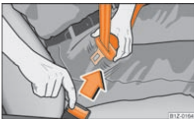
Fig. 121 Releasing lock tongue from belt lock
