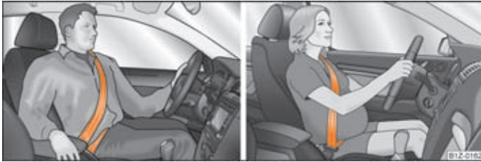
Fig. 119 Routing of belt webbing over the shoulders and the lap belt/Routing of belt webbing for an expectant mother
