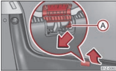
Fig. 17 Emergency unlocking of the boot lid
