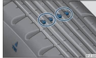
Fig. 158 Tyre tread with wear indicators
