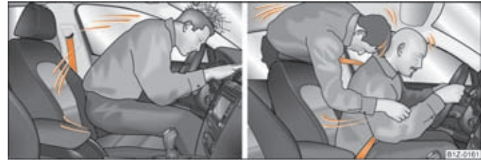
Fig. 118 The driver is catapulted forward if not wearing a belt/The rear seat occupant is catapulted forward if not wearing a belt
