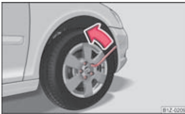
Fig. 166 Changing a wheel: Slackening wheel bolts
