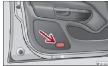
Fig. 33 Front door: Warning light
