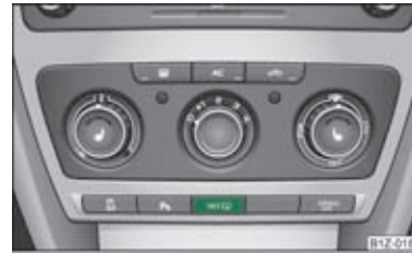
Fig. 140 Button for setting the tyre inflation pressure control value
