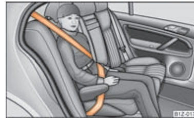
Fig. 135 Child seat in Group 3 installed on the rear seat facing the direction of travel
