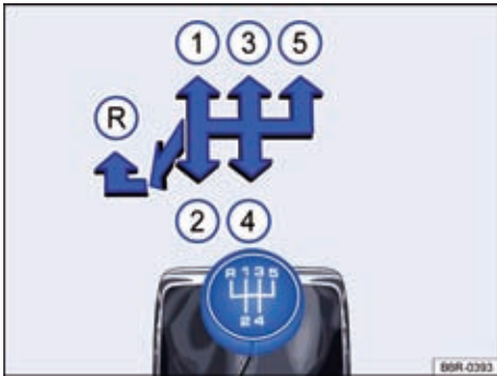
Fig. 69 Shift pattern of the 5-speed manual gearbox.
