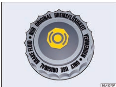
Fig. 73 In the engine compartment: Cover of the brake fluid reservoir.
