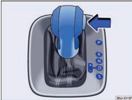
Fig. 70 Selector lever of automatic gearbox with lock button (arrow).
