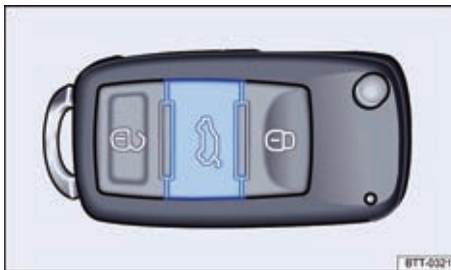
Fig. 19 Vehicle key with unlocking button for the boot lid.
