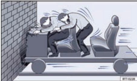
Fig. 32 A vehicle hits the wall with occupants not wearing seat belts.
