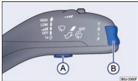
Fig. 10 Button (A) on the windscreen wiper lever to confirm a menu item, and rocker (B) to change the menus.
