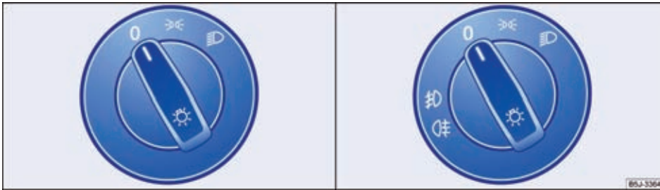
Fig. 45 Beside the steering wheel: Representation of two versions of the light switch.
