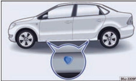
Fig. 111 Jacking points for positioning the jack.
