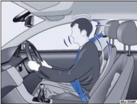
Fig. 35 Driver wearing a seat belt who is caught by the correctly fastened and adjusted seat belt in a sudden braking manoeuvre.
