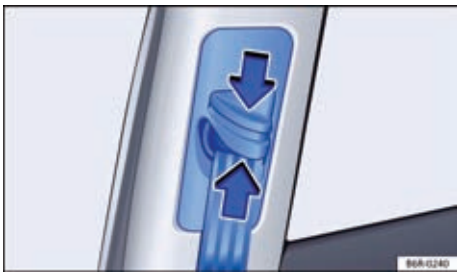
Fig. 40 At the side of the front seats: Seat belt height adjusters.
