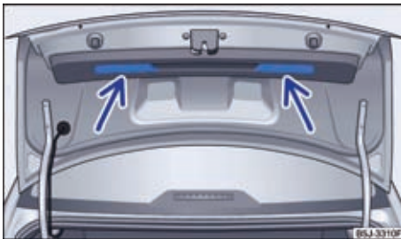
Fig. 21 Open boot lid: Recesses for closing.
