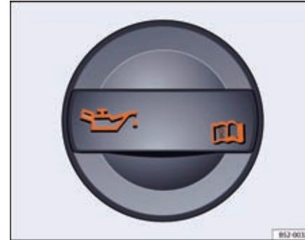
Fig. 85 In the engine compartment: Cap of the engine oil filler opening.
