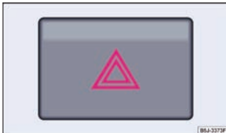
Fig. 99 In the centre of the instrument panel: Switch for the hazard warning light system.
