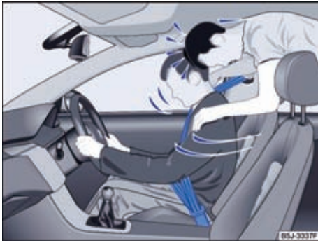
Fig. 34 A passenger not wearing a seat belt on the rear seat is catapulted forward toward the driver wearing a seat belt.
