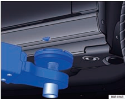
Fig. 97 Front jacking points to lift the vehicle with a lifting platform or car jack.
