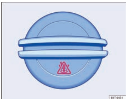
Fig. 87 In the engine compartment: Cap of the engine coolant expansion reservoir.
