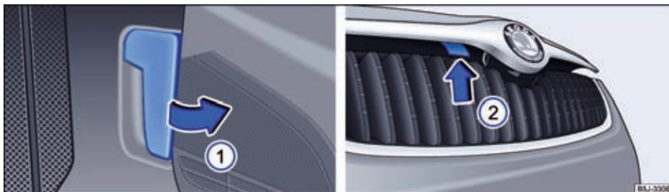
Fig. 82 Left picture: Release lever in the footwell on the driver's side. Right picture: Release lever on the bonnet.
