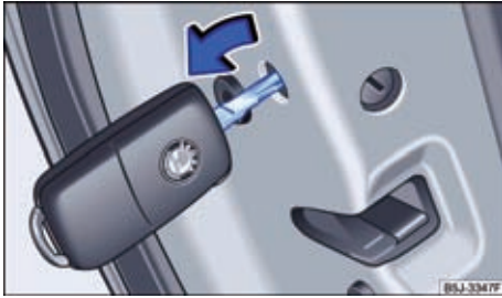
Fig. 102 Emergency locking the vehicle with the vehicle key (the emergency lock is covered by a rubber seal).
