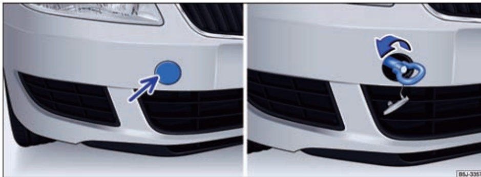
Fig. 125 In the bumper front right: screw in the towing eye. ▶
