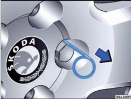
Fig. 108 Pulling off the caps from the wheel bolts.
