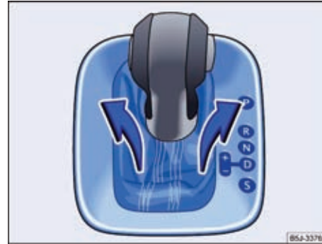
Fig. 103 Remove the cover of the shift gate.
