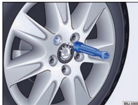
Fig. 113 Changing a wheel: Unscrew the wheel bolts using the hexagon socket in the screwdriver handle.
