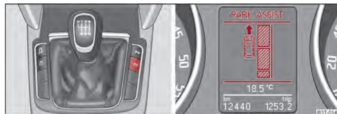
Fig. 122 Switch on display of the park assist in the information display/information display: Finding a suitable parking space
