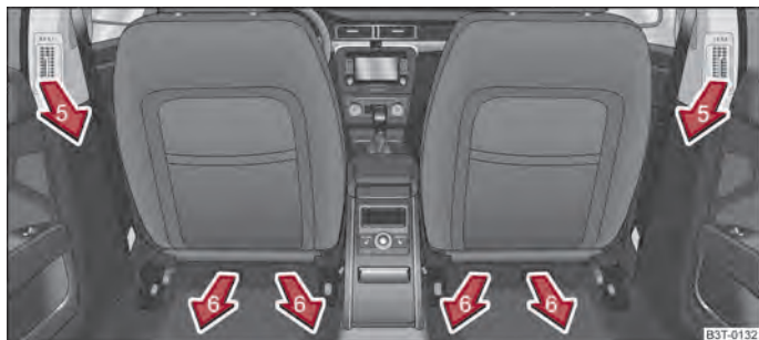
Fig. 109 Air vents at the rear
