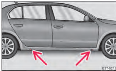
Fig. 189 Changing a wheel: Jacking points for positioning lifting jack
