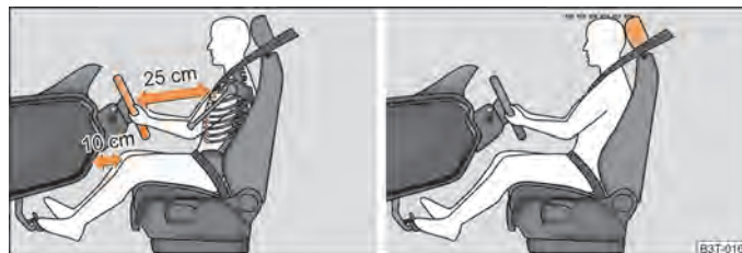
Fig. 138 The correct distance of the driver from the steering wheel and the gear lever/The correct head restraint adjustment for the driver
