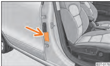
Fig. 153 Sticker on the centre column of the body on the front passenger side.
