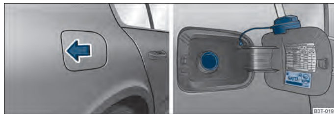
Fig. 169 Right rear side of the vehicle: Open fuel filler flap/fuel filler flap with cap unscrewed
