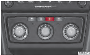
Fig. 112 Button for direct switching on/off of the auxiliary heating (auxiliary heating and ventilation) on the operating part of the air conditioning system
