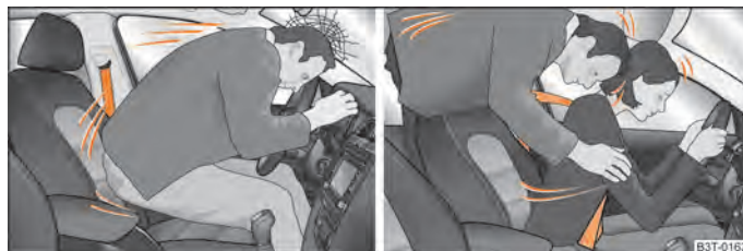
Fig. 140 The driver is catapulted forward if not wearing a belt/The rear seat occupant is catapulted forward if not wearing a belt
