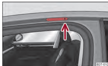
Fig. 85 Attachment points for base roof carrier
