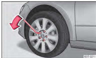
Fig. 188 Changing a wheel: Slackening wheel bolts
