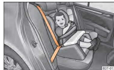
Fig. 156 Child seat with padded table in Group 1 installed on rear seat bench facing the direction of travel
