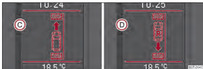
Fig. 124 Information display: Information for engaging the forward gear (C) or the reverse gear (D)
