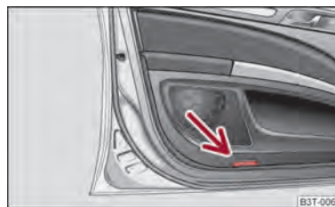
Fig. 45 Front door: Warning light
