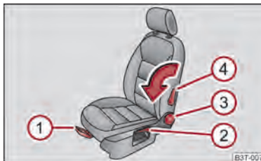
Fig. 56 Controls at seat
