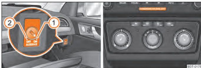
Fig. 152 Storage compartment: Switch for the front passenger airbag/indicator light for a switched off front seat passenger airbag
