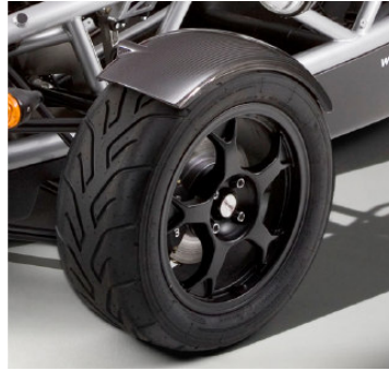
Team Dynamic Pro Race 2.0 5-Spoke "webbed ends" 15 x 7 +35mm offset 16 x 7 +38mm offset Wheel nut type: M12 x 1.5mm Lug nut torque: 80 ft-lbs
