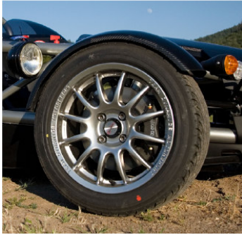
Team Dynamic Pro Race 1.2 12-Spoke 15 x 7 +35mm offset 16 x 7 +38mm offset Wheel nut type: M12 x 1.5mm Lug nut torque: 80 ft-lbs
