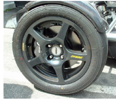
Dymag 5-Spoke Magnesium 15 x 7 +35mm offset 16 x 8 +38mm offset Wheel nut type: M12 x 1.5mm Lug nut torque: 80 ft-lbs
