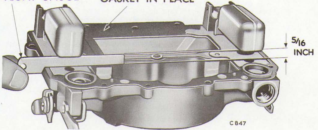
Fig. 17 Checking Float Height
