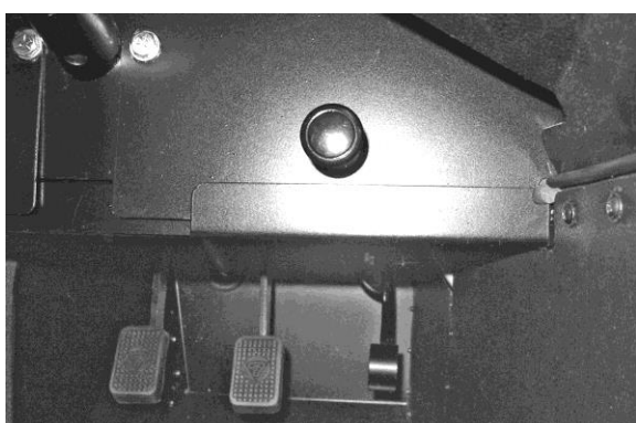
Figure 60: Heater control location
