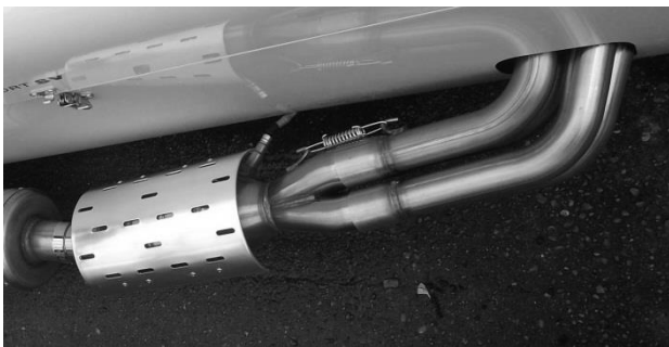
Figure 49: Primary pipes and collector/catalyst
