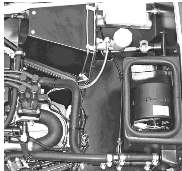
Figure 47: Clutch hydraulic hose
