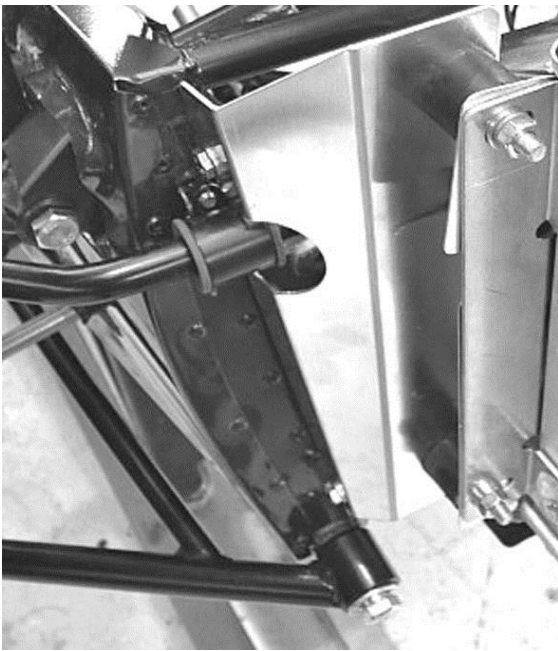
Figure 110: SV radiator arrangement
