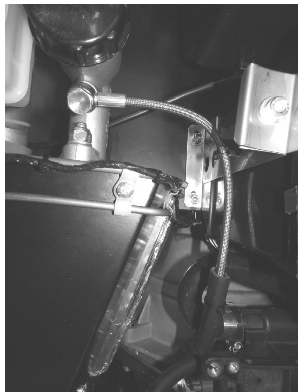
Figure 100: Clutch hydraulic hose
