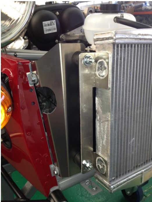
Figure 56: SV radiator arrangement
