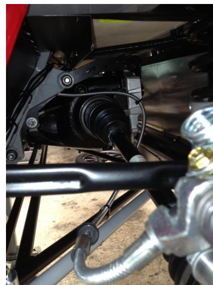
Figure 137: Handbrake cable routing S3 (non-adjustable side)
