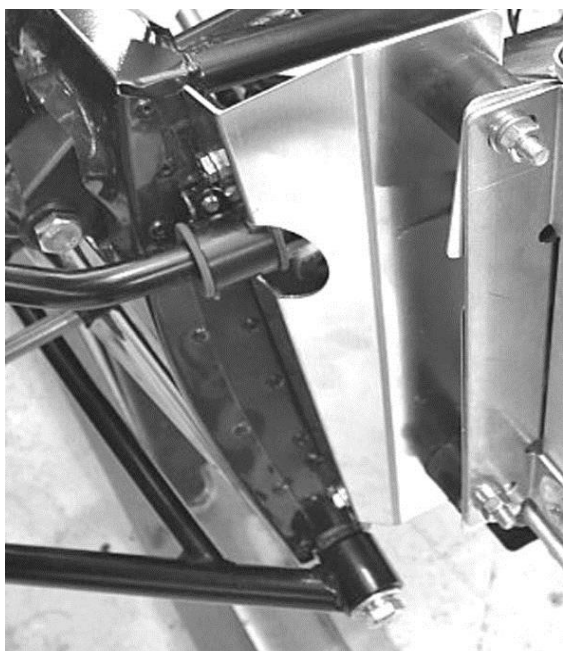
Figure 82: SV radiator arrangement
