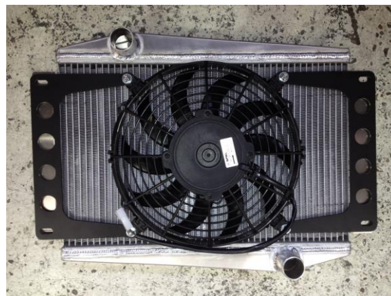
Figure 54: Radiator/fan prior to fitting
