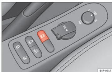
Fig. 134 Centre console: Switch for parking aid.
