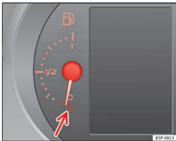
Fig. 27 Instrument panel: fuel gauge
