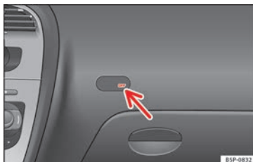
Fig. 20 Control lamp for deactivated front passenger airbag.
