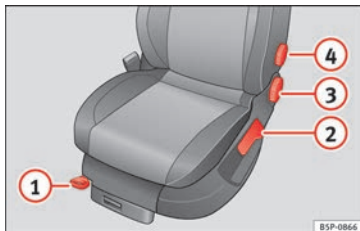
Fig. 74 Front left seat controls
