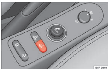
Fig. 32 Centre console: tyre monitoring system button.
