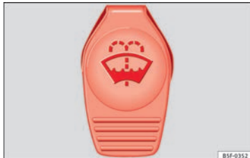
Fig. 150 In the engine compartment: Cap of windscreen washer reservoir
