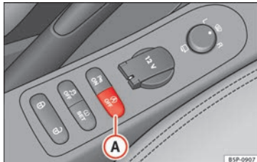
Fig. 132 The Start-Stop function button.
