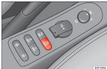
Fig. 121 Centre console: gas system control switch.
