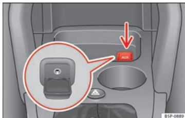
Fig. 99 Auxiliary audio connection.
