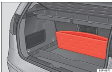
Fig. 109 Variable storage in the boot floor.
