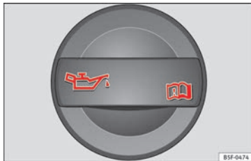
Fig. 148 In the engine compartment: Engine oil filler cap
