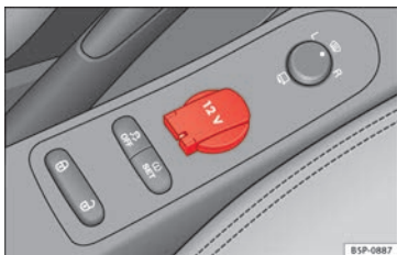
Fig. 97 Power socket, front centre console.
