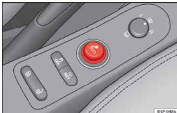
Fig. 96 The cigarette lighter is located in the power socket of the front centre console.
