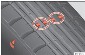
Fig. 152 Tyre tread wear indicators.
