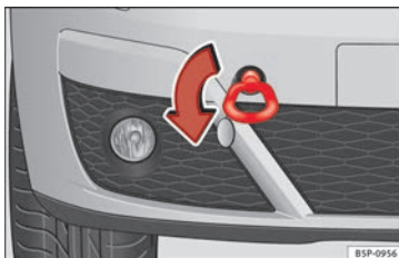
Fig. 165 Fitting the front towline anchorage to the front right section of the vehicle.
