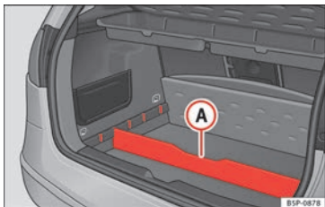
Fig. 110 Boot floor partition.
