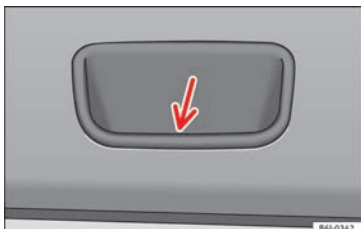
Fig. 54 Close-up of the inside trim of the rear lid: hand grip
