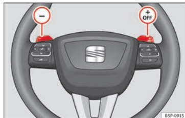
Fig. 129 Steering wheel with paddle shifters for automatic gearbox.
