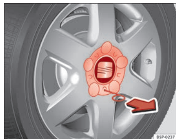
Fig. 155 Changing a wheel: remove the wheel trim.
