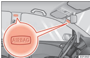
Fig. 17 Location of head-protection airbags on the left side of the vehicle
