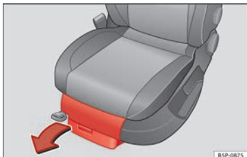
Fig. 85 Storage compartment under the front seats.
