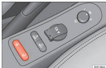
Fig. 47 Detailed view of the centre console: central locking button.
