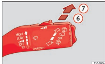
Fig. 71 Windscreen wiper lever: rear window wiper.
