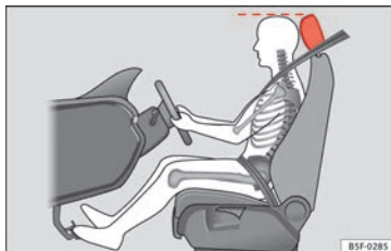
Fig. 2 Correct head restraint position for the driver.
