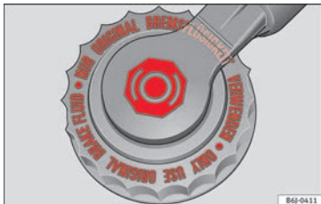
Fig. 151 Engine compartment: brake fluid reservoir cap
