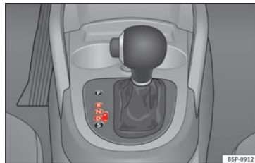
Fig. 126 Centre console: automatic gearbox selector lever.
