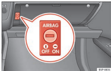
Fig. 19 In the glove compartment: Switch for activating and deactivating the front passenger airbag
