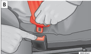
Fig. 14 Positioning and removing the seat belt buckle.
