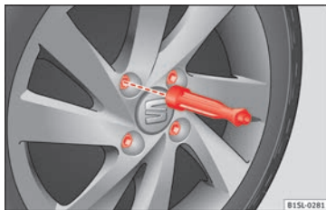
Fig. 57 Changing a wheel: loosen wheel bolts with the socket at the end of the wheel brace
