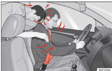
Fig. 71 The unbelted passenger in the rear seat is thrown forward violently, hitting the driver who is wearing a seat belt.
