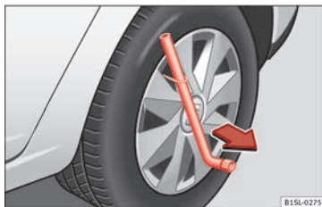
Fig. 51 Removing the full hubcap
