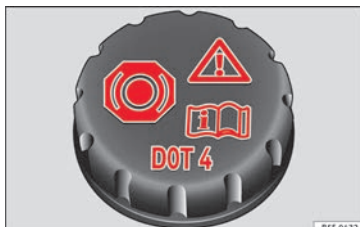
Fig. 43 Engine compartment: brake fluid reservoir cap.
