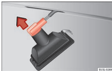
Fig. 91 Number plate light: Remove the bulb holder.
