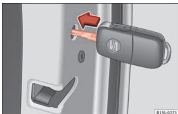
Fig. 5 Emergency locking of the vehicle using the vehicle key
