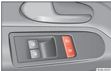
Fig. 103 In the driver door: central locking button
