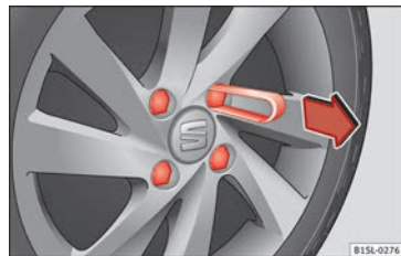
Fig. 52 Removing the wheel bolt caps
