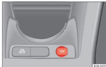
Fig. 133 Front centre console: 12 Volt socket in the storage compartment
