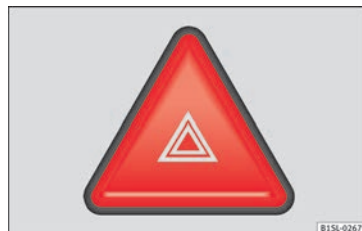
Fig. 31 Dash panel: switch for hazard warning lights.
