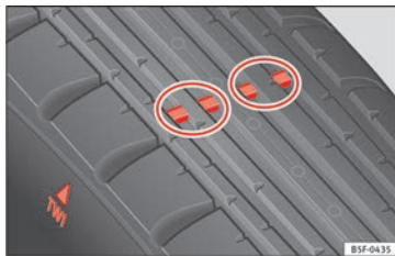
Fig. 175 Tyre tread: tread wear indicators
