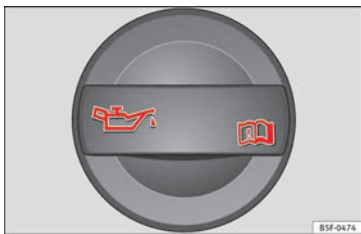
Fig. 41 In the engine compartment: Engine oil filler cap.
