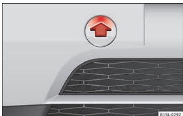
Fig. 80 On the right-hand side of the front bumper: Remove the cover.
