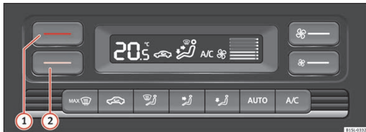
Fig. 37 At the top of the centre console: Climatronic controls
