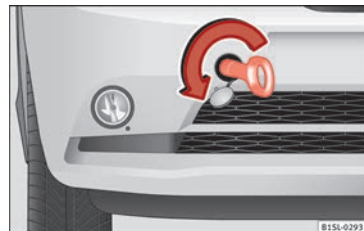
Fig. 58 Right side of the front bumper: towline anchorage screwed in.
