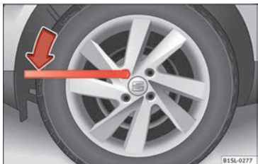
Fig. 53 Changing a wheel: Slacken the wheel bolts.
