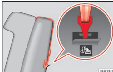
Fig. 27 Example of an upper retaining strap connected.
