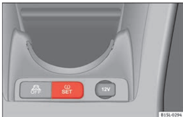
Fig. 176 Centre console: tyre monitor system button
