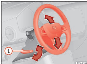
Fig. 17 Mechanical steering wheel adjustment
