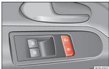
Fig. 2 In the driver door: central locking button
