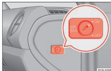
Fig. 20 On front passenger side: Key switch for enabling and disabling the front passenger front airbag.
