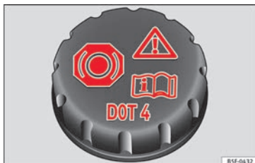
Fig. 62 Engine compartment: brake fluid reservoir cap.
