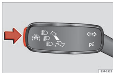
Fig. 44 On the turn signal and main beam headlight lever: button for the driver assistance systems
