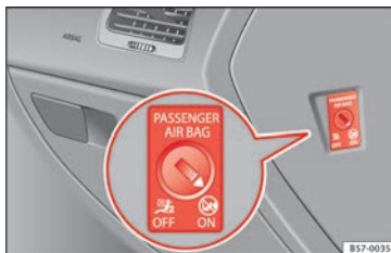
Fig. 94 Front passenger front airbag switch.
