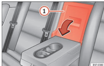
Fig. 158 On the rear seat backrest: opening the tailboard.
