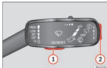
Fig. 42 Windscreen wiper lever: control buttons.
