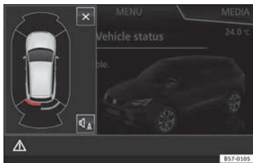
Fig. 220 Miniature indication of automatic activation.
