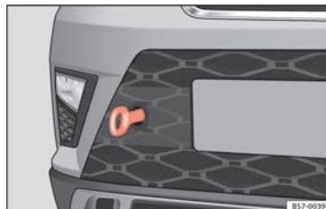
Fig. 98 Front bumper on right: towline anchorage screwed in.
