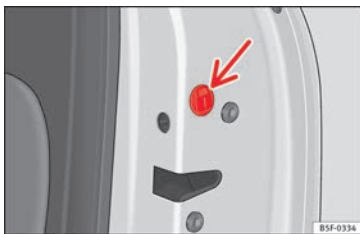
Fig. 4 Locking the door manually.
