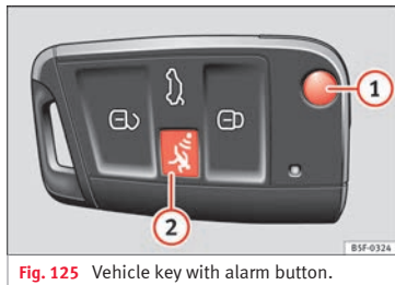
Fig. 125 Vehicle key with alarm button.
