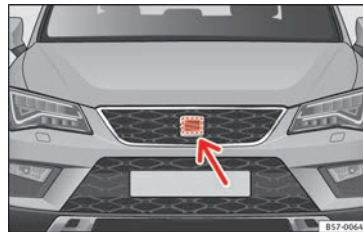
Fig. 185 On the front behind the SEAT badge: radar sensor.
