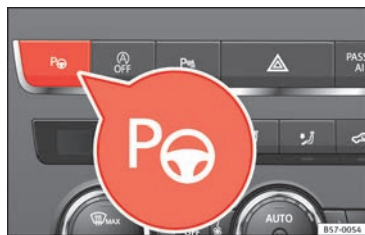
Fig. 212 At the top of the centre console: button to switch on the Park Assist system.
