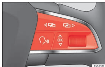
Fig. 43 Right side of multifunction steering wheel: control buttons.
