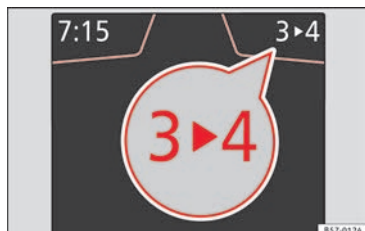
Fig. 46 Instrument panel: gear-change indicator (manual gearbox).
