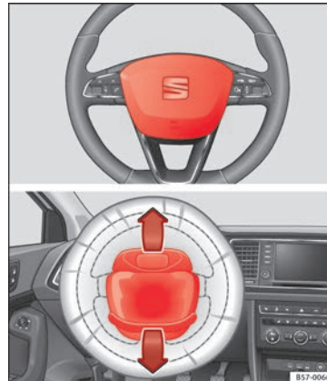
Fig. 20 Driver airbag located in steering wheel.
