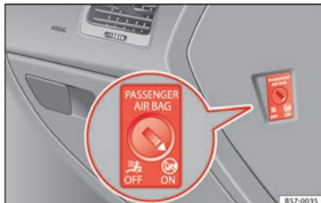
Fig. 22 Front passenger front airbag switch.
