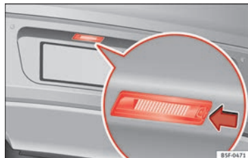
Fig. 114 In the rear bumper: number plate light.
