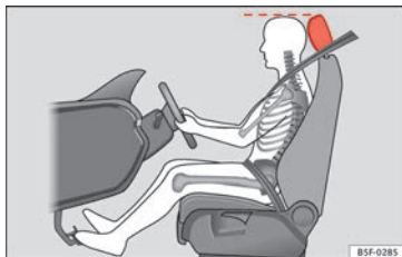
Fig. 83 Correct head restraint position for the driver.
