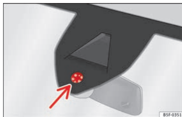
Fig. 144 Rain sensor sensitive surface
