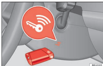
Fig. 171 On the right of the steering column: emergency start.
