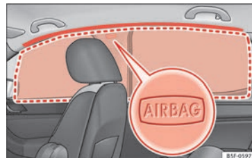
Fig. 27 Location of head-protection airbags.
