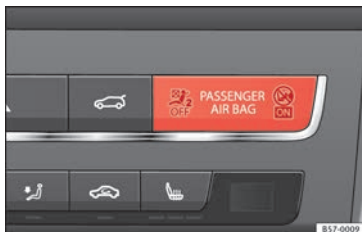
Fig. 93 Control lamp for disabling the front passenger front airbag on the dash panel
