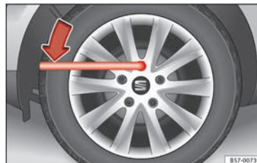
Fig. 72 Wheel: loosen the wheel bolts.
