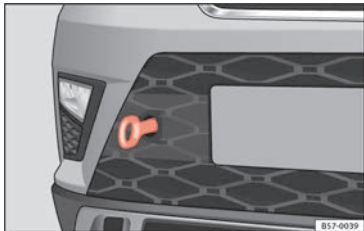
Fig. 75 Right side of the front bumper: towline anchorage screwed in.
