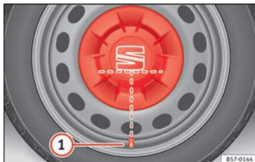
Fig. 69 Correct positioning of the central wheel trim for steel rims.
