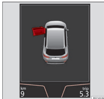
Fig. 50 On the instrument panel display: door open.
