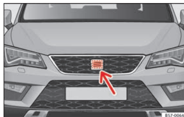
Fig. 193 On the front behind the SEAT badge: radar sensor.
