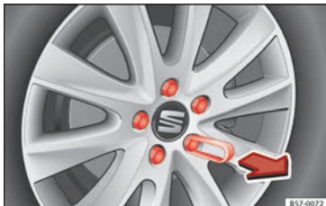
Fig. 70 Wheel: wheel bolts with caps.
