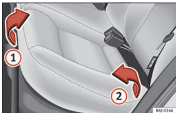
Fig. 153 Folding up the rear seat cushion.
