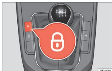
Fig. 3 Centre console: Central lock buttons.
