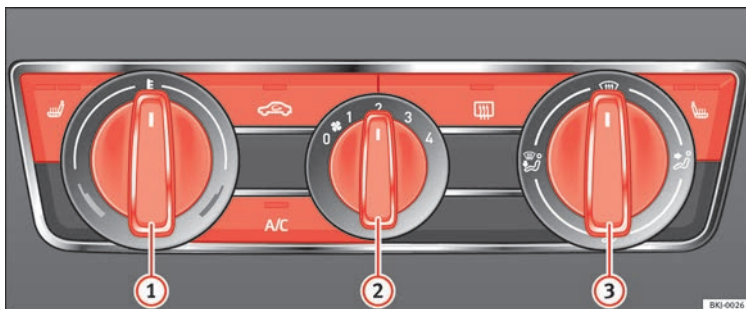
Fig. 61 In the centre console: Manual air conditioning controls.
