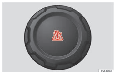
Fig. 66 Engine compartment: coolant expansion tank cap.
