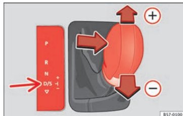
Fig. 179 Centre console: changing gear with tiptronic
