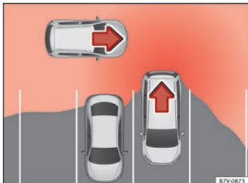
Fig. 205 Schematic representation of the rear cross traffic alert: zone monitored around the vehicle exiting the parking space.
