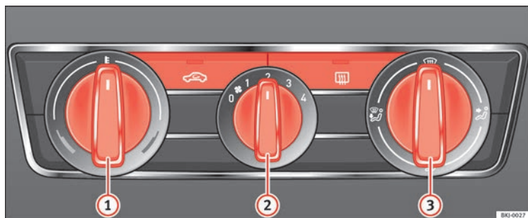
Fig. 62 In the centre console: heating system and fresh air controls.
