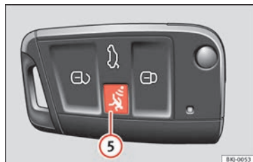
Fig. 134 Vehicle key with alarm button.
