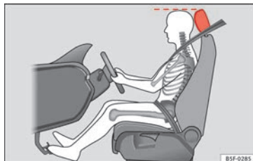
Fig. 92 Correct head restraint position for the driver.
