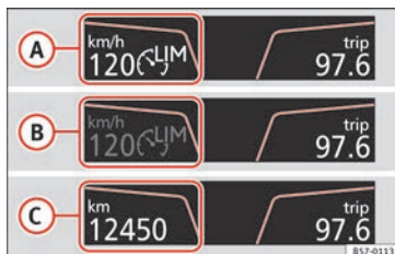
Fig. 184 On the instrument panel display: messages on the status of the speed limiter.
