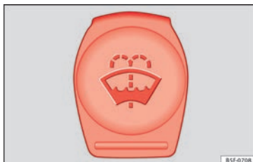
Fig. 68 In the engine compartment: windscreen washer reservoir top.
