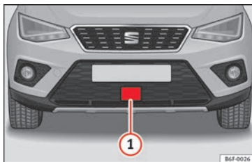
Fig. 195 On the front bumper: radar sensor.
