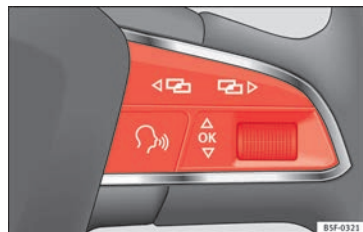
Fig. 45 Right side of multifunction steering wheel: control buttons.
