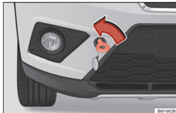
Fig. 84 Right side of the front bumper: Towing ring.
