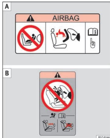
Fig. 28 Airbag stickers - version 2: on the passenger-side sun blind A and on the rear frame of the front passenger's door B .
