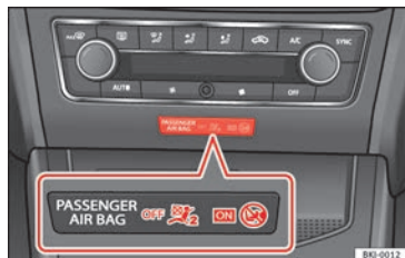
Fig. 103 Centre side of dash panel: control lamp for deactivated front passenger airbag in centre console.
