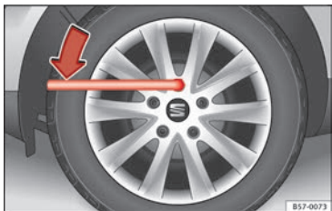
Fig. 80 Changing a wheel: loosen the wheel bolts.
