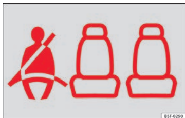
Fig. 96 Instrument panel: right rear seat occupied and corresponding seat belt fastened display.
