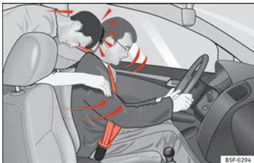
Fig. 99 The unbelted passenger in the rear seat is thrown forward violently, hitting the driver who is wearing a seat belt.
