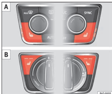
Fig. 152 In the centre console: front seats heating switch A : version with Climatronic. B : version with manual air conditioning.
