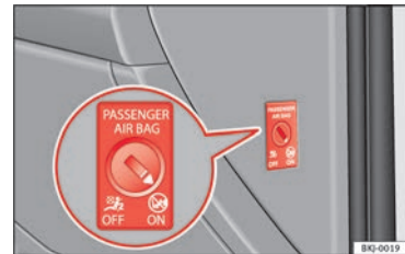
Fig. 22 Front passenger front airbag switch.
