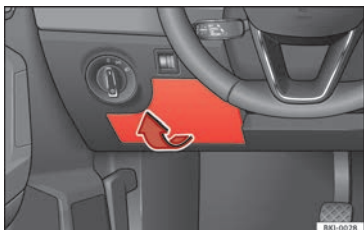
Fig. 69 On the driver-side dash panel: fuse box cover.
