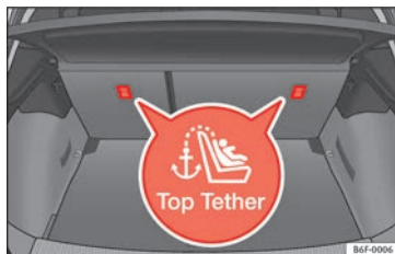
Fig. 31 Position of the Top Tether rings on the back of the rear seat.
