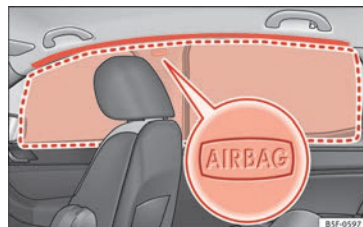
Fig. 25 Location and deployment area of the head-protection airbag.
