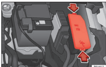
Fig. 70 In the engine compartment: fuse box cover.
