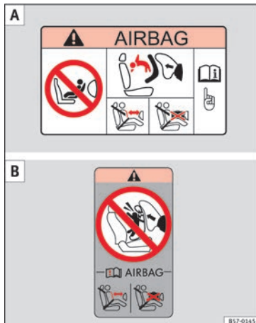
Fig. 27 Airbag stickers - version 1: on the passenger-side sun blind A and on the rear frame of the front passenger's door B .
