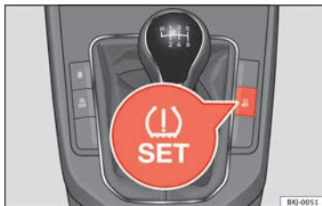
Fig. 241 Centre console: tyre monitoring system button.
