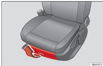
Fig. 156 Storage compartment under the right front passenger seat.
