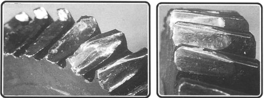
Figure 17. Completely ruined gear.
