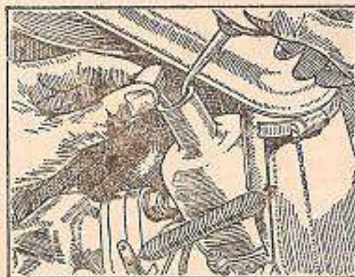
Fig. 53 Lubricating the carburettor piston damper
