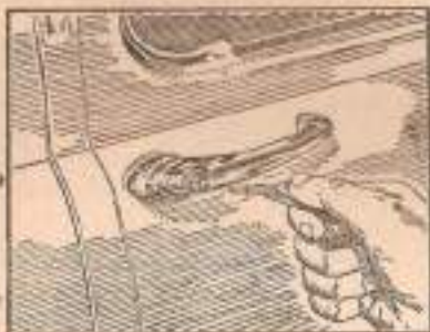
Fig. 6 The ignition key is used to lock the driver's door
