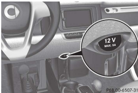
Auxiliary power outlet
