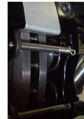
Correct R-Clip Fitting - Within the recess - R-Clip facing Outwards
