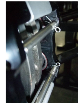
Correct R-Clip Fitting - Within the recess - R-Clip facing Inwards
