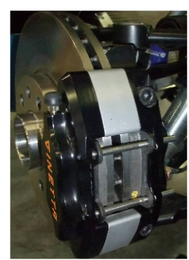
Correct Caliper Assembly
