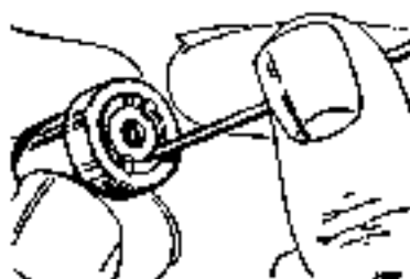
Fig. Da.30 Clearing the feed channel bores
