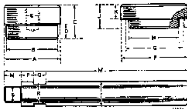
Fig. A.16 Cylinder liner pilot dimensions
