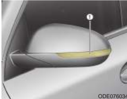
(1) Side repeater lamp (LED type)
