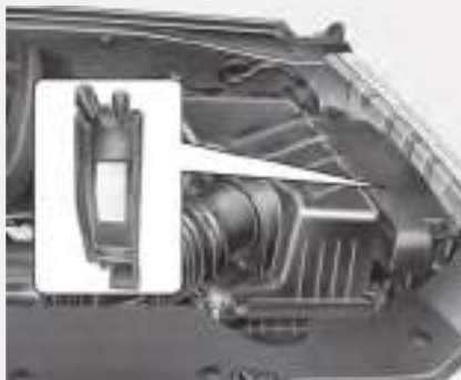
Engine compartment fuse panel
