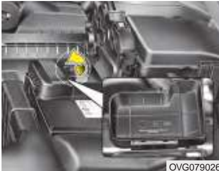
Engine room (Battery terminal cover)
