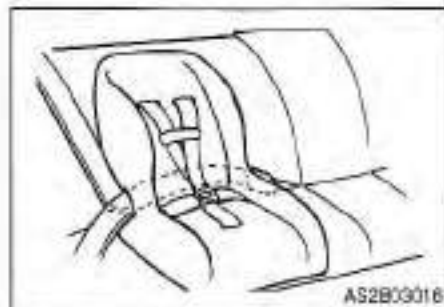
Installing a child restraint system in rear outboard seats
