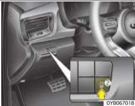
Low tire pressure telltale (1) / TPMS SET switch (2)
