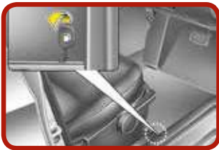
Opening the fuel filler [4] Pull up the fuel filler lid release lever.
