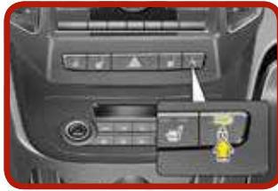
Operating door locks from inside the vehicle with central door lock switch [4]
