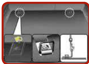
Securing with "Tether Anchor" system* [3]
