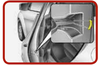
Emergency door locking [4]
