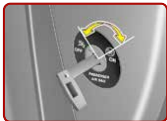
Passenger's front air bag ON/OFF switch [3]
