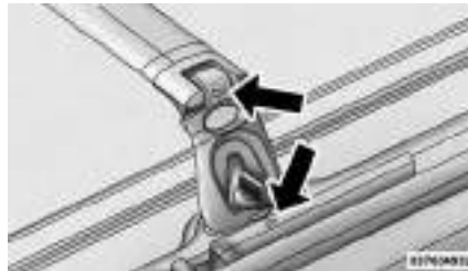
Crossbar To Side Rail Installation
