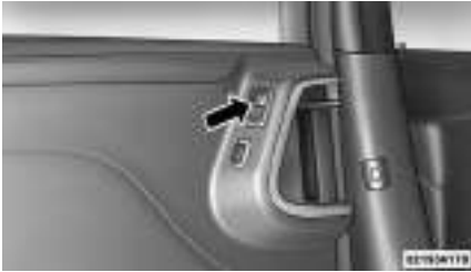
Sliding Door Power Window Switch
