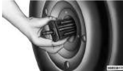
Removing Wheel Spacer
