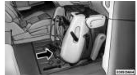
Cross Beam For Seat Removal
