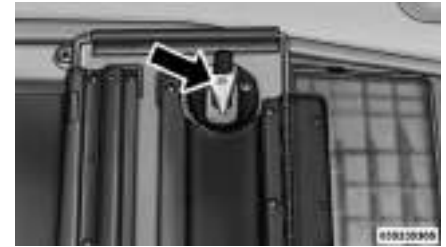
Storage Bin Cover Emergency Release Lever
