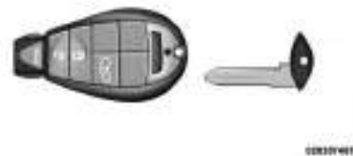
Ignition Node Module (IGNM) Emergency Key Removal
