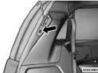
Rear Power Liftgate Switch
