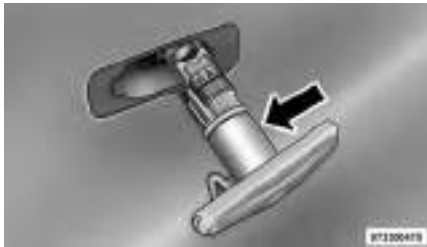
Side Repeater Bulb Replacement
