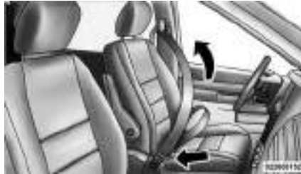
Removing Slack From Belt
