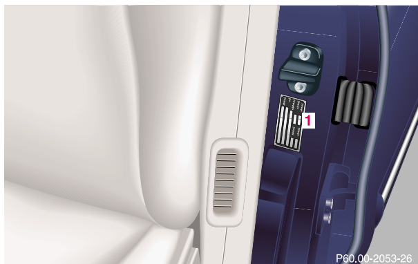
1 Certification label (below driver's door lock latch)
