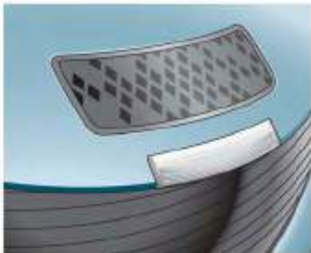
Solar cell module on the rear spoiler
