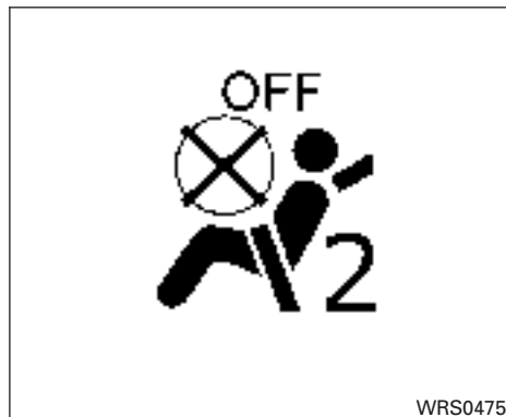
Front passenger air bag and status light
