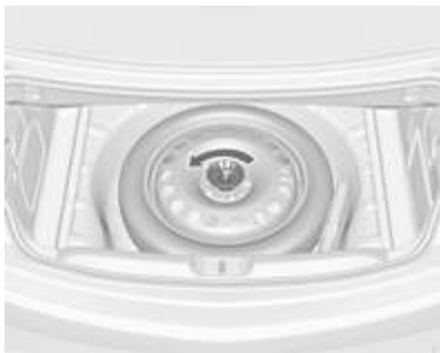
3. The spare wheel is secured with a wing nut in the well. Untwist nut,
