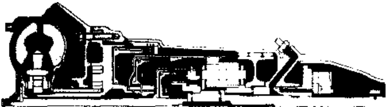
Figure 7C-23 Second Clutch Drum, Piston, Springs, Clutch Plates, Spacer And Ring Gear
