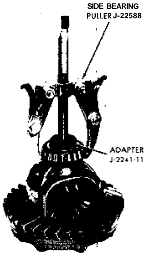
Figure 4B-6 Removing Differential Side Bearings
