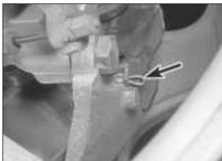
6.2 Brake pad locking key spring clip (arrowed)
