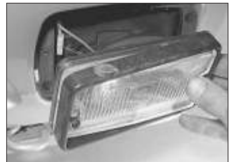
8.15 On GTI models, remove the driving light lens surround, lens and reflector ...
