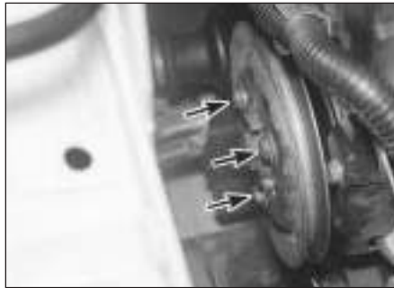
6.6a Undo the three bolts (arrowed) ...
