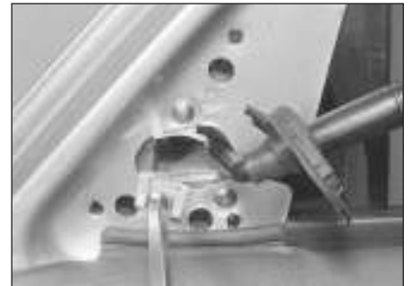
12.8 . . . remove the screws and withdraw the mirror
