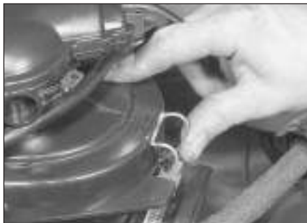
2.7a Release the spring clips . . .
