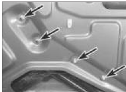
12.2a Window regulator mounting nuts (arrowed)
