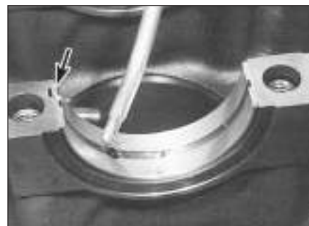
13.71 Ensure each bearing shell tab (arrowed) is correctly located and apply clean oil
