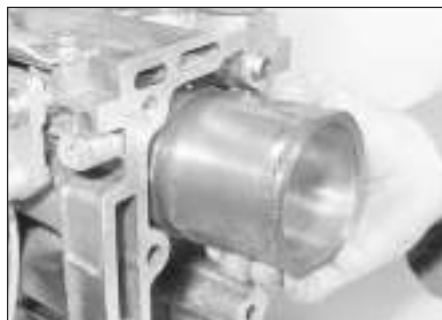
9.36 Fitting a liner to the cylinder block
