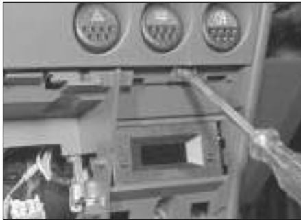
4.13a On later models, remove the switch panel lower screws . . .
