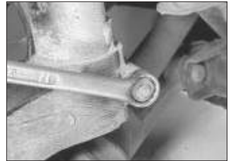
2.11 Unscrew the clamp bolt securing the lower end of the suspension strut to the hub carrier
