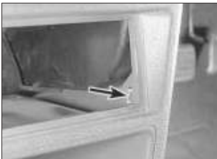
26.8 Centre console upper clip (arrowed)
