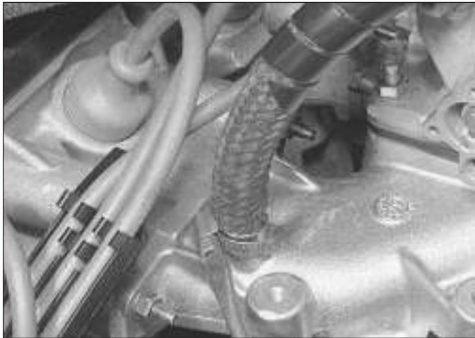
11.4 Disconnecting the brake servo vacuum hose at the inlet manifold - TU series engine shown
