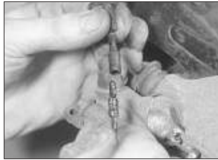
4.3b Disconnecting the pad wear wiring connector (DBA Bendix caliper)
