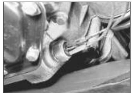
4.18 Reversing light switch location on the BH3 transmission
