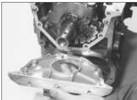
8.11 Removing the oil seal carrier from the front of the block - XU series engines
