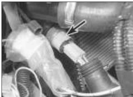
5.4a Disconnect the thermo-switch (arrowed) . . .
