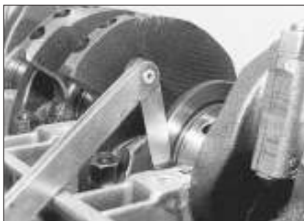
8.7 Checking crankshaft endfloat using feeler blades
