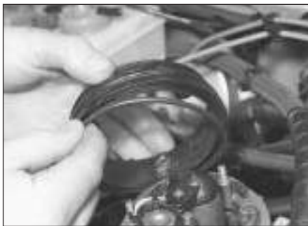
11.11b . . . and recover the O-ring
