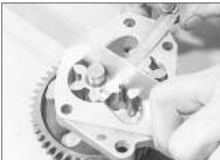
5.5 Checking oil pump gear endfloat
