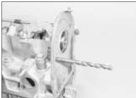
7.21 Align the camshaft sprocket cover plate using a dowel or twist drill
