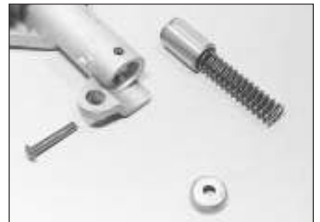
5.8 Oil pump pressure relief valve components
