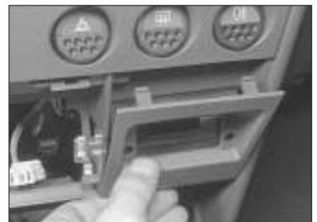
26.26 Removing the clock surround
