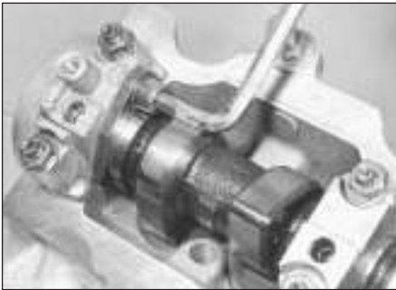
7.5a Removing the camshaft thrust plate bolt . . .
