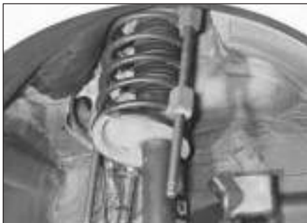
4.1 Coil spring compressors fitted to strut spring
