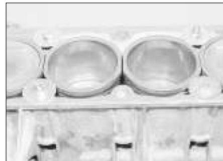
8.17 Cylinder liners clamped with washers and bolts
