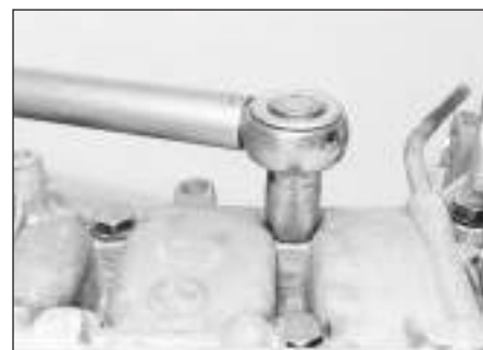
13.45 Tightening the main bearing/casing bolts
