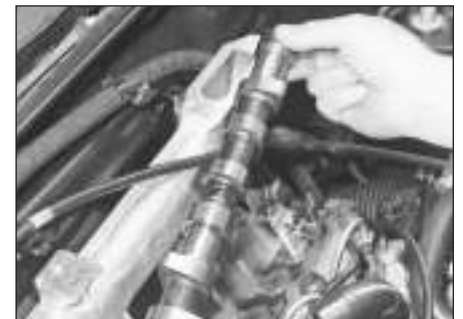
7.9 Lift the camshaft from the cylinder head
