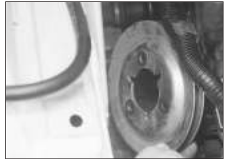
6.6b ... and remove the crankshaft pulley
