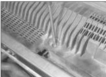
15.3 Removing the air intake grille screws
