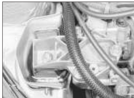
8.6 Right-hand engine mounting and cylinder head bracket
