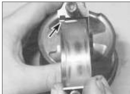
14.5 Ensure that the tab (arrowed) is correctly located in the connecting rod when fitting the bearing shells
