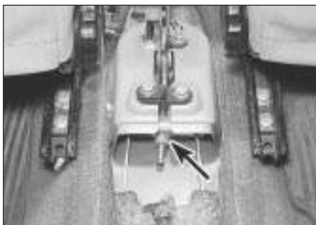
15.5 Handbrake adjustment nut and locknut (arrowed)
