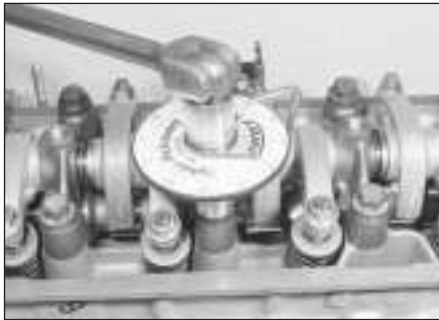
11.38 . . . then with an angle tightening gauge
