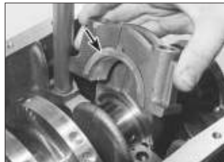
8.16 Removing the main bearing cap and thrustwashers (arrowed)
