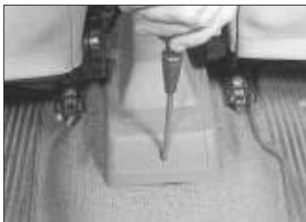
15.4 Remove the screw and lift the cover from the handbrake lever
