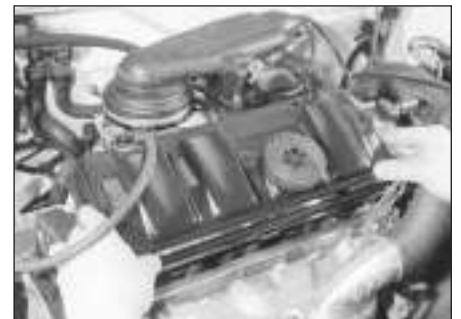
4.5 . . . and lift off the cylinder head cover
