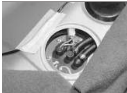
5.3 Fuel pump locations and connections
