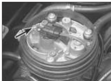
12.5 Fuel injector retaining plate securing screw (arrowed)
