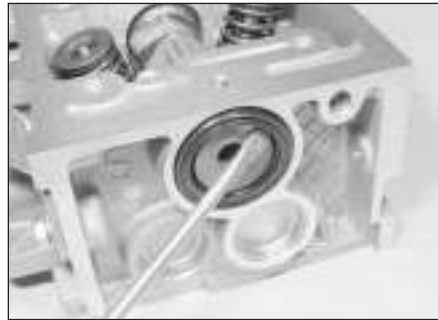
10.9a . . . prise out the oil seal . . .
