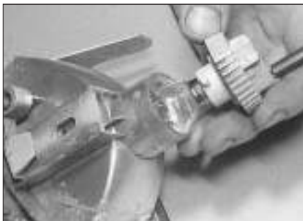
8.10 Remove the front direction indicator light bulbholder ...
