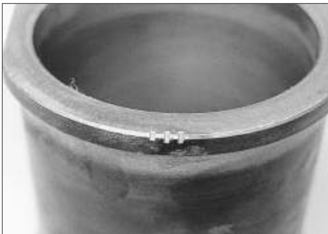
9.18 Cylinder liner size group marking
