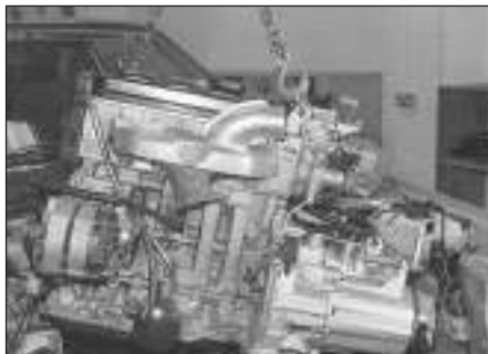
3.21 Removing the engine and manual transmission
