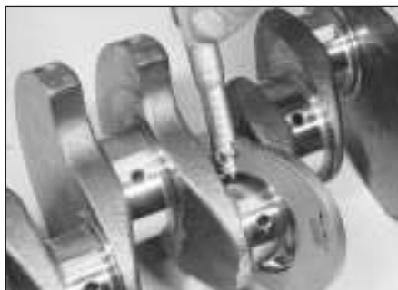
8.40 Measuring a crankshaft big-end journal diameter
