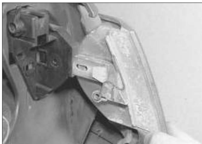
11.3b . . . and withdraw the front direction indicator light unit
