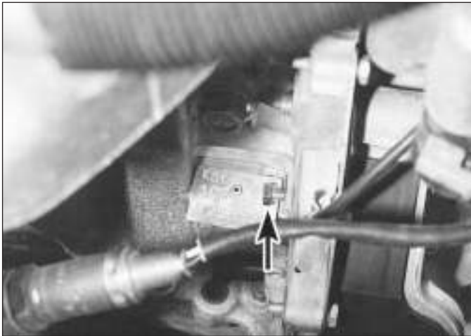
3.4 Insert a 6 mm bolt (arrowed) through hole in cylinder block flange and into timing hole in flywheel . . .
