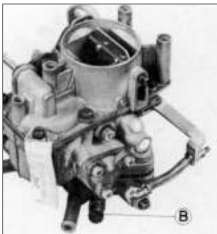
28.17a Typical idle mixture adjusting screw location (B) on the Solex PBISA carburettors
