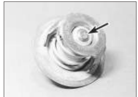
4.9 Thermostat temperature rating (arrowed) stamped on base
