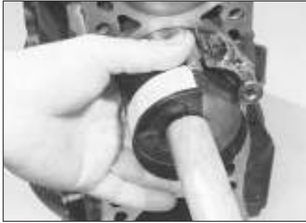
14.19 Tap the piston into the bore using a hammer handle
