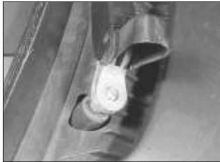
14.2b . . . and remove the wiper arm
