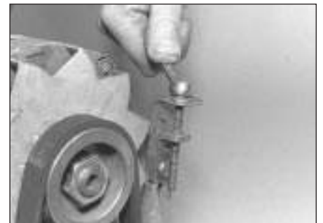
9.9 Slackening the alternator adjuster bolt to release the auxiliary drivebelt
