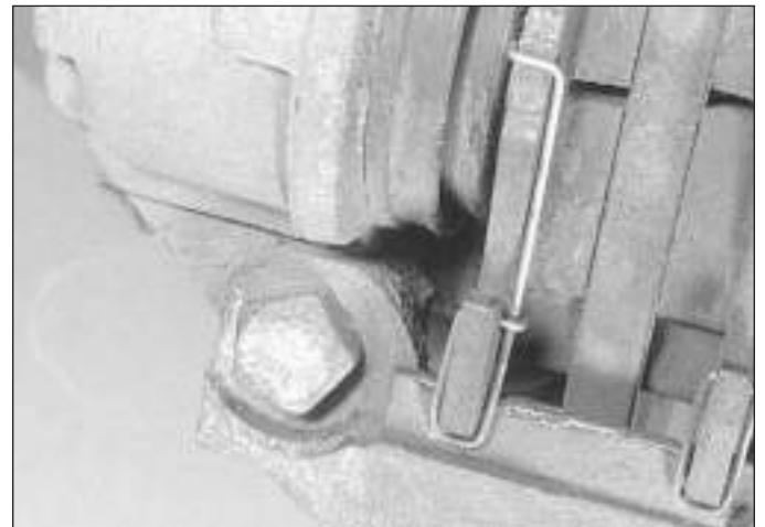
4.10 Fitted position of the anti-rattle springs on the brake pads (DBA Bendix caliper)
