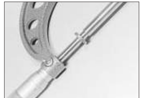
2.12b . . . then measure the shim thickness with a micrometer
