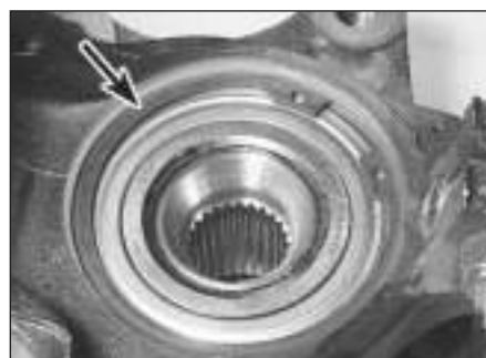
3.3 Front hub bearing retaining circlip (arrowed)
