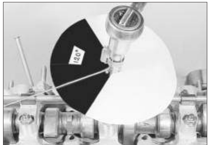
8.29 Home-made torque angle measuring gauge. Disc is fixed and pointer rotates
