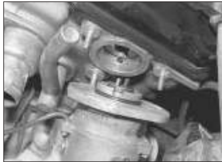
4.9b . . . and remove the distributor
