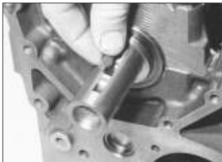
8.12b . . . and remove the Woodruff key
