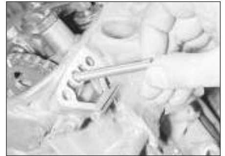
7.21 Removing the fuel pump plunger
