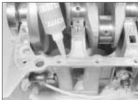
13.73 Apply a thin film of sealant to the cylinder block/crankcase mating face . . .
