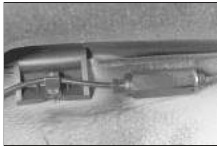
13.7 Rear brake compensator fitted to 1.9 GTI models
