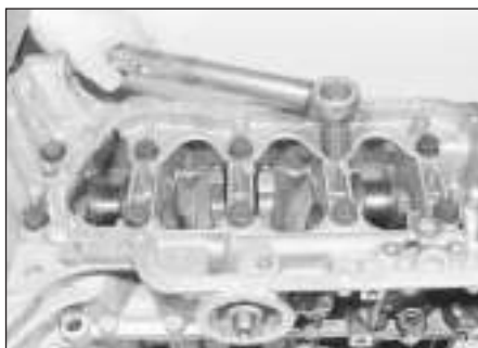
13.75a Tighten the 11 mm main bearing bolts to the Stage 1 torque setting . . .
