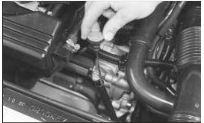
5.1 Withdrawing the automatic transmission fluid dipstick
