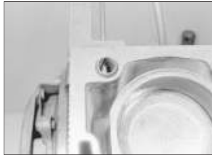
8.24 Using a nail to hold the cylinder block dowel in the raised position
