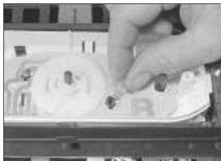
9.18 Removing the heater control panel illumination bulb on later models
