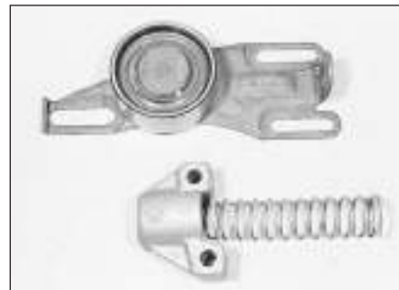
5.12 Spring loaded timing belt tensioner components
