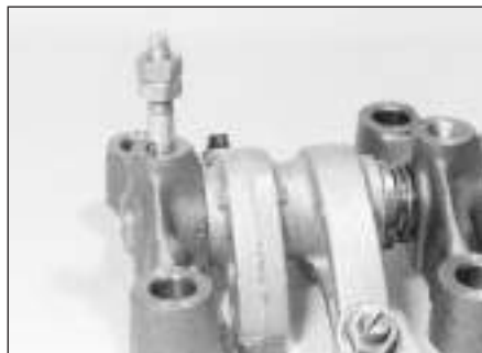
10.5a To remove the left-hand pedestal, lock two nuts together and unscrew the stud . . .
