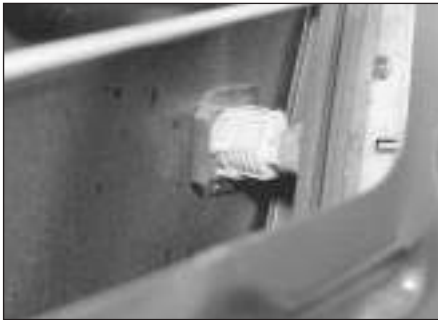
12.4 Pull out the retaining clip to remove the private lock
