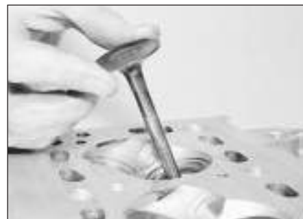
6.6 Withdraw the valve through the combustion chamber
