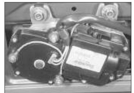
16.6 Tailgate wiper motor and mounting bolts
