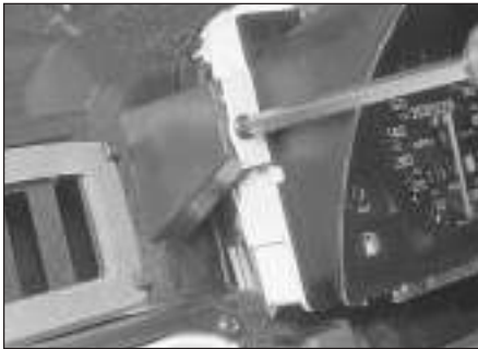
5.16 Removing the instrument panel mounting screws on later models . . .
