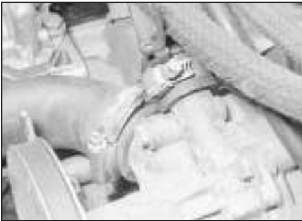
8.2 Radiator and heater hose connections on the coolant pump - XV, XW and XY series engines
