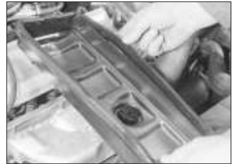
4.8 Ensure the rubber seal is correctly located on the cover when refitting
