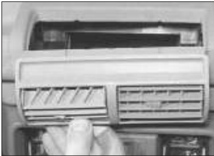
26.4 Removing the central air vents
