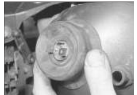
8.6 . . . remove the rubber cover . . .
