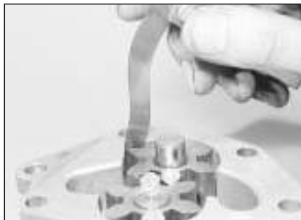
5.6 Checking oil pump gear to body clearance
