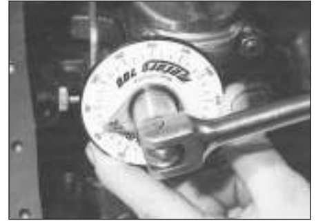
14.23 . . . and further, on XU series engines, through the specified angle using an angle tightening gauge
