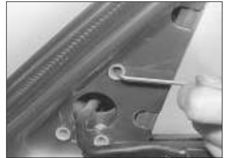
12.6b . . . and remove the exterior mirror mounting screws
