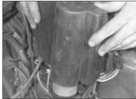
3.3 On all engines except TU series, access to the coil and ignition module is gained after sliding up the protective cover
