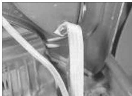
6.3 Braided lead fitted to the bonnet
