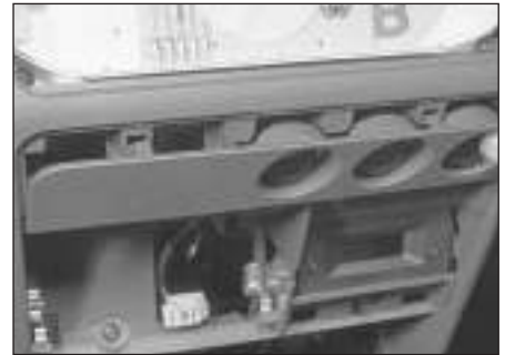
4.13c . . . and withdraw the switch panel surround
