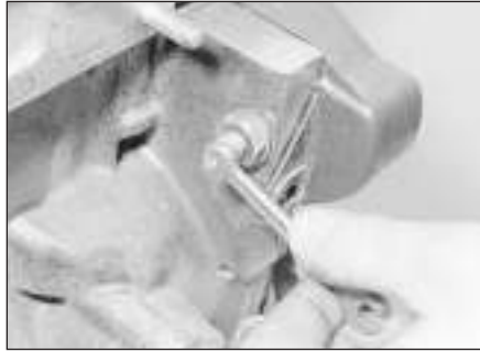
4.13b . . . and turn the tensioner cam spindle to the horizontal position
