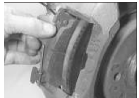
4.6 Removing the inner pad (DBA Bendix caliper)
