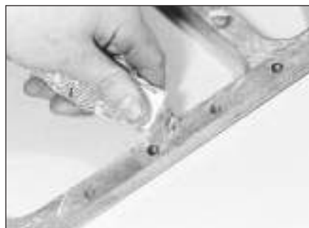
9.10 Applying sealant to the sump spacer plate upper surface
