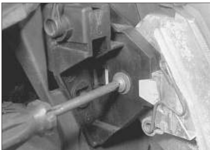
11.3a Remove the headlight adjustment assembly screw . . .
