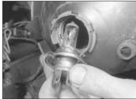
8.7b ... and withdraw the headlight bulb
