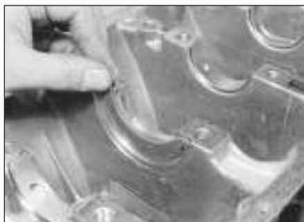
13.70 Refitting a crankshaft thrustwasher - TU series aluminium block engine
