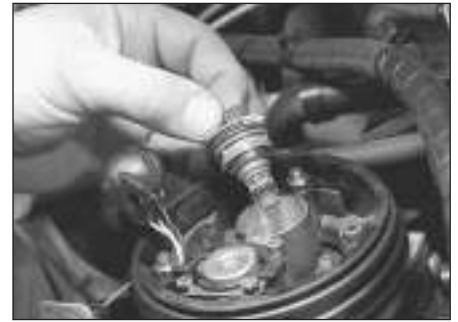
11.7 Withdrawing the fuel injector
