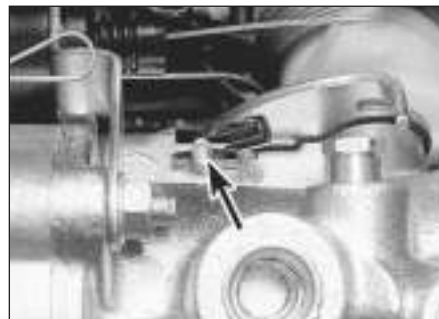
10.8 Prise the tamperproof cap from the throttle stop screw (arrowed) and adjust as described in text
