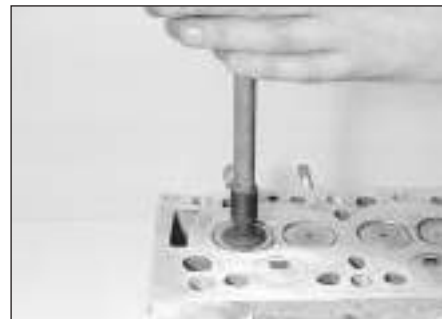
6.21 Grinding-in a valve
