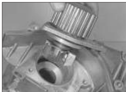
8.18a With the housing removed, undo the bolts and remove the coolant pump ...
