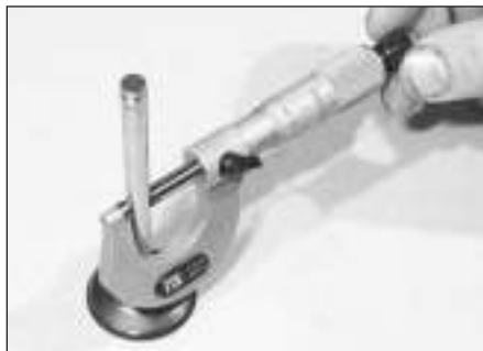
6.18 Measuring the valve stem diameter
