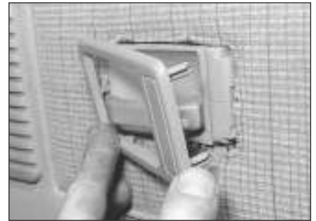
11.5 Removing the interior door handle surround
