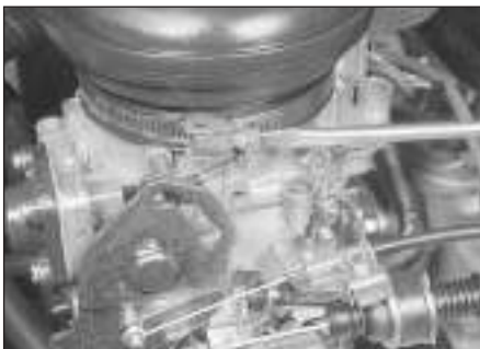
2.5 On TU series engines, slacken the air cleaner and release the ducting from the carburettor
