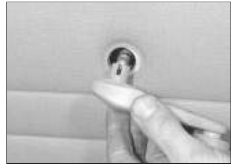
11.4 Removing the window regulator handle
