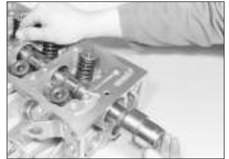
10.9b . . . and slide out the camshaft
