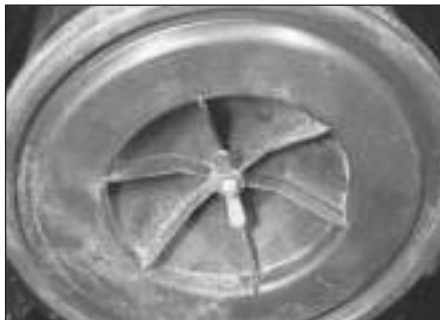
26.1 On XV, XW and XY series engines, unscrew the wing nut on the air cleaner cover . . .
