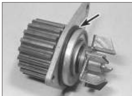
8.18b ... then recover the O-ring seal (arrowed)
