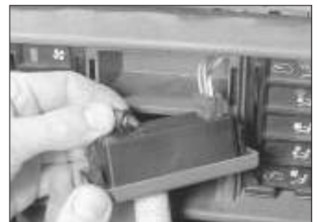
9.11 Removing digital clock illumination light bulb
