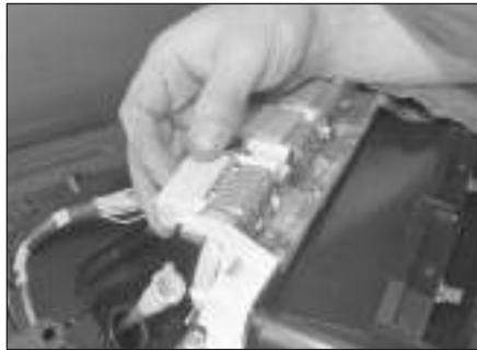
5.17 . . . and disconnecting the wiring plugs
