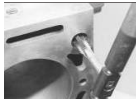
9.8 Cleaning a cylinder block threaded hole using a suitable tap
