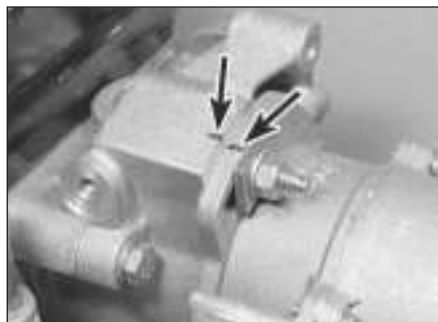
4.17 Mark the distributor and housing . . .
