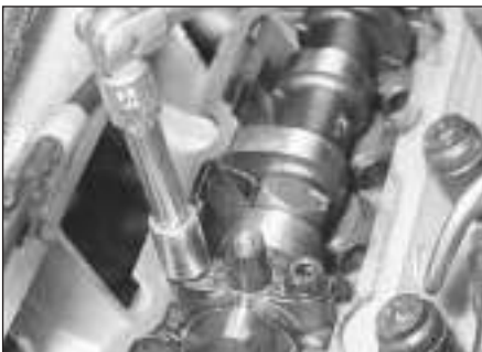
7.7 Progressively unscrew the camshaft bearing cap nuts . . .
