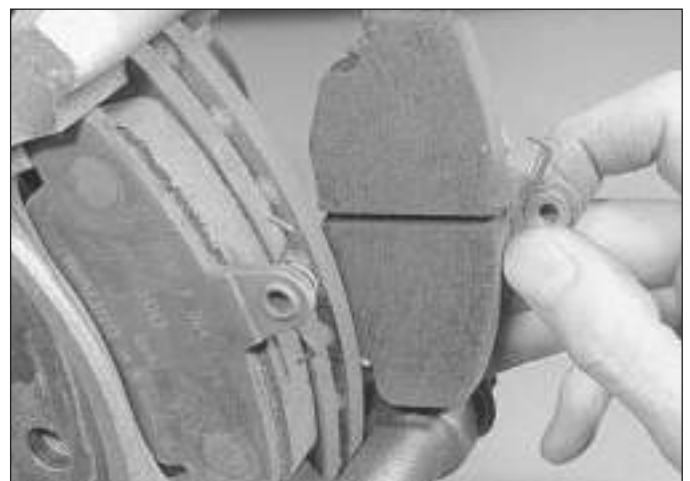
4.20b . . . then withdraw the two brake pads (1.9 GTI)
