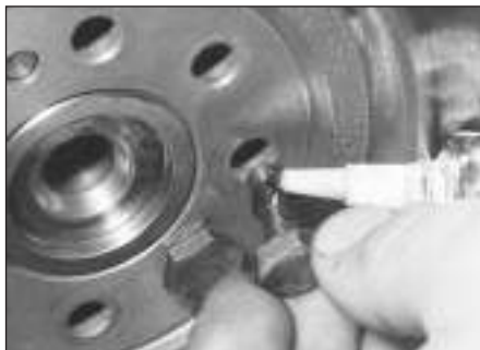
13.10 Apply thread locking compound to the flywheel bolts if not already pre-coated
