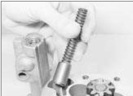
10.5b . . . and take out the relief valve piston and spring
