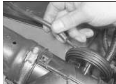
2.9 Disconnect the hose from the vacuum motor
