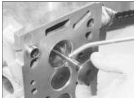
6.27 Lubricate the valve stems prior to refitting
