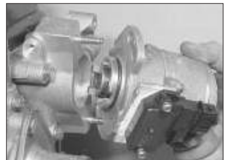
4.18 . . . then remove the distributor
