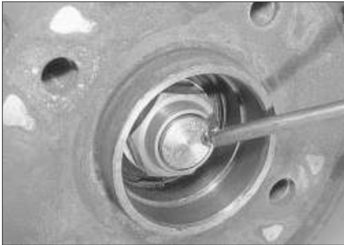
11.9 Lock the hub nut by staking the nut flange into the groove on the stub axle
