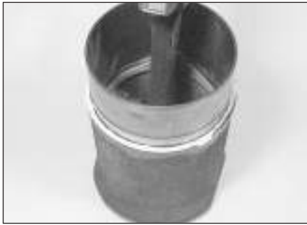
9.11 Cylinder liner with paper base seal
