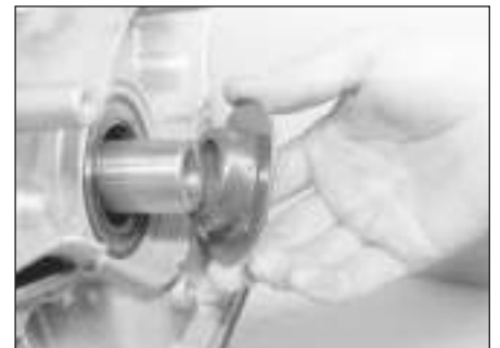
8.12 Remove the flanged spacer if necessary
