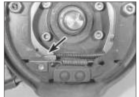
5.6 Automatic adjuster lever - arrowed (DBA Bendix type)
