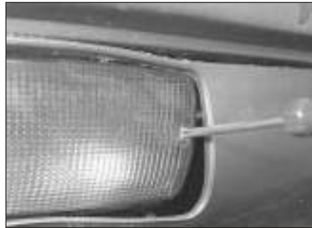
8.20 Remove the rear foglight lens . . .
