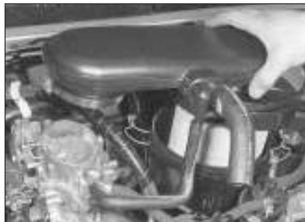
2.7b . . . and remove the air cleaner ducting and element from the body
