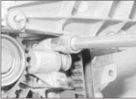
4.13a Slacken the two nuts at the front of the timing belt tensioner . . .
