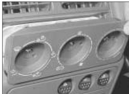
26.21 . . . Withdraw the heater control surround
