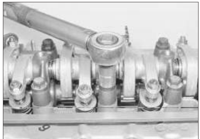
11.37b Working in the sequence, tighten the head bolts first with a torque wrench . . .
