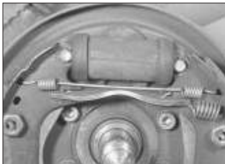
5.4 Upper return spring location (DBA Bendix type)
