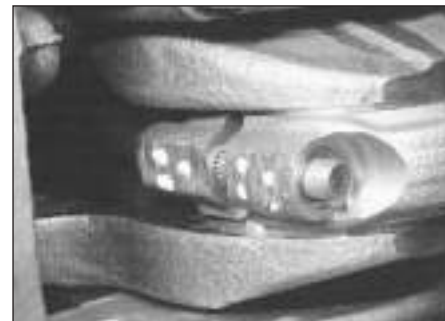
7.9 Marks made on connecting rod and bearing cap - XU and TU series engines
