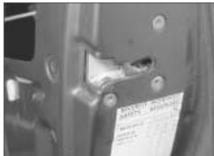
12.3a Door lock and mounting screws
