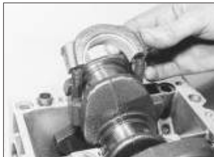
7.5 Remove the big-end bearing caps
