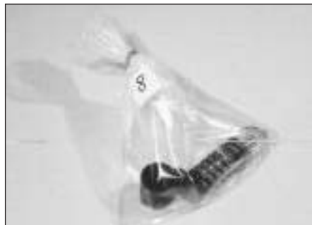
6.7 Place each valve and its associated components in a labelled polythene bag
