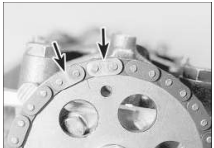
4.21 Camshaft sprocket timing mark positioned between two bright links (arrowed) on chain
