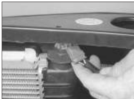
5.4b . . . and low coolant level sensor wiring
