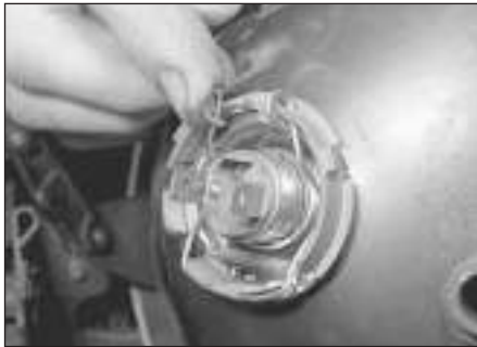
8.7a ... release the spring clips ...
