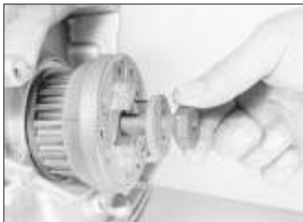
8.11a Remove the crankshaft sprocket bolt . . .
