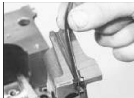
13.57 Fitting a sealing strip to No 1 main bearing cap
