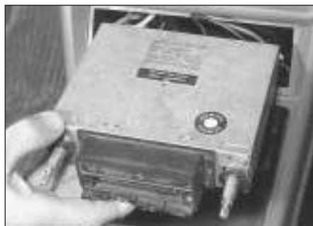
22.3 Removing the radio on early models
