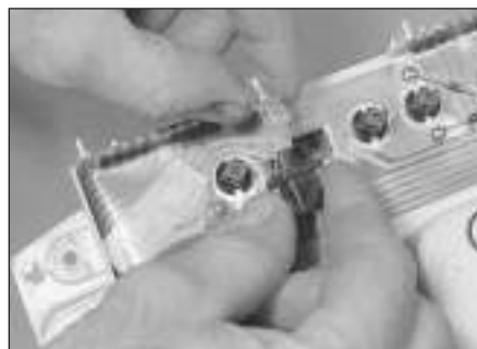
9.7 Removing square type instrument panel bulbholder
