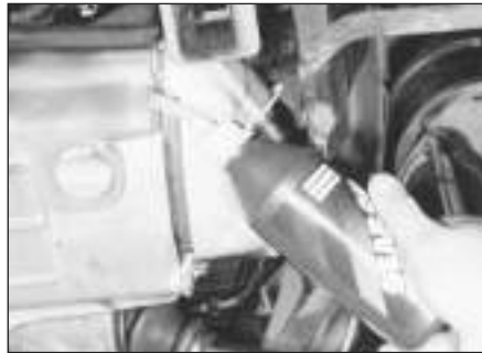
21.4 Topping-up the transmission oil level
