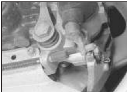
8.4 Handbrake cable attachment at rear brake caliper
