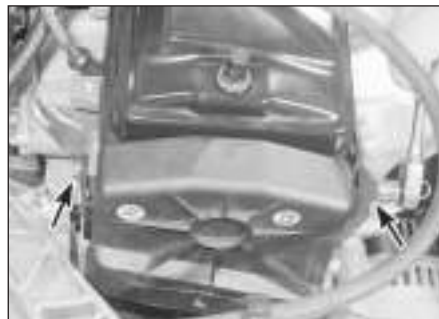
6.1a Undo the two retaining bolts (arrowed) . . .
