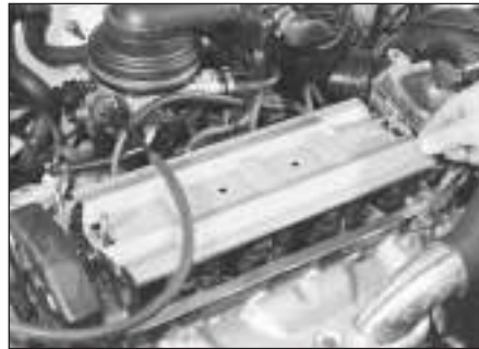
4.6b . . . and remove the oil baffle plate
