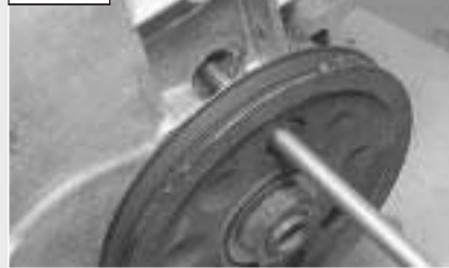
A crankshaft locking tool can be made from a 100 mm length of 8.0 mm dowel rod.
