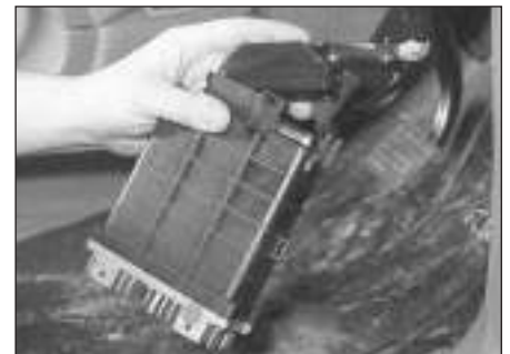
11.33 Disconnecting the ECU wiring plug
