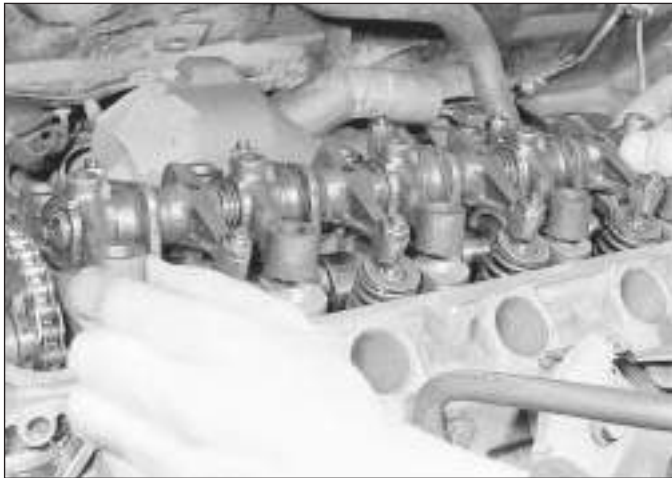
7.26 Removing the rocker shaft assembly
