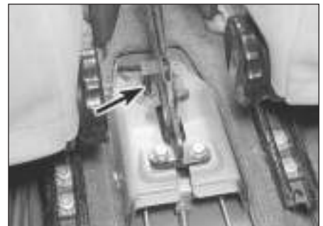
4.31 Handbrake warning light switch (arrowed)
