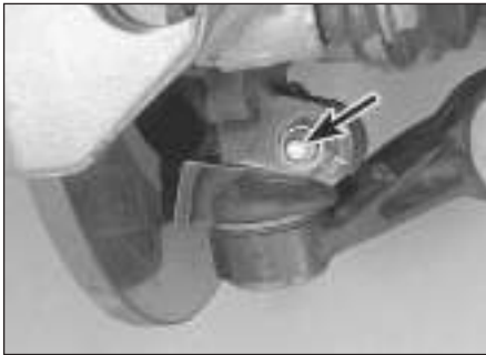
2.4a Unscrew the lower balljoint clamp bolt . . .
